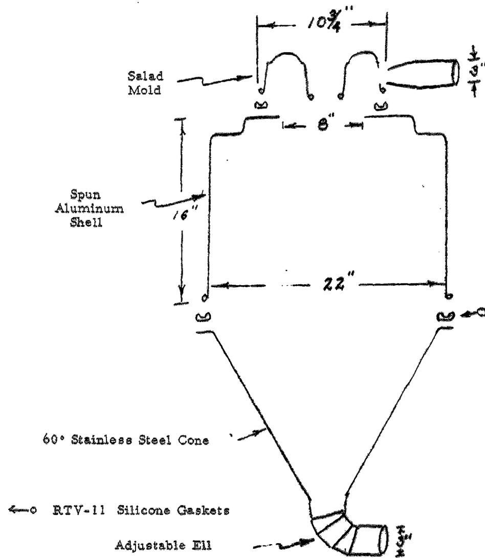
Figure 7. Exploded Cross Section of Drying Chamber.
