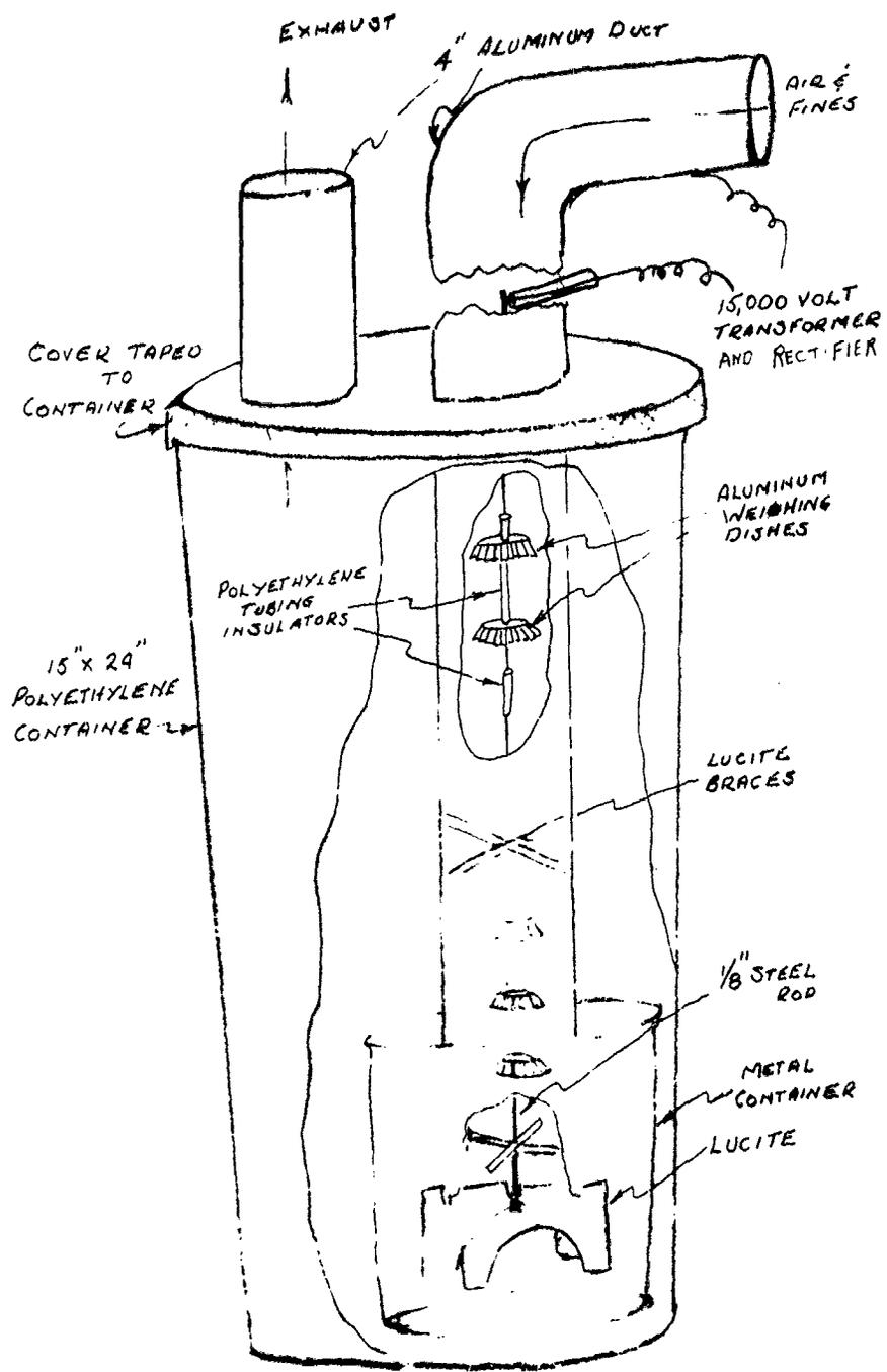
Figure 17. Electrostatic Precipitator.
