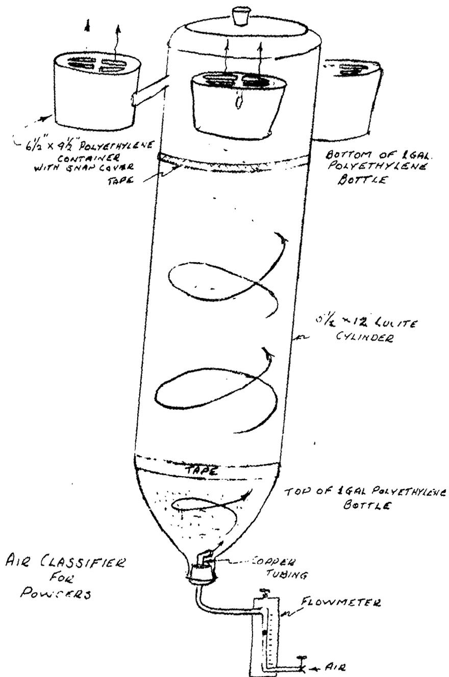
Figure 29. Air Classifier Apparatus for Separation of Powders.
