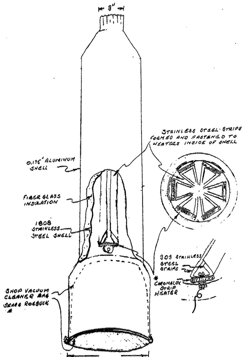
Figure 4. Stainless Steel Heater Shell.
