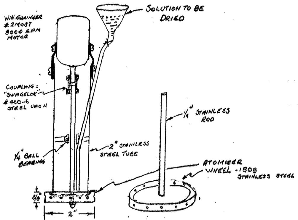
Figure 9. Centrifugal or Spinning Disc Type Atomizer.
