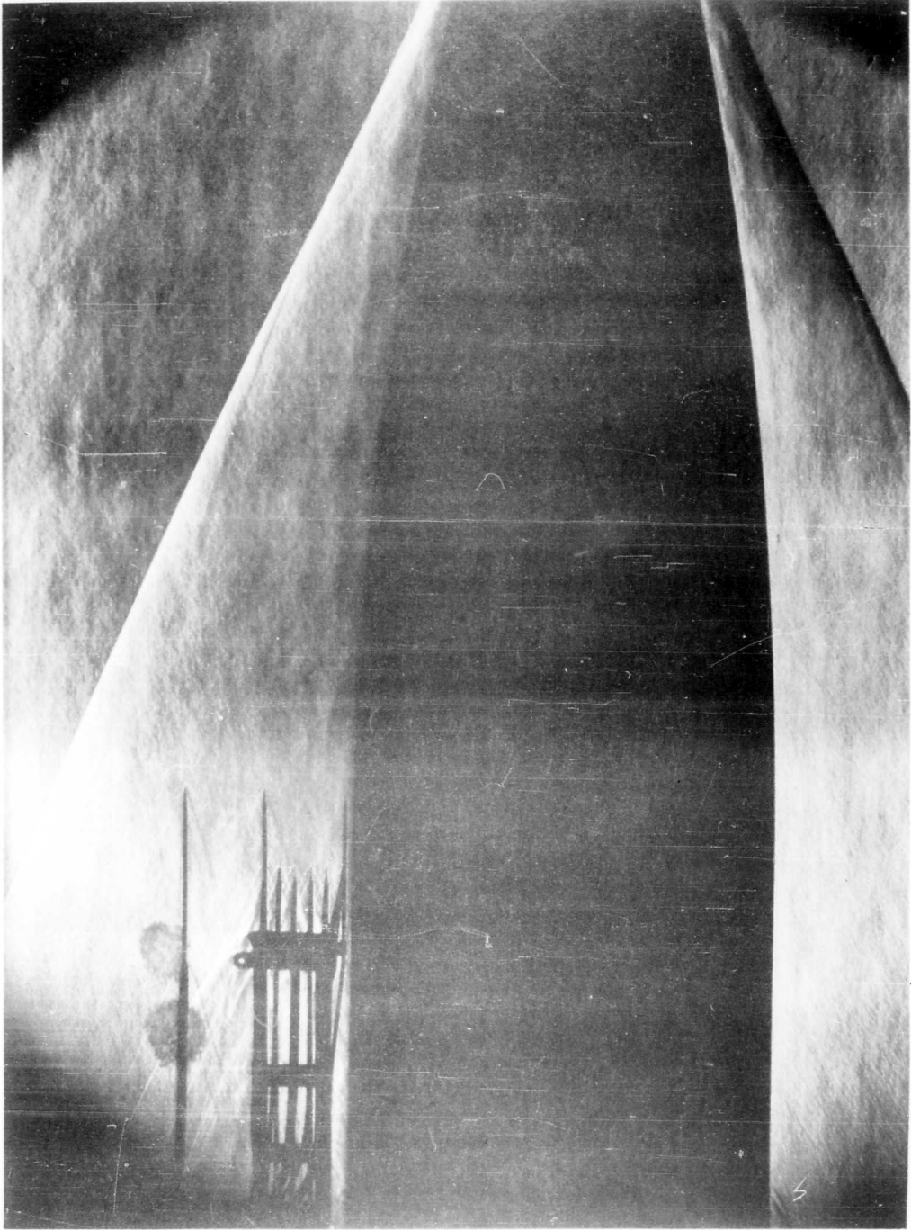
Figure 33. - Schlieren photograph of flow over convex center section at M_\infty = 3.3 . Static-pressure probes attached to rake to obtain profile at station 12.
