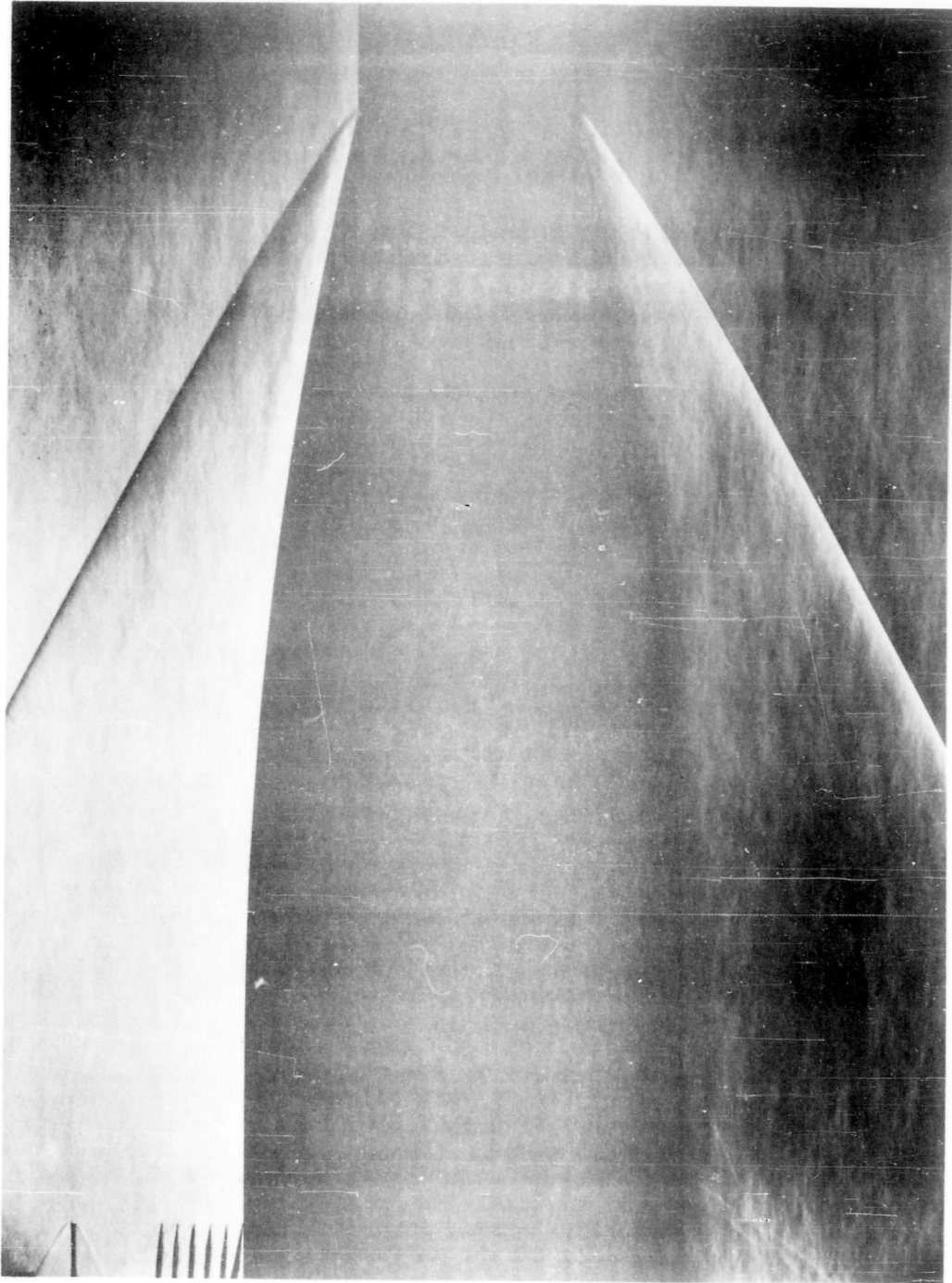
Figure 32. - Schlieren photograph of flow over convex center section at M_\infty = 2.58 . Rake mounted at station 14.
