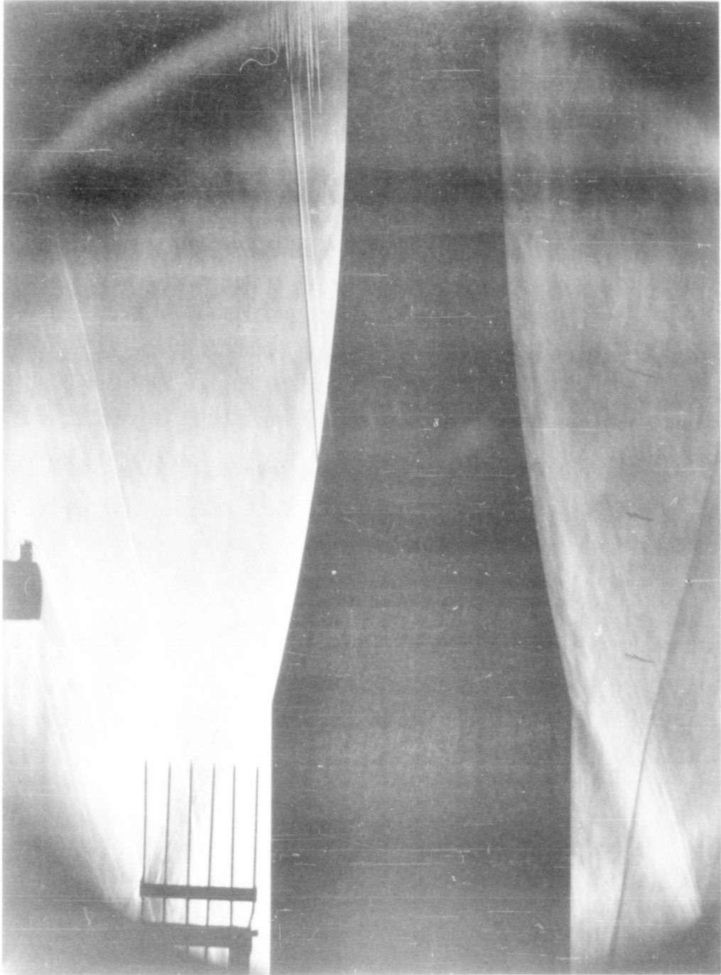
Figure 29. - Schlieren photograph of flow over concave center section at M_\infty = 4.5 . Static-pressure rake mounted at station 13.
