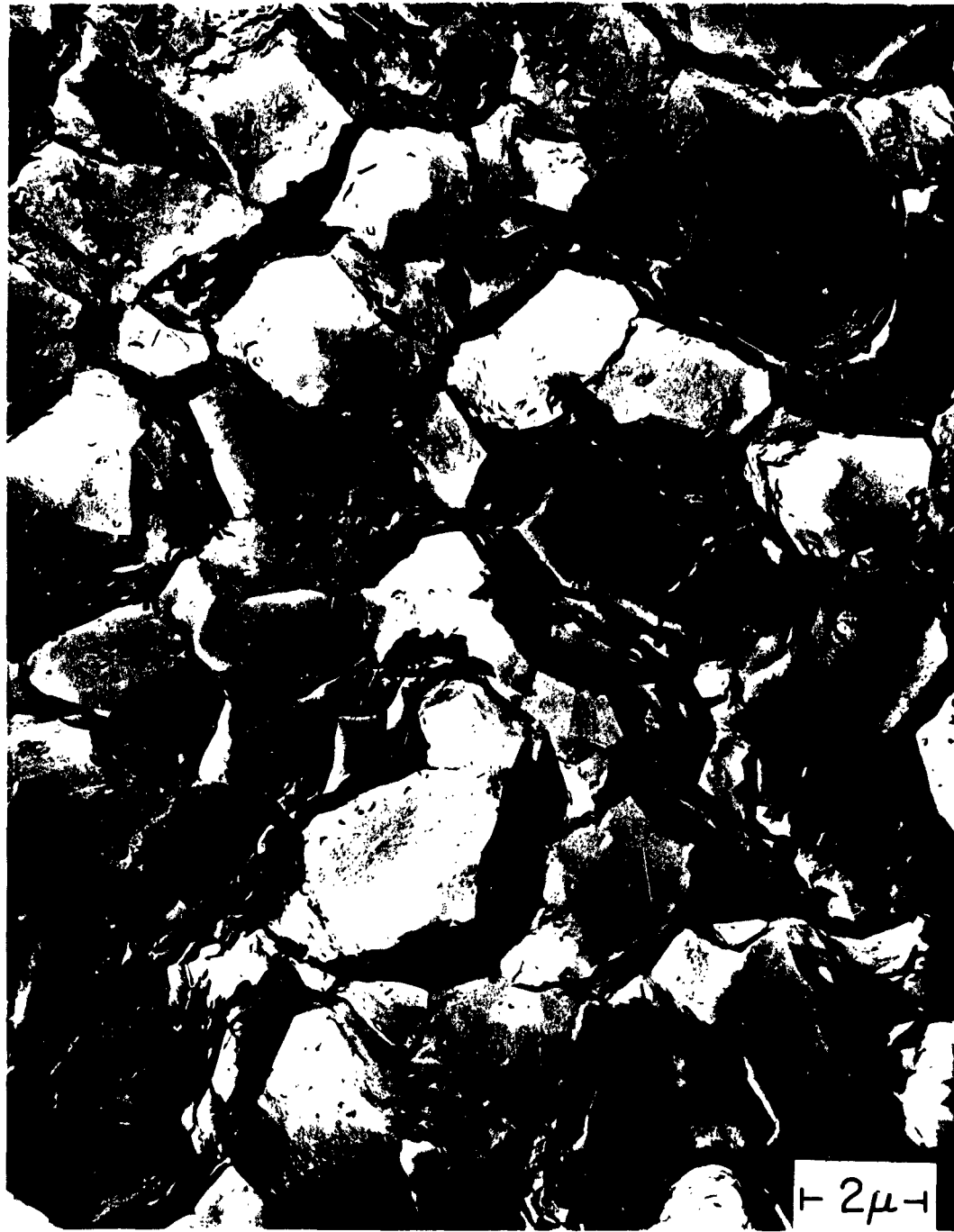
FIGURE 7. INTERGRANULAR FRACTURE IN THE CRACK-INITIATION REGION OF A 7075-T6 ALUMINUM ALLOY FORGING WHICH FAILED IN A FATIGUE TEST.(10)
