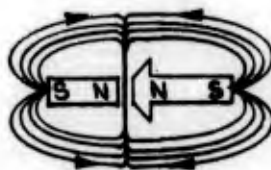
FIGURE 5-2 MAGNETIC CIRCUIT AND FLUX PATTERNS FOR ORIGINAL DISPLAY MODEL (FIG. 5.1)
