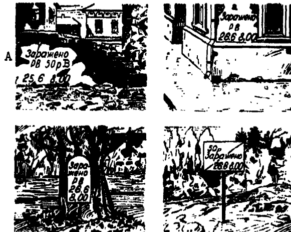
Fig. 17. The boundaries of contaminated areas can be indicated in the above fashion if no warning signs are available. A) Contaminated with radioactive substances; B) r.
