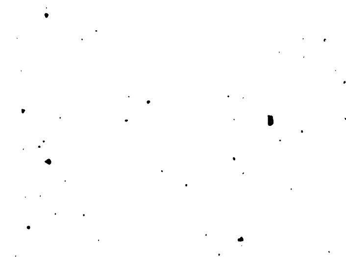
Figure 15. Inclusion Distribution Found in the Maraged 120 inch Vessel Closure Plate Ring Forging at the Delamination Site Unetched 100X
