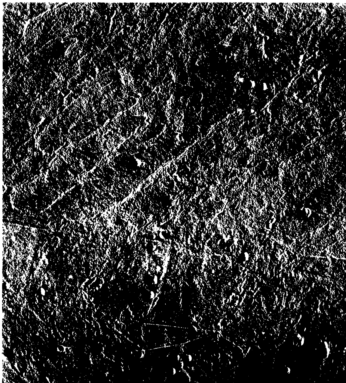
Figure 46. Typical Electron Microstructure of Ring Forging Used in 120 inch Maraging 18Ni Steel Vessel Closure Plate 13,000X Plastic Replica
