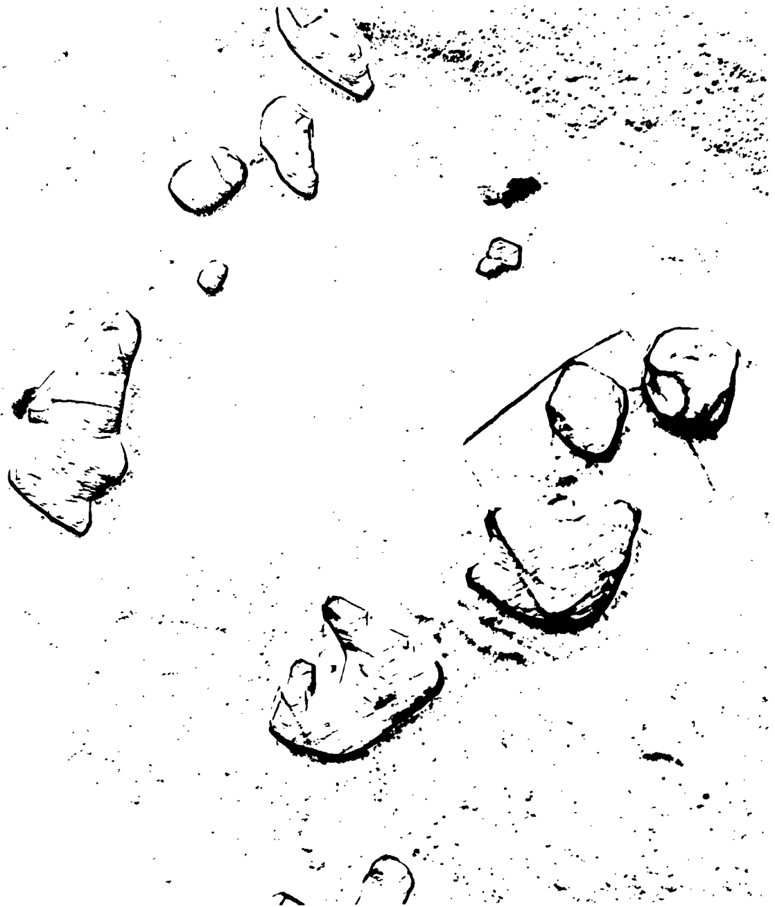
Figure 45. Typical Electron Microstructure Showing Clam Shell Shaped Titanium Carbides or Nitrides at Forging-Weld Fusion Zone. 120 inch Maraging 18Ni Steel Vessel Closure Plate 24,000X Plastic Replica
