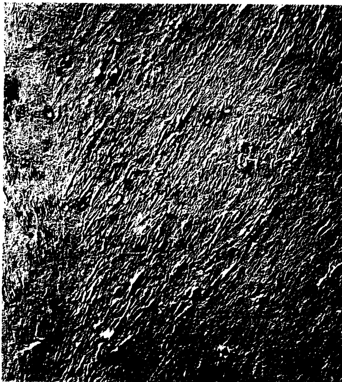
Figure 44. Electron Microstructure of Dark Etching Area of the Weld-Plate Interface. 120 inch Vessel Closure Plate Weld 6,900X Plastic Replica
