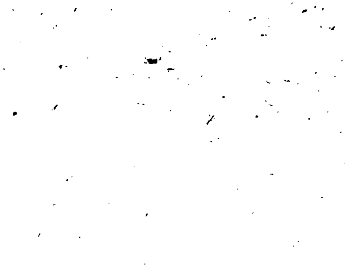
Figure 14. Inclusion Distribution in the Unaged Material of 120 inch Vessel Closure Plate Ring Forging
