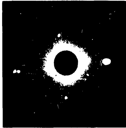
a) X-Ray of Electrolytically Cut End Specimen S1<110>3
