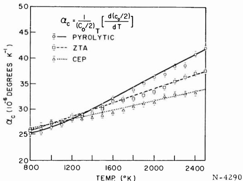
Figure 9. Linear Coefficient of Thermal Expansion of Graphites
