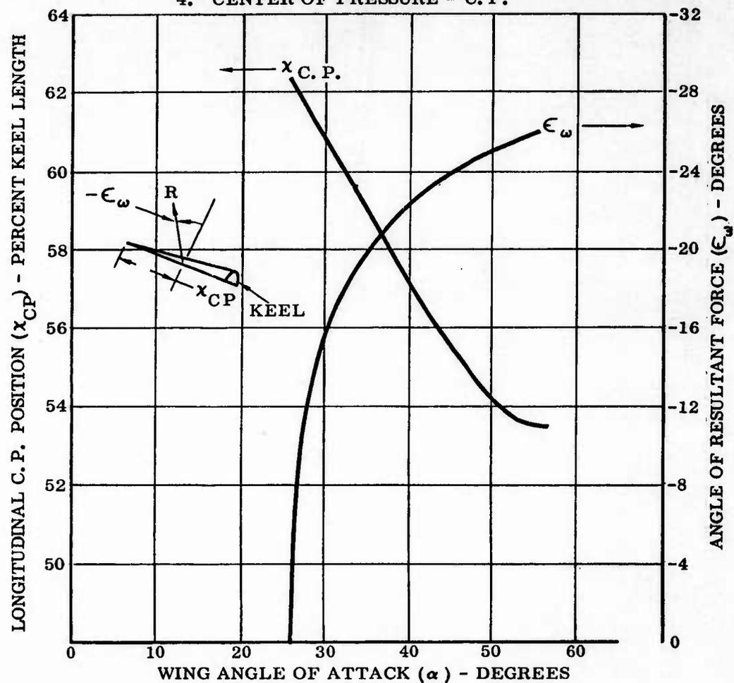
Figure 6 Theoretical Longitudinal C. P. Position
