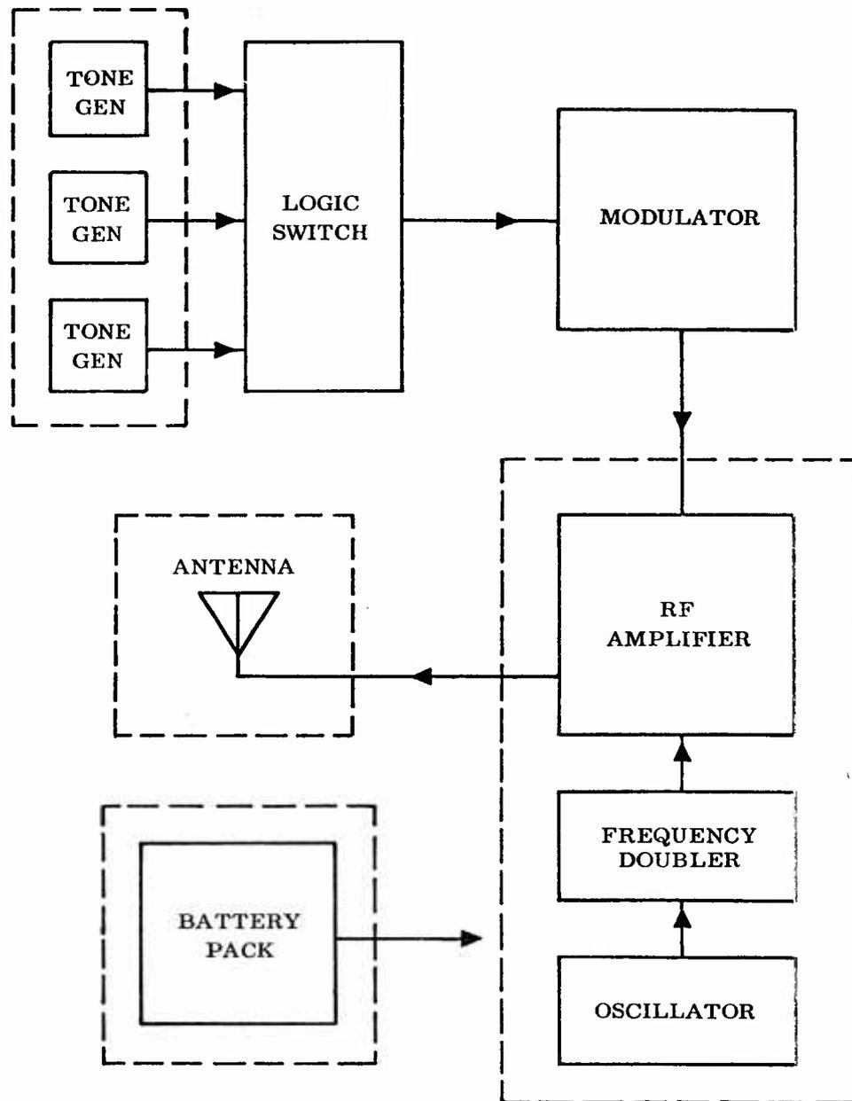
Figure 17 Control Transmitter, Block Diagram
