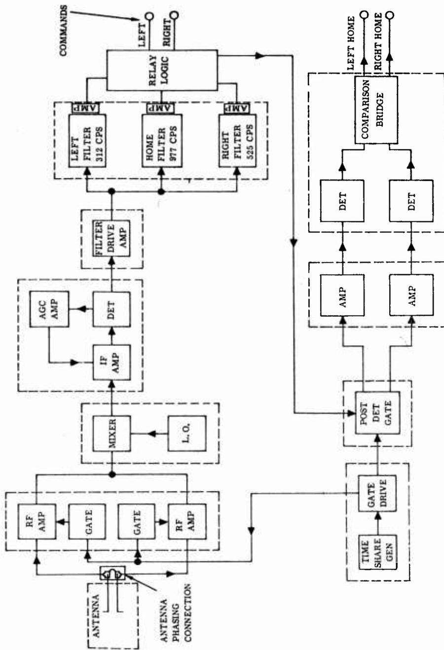
Figure 16 Control Receiver, Block Diagram
