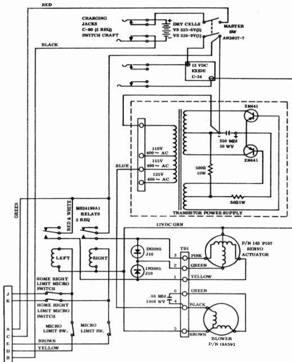
Figure 21 Paraglider Control Box, Schematic Diagram
