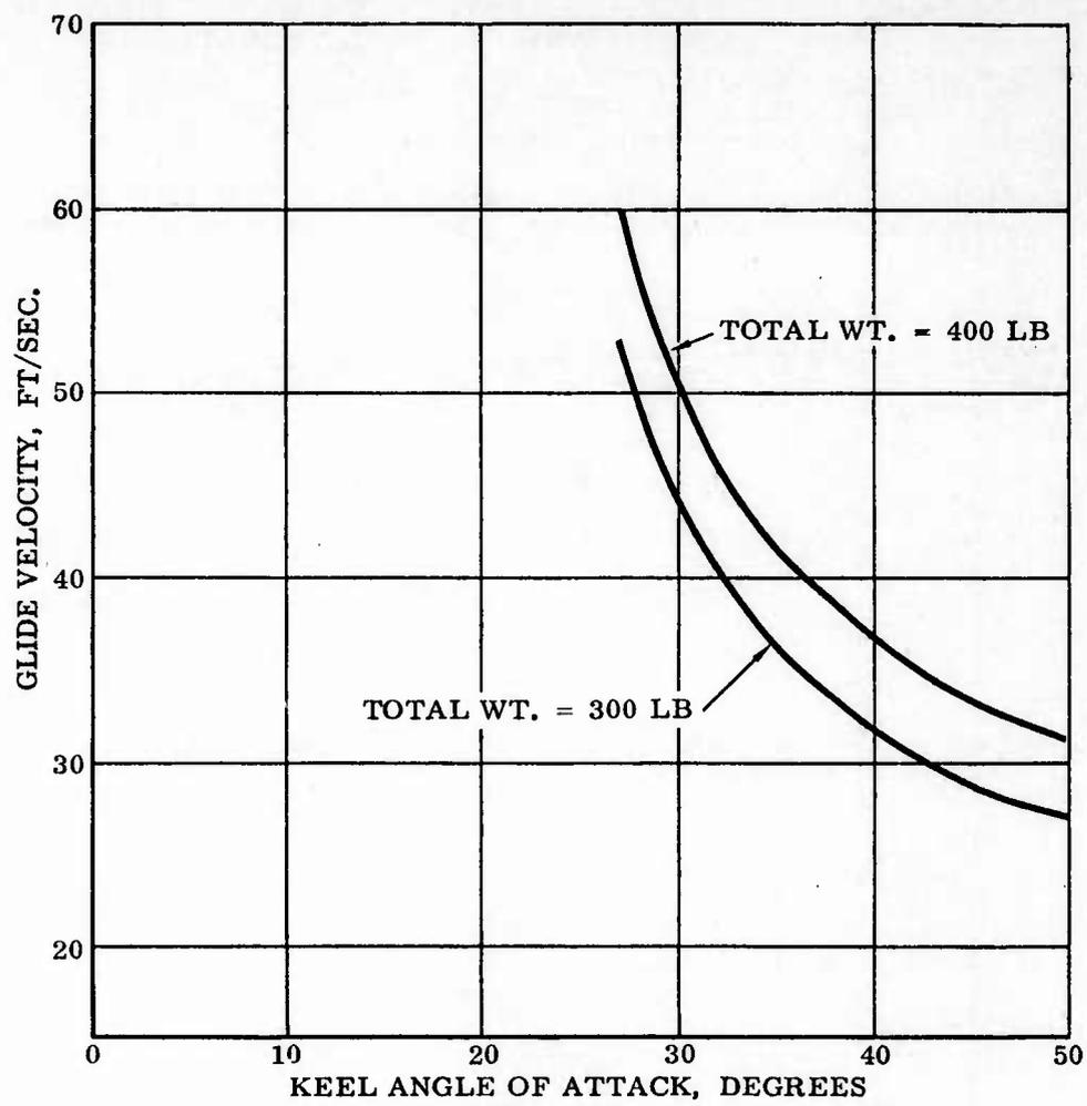
Figure 8 Predicted Glide Velocity at Sea Level
