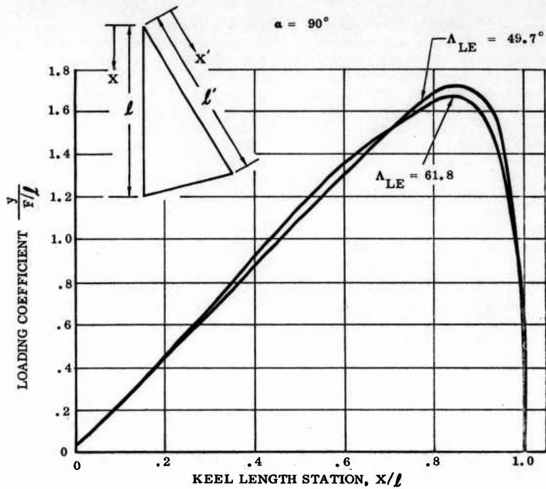
Figure 10 Theoretical Keel and L. E. Membrane Load Distribution
