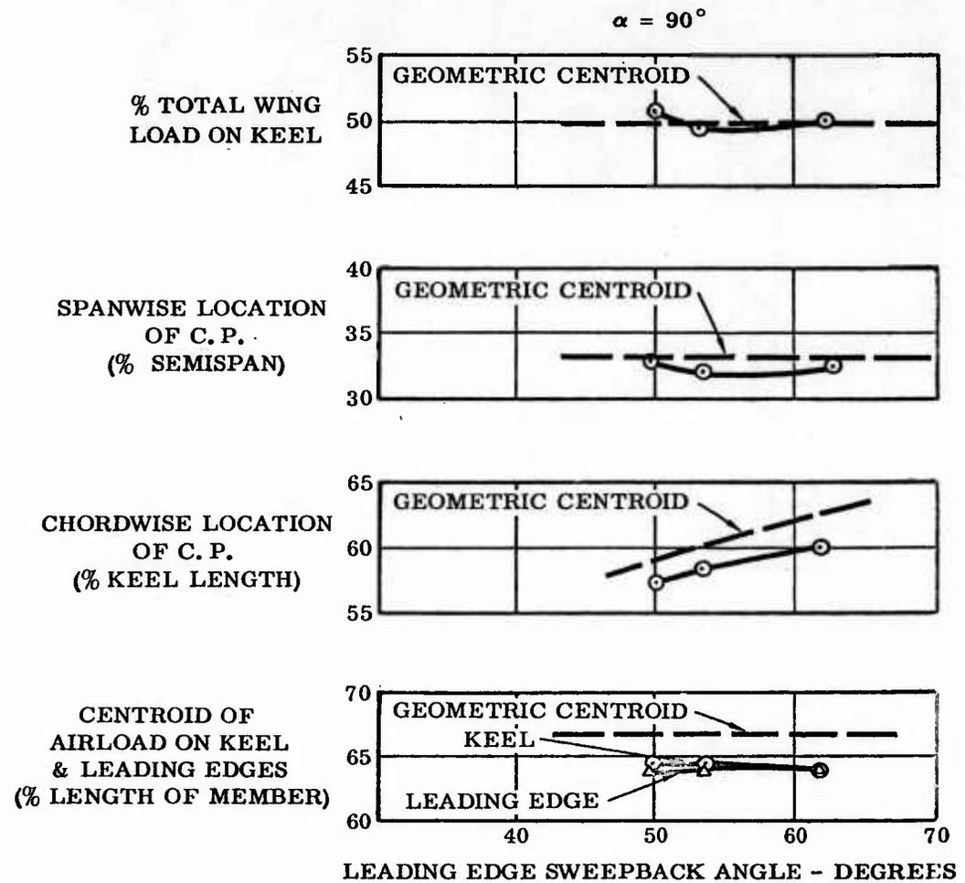
Figure 11 Theoretical Wing Airload Characteristics
