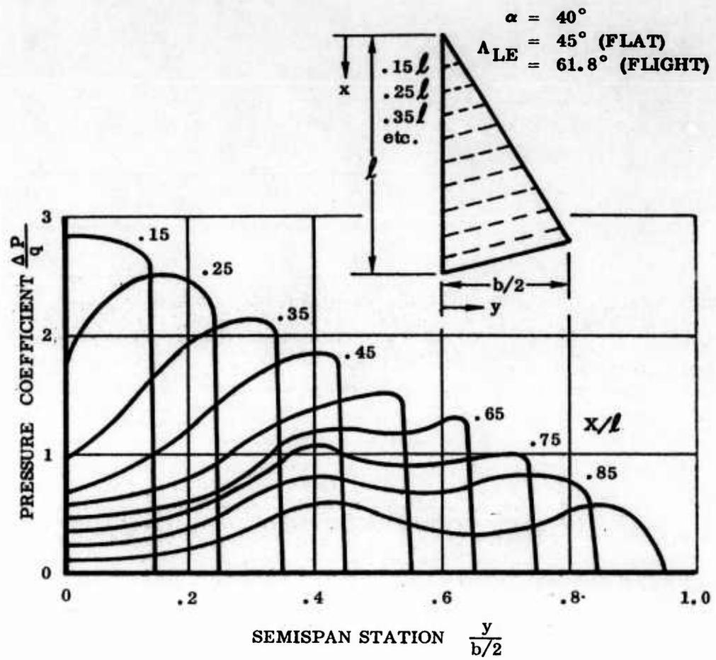
Figure 11a Theoretical Wing Airload Distribution
