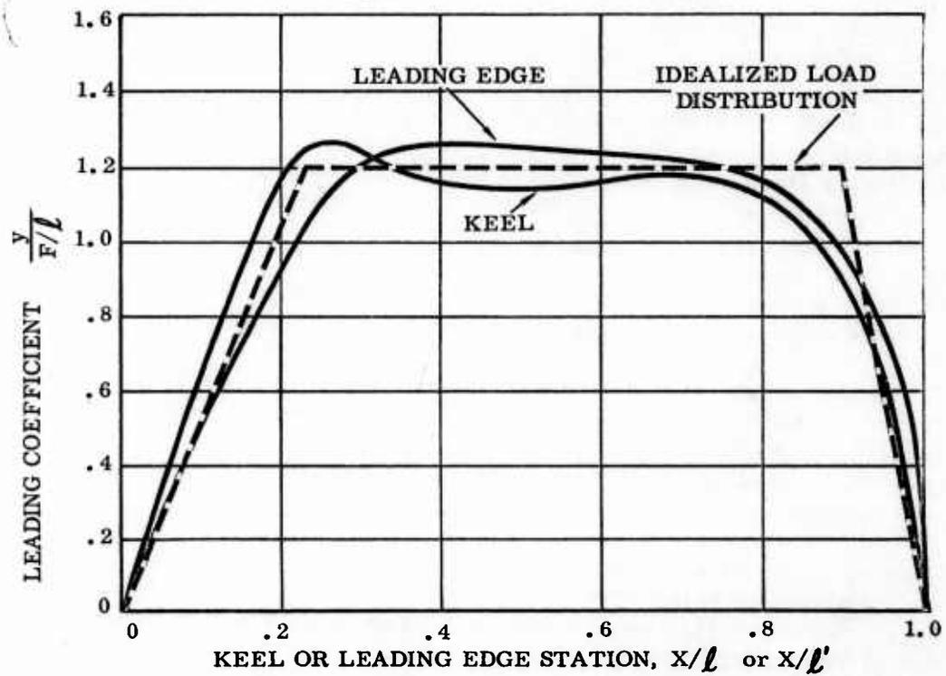
Figure 12 Theoretical Keel and L. E. Membrane Load Distribution
