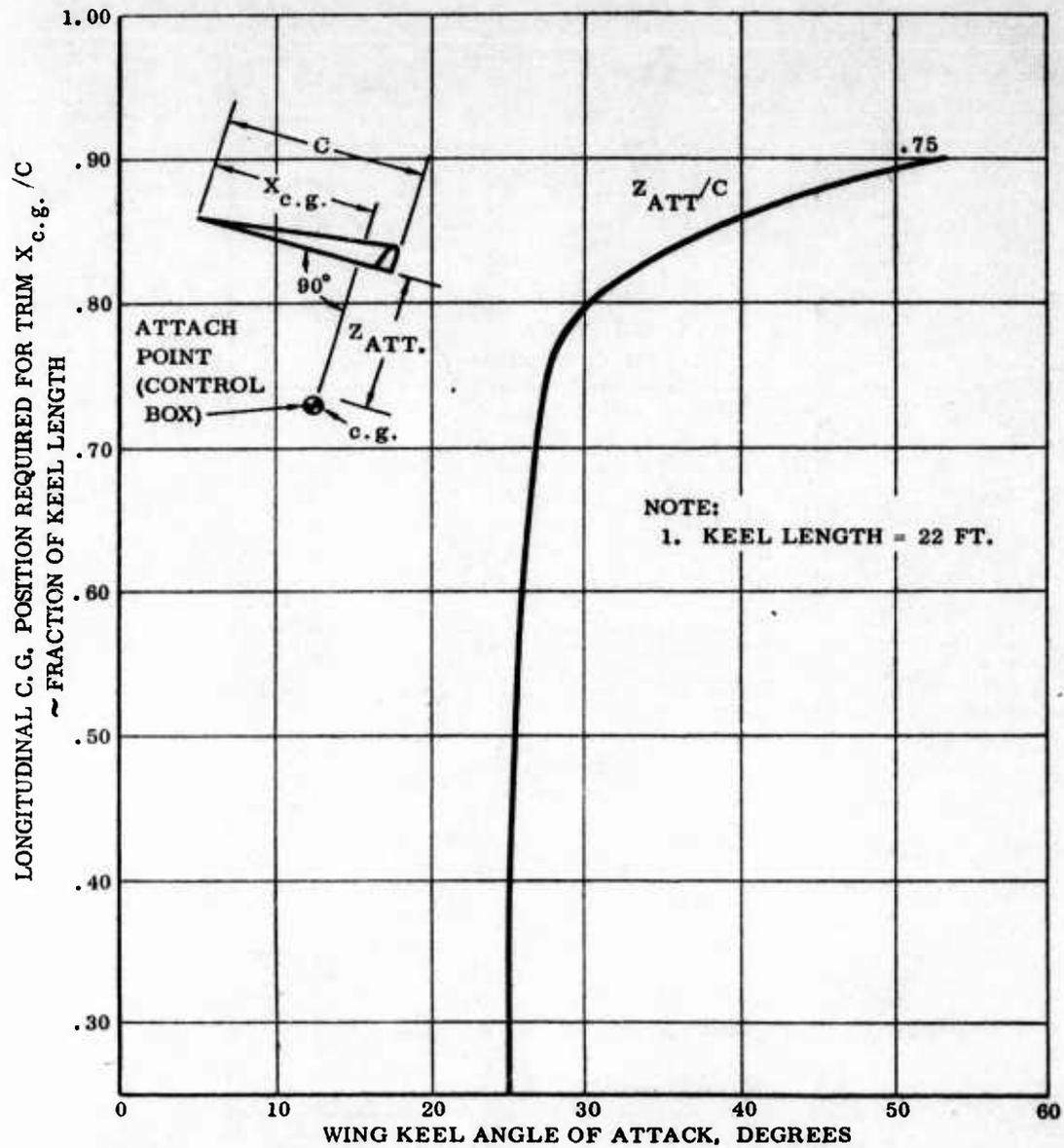
Figure 5 Theoretical Longitudinal C.G. Position Required for Trim
