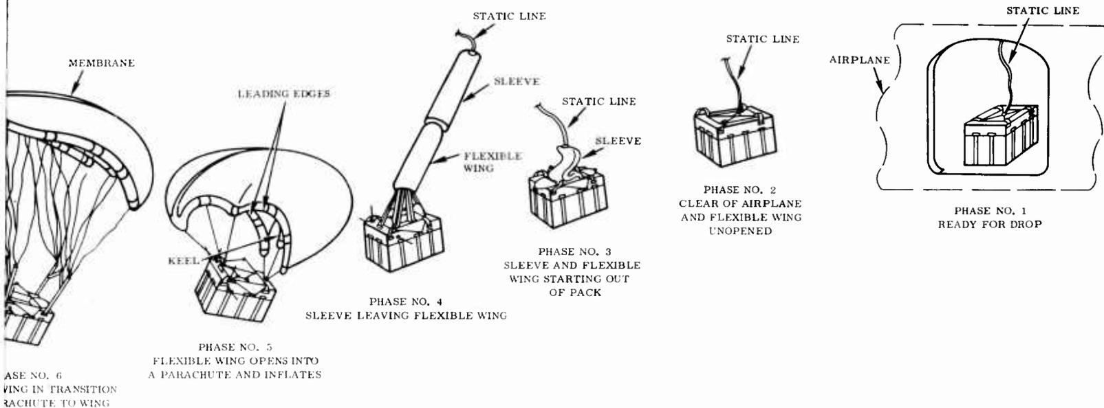
Figure 45 Glider Launch - Deployment Sequence
