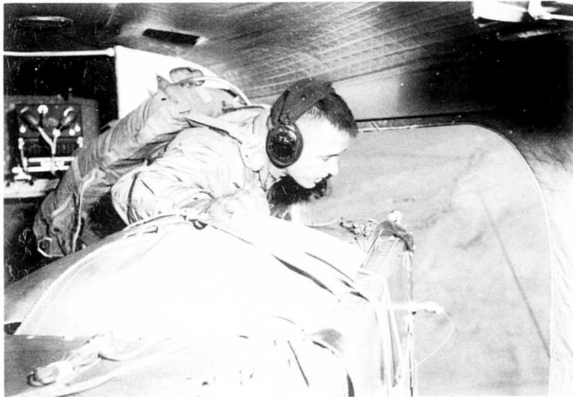
Figure 43 PDG Launch Procedure - Unfasten Tiedown Strap
