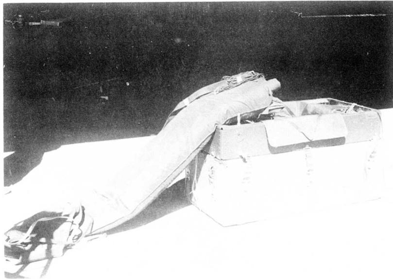
Figure 37 Wing Alignment to Control Box Storage Pan
