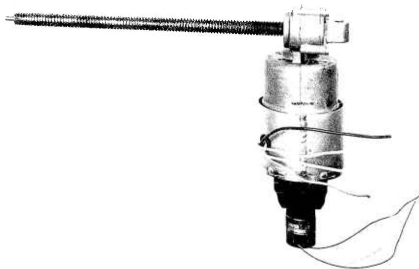
Figure 20 Paraglider Control Servo Motor
