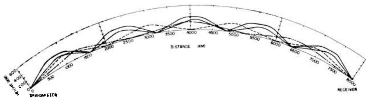
FIG. 2. CROSS SECTION OF IONOSPHERIC RAY PATHS.
