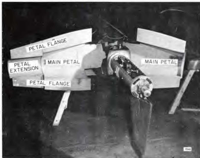
FIGURE 10 PETAL CONSTRUCTION: FULL-OPEN POSITION
