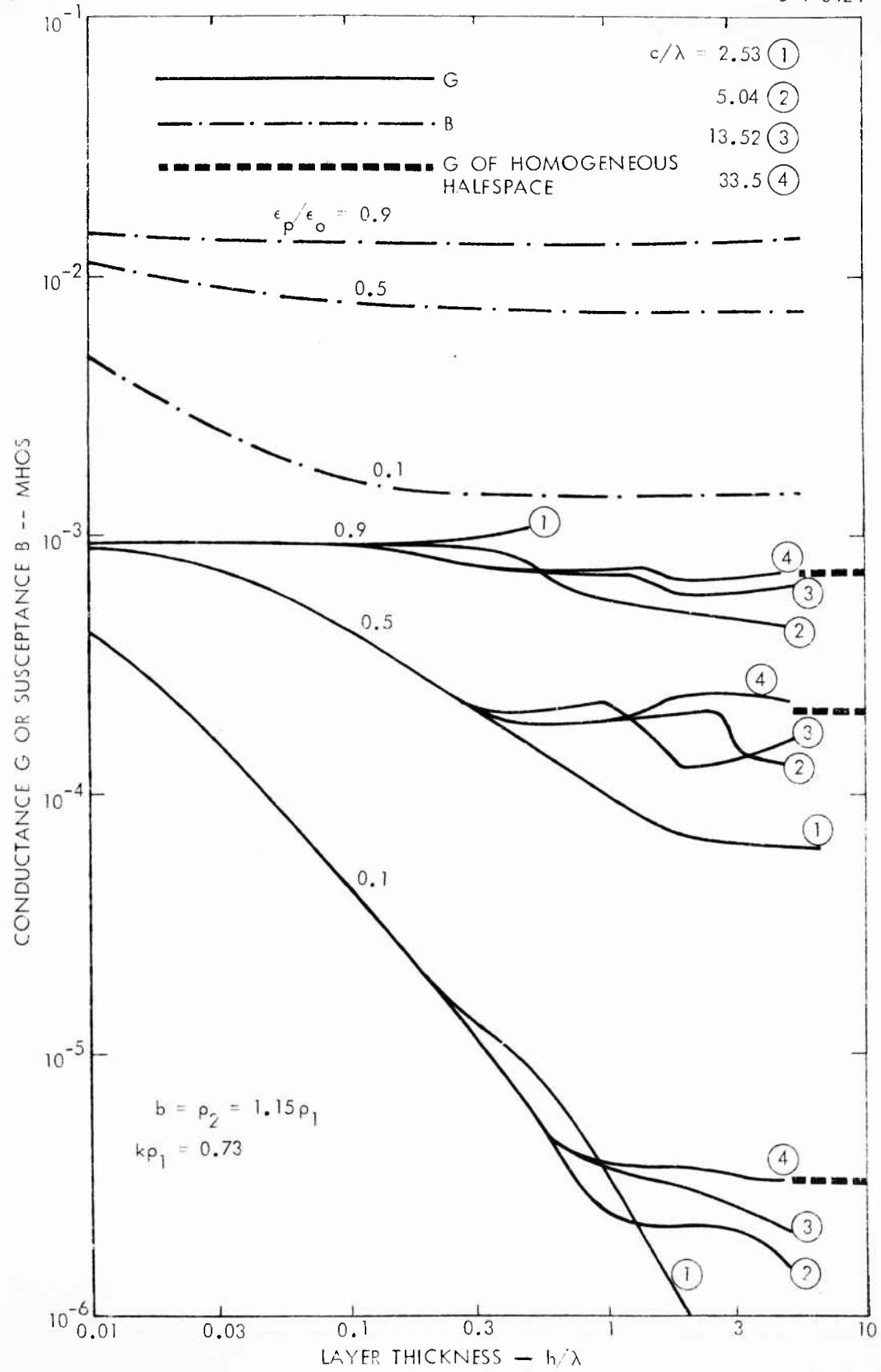
Figure 5. Slot Admittance for Lossless Plasma Layers
