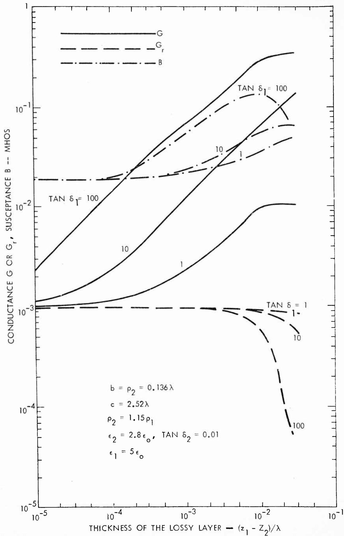
Figure 10. Admittance of a Slot Covered by Lossy Dielectric at a Distance  $Z_2 = 3 \times 10^{-3}\lambda$
