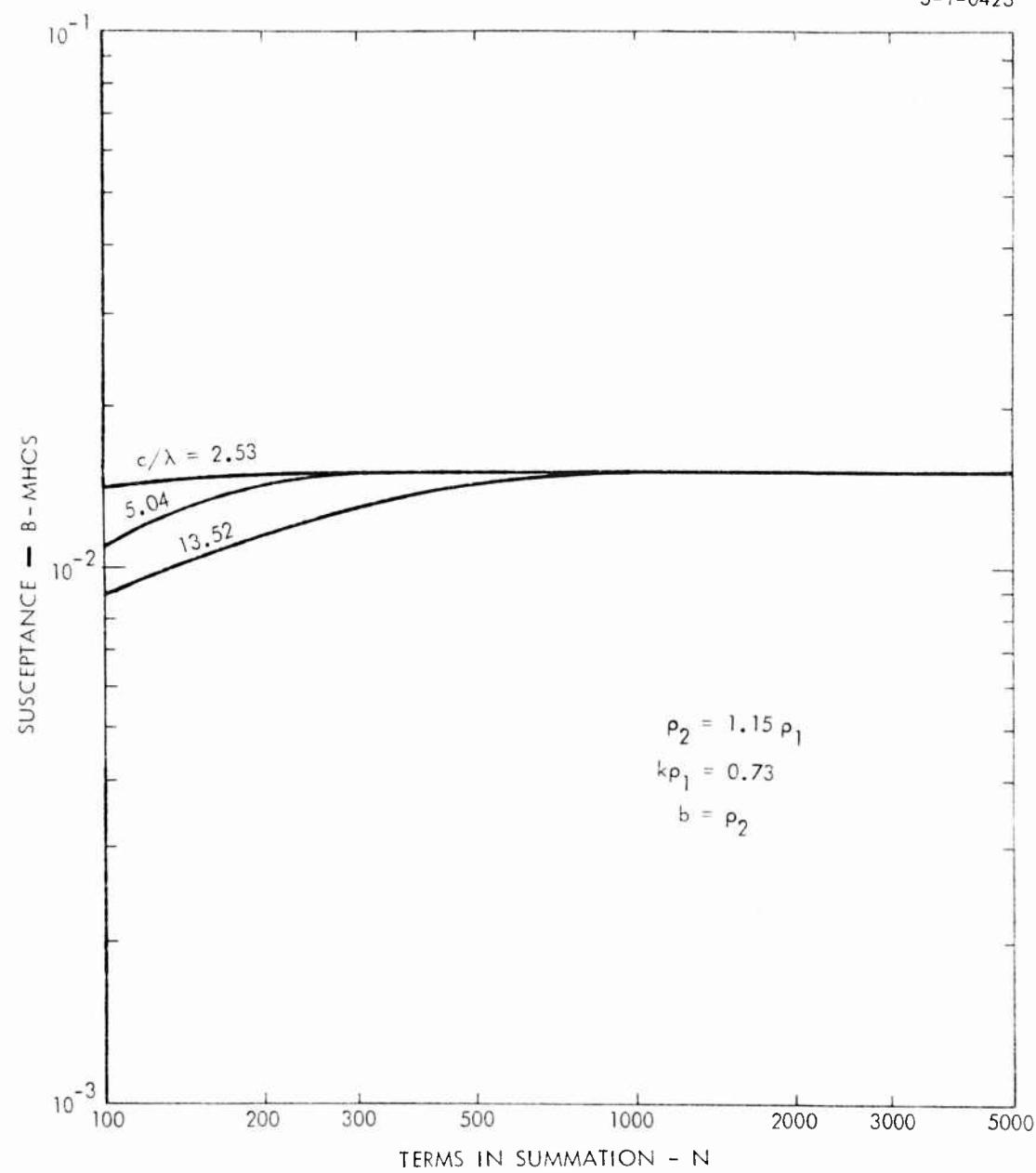
Figure 4. Susceptance of the Annular Slot
