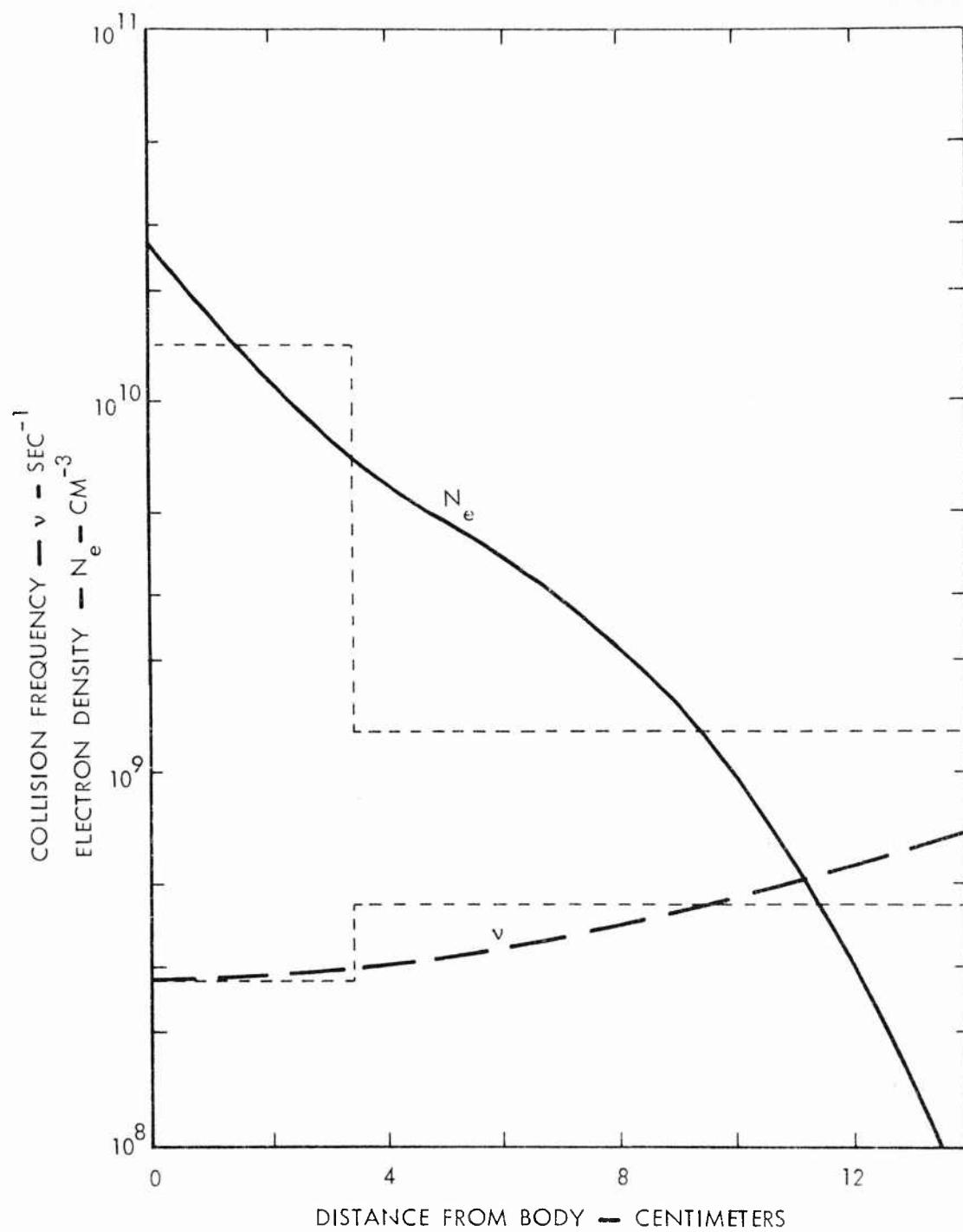
Figure 7. Profile of Electron Density and Collision Frequency and the Two Layer Approximation.
