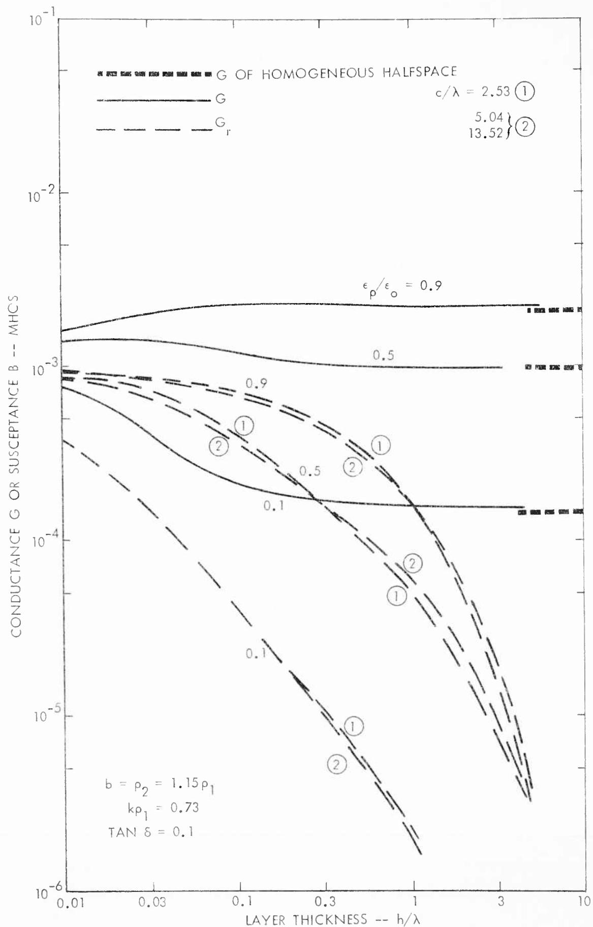
Figure 6. Slot Admittance for Lossy Plasma Layers
