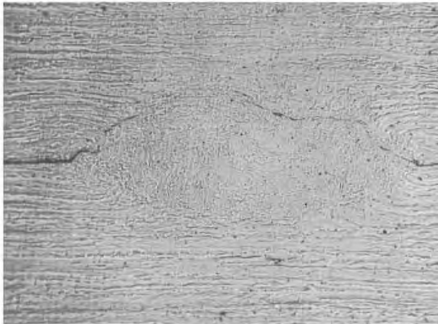
b. 0.010-Inch, Lot 4, Slightly Contaminated Magnification: 500X
