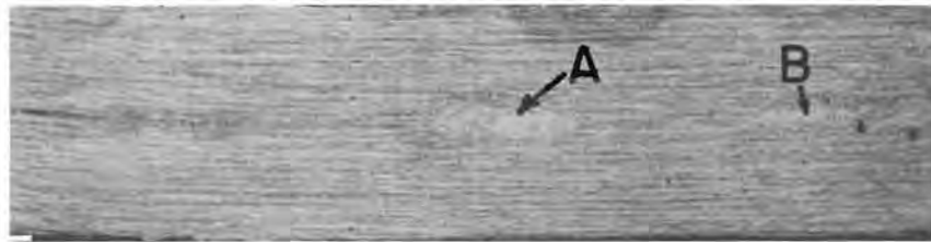
a. Cross Section Showing Excellent Bond With Heavy Local Interpenetration (A and B)
