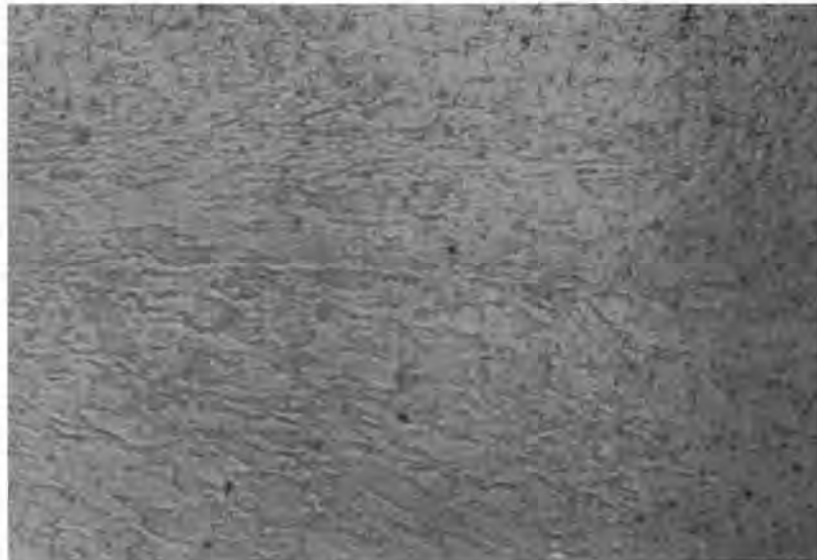
b. Detail A of Section a Above, Showing Intimacy of Bond Magnification: 500X
