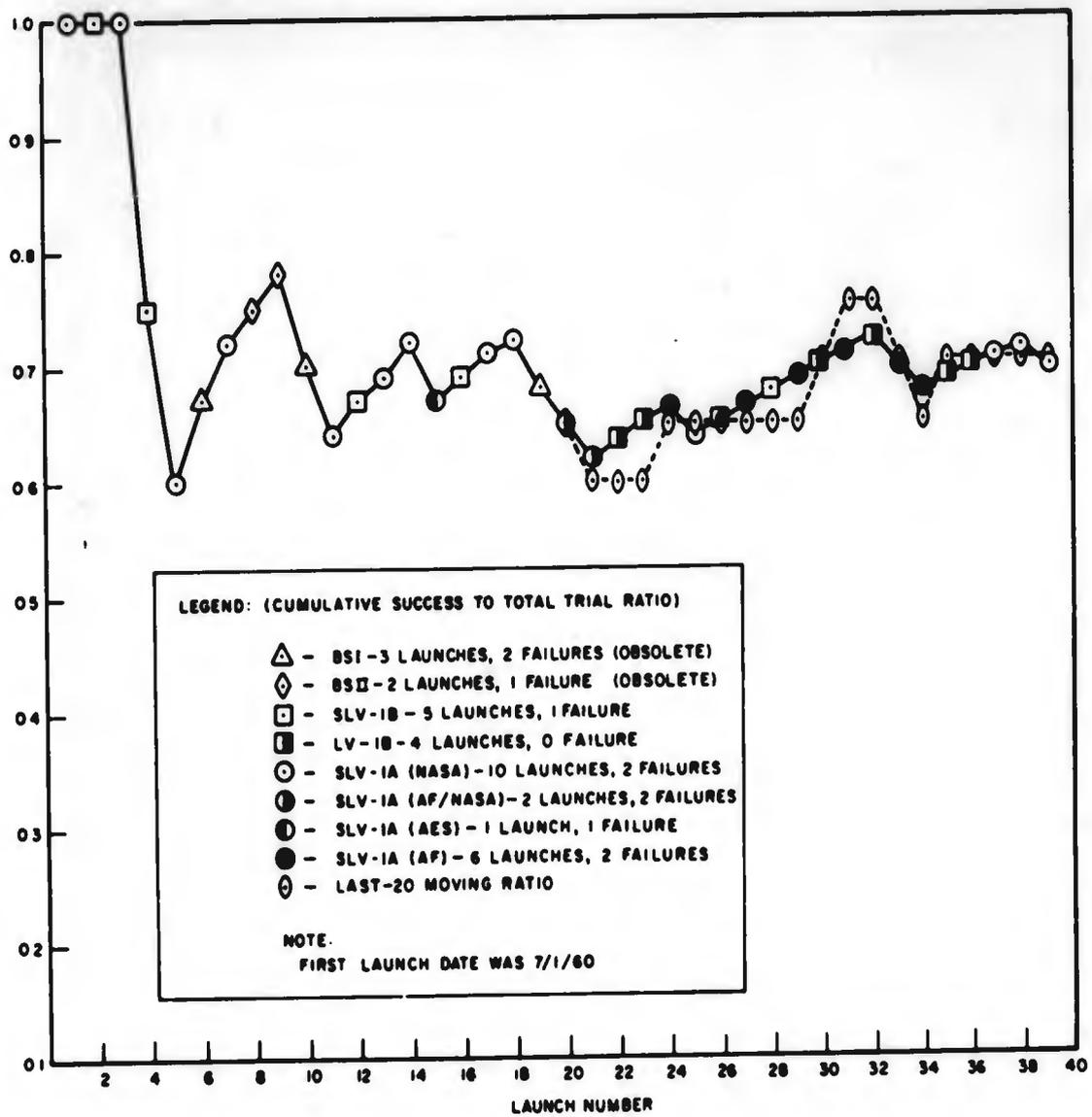
Figure 10. SLV-I Success Ratio vs Launch Number
