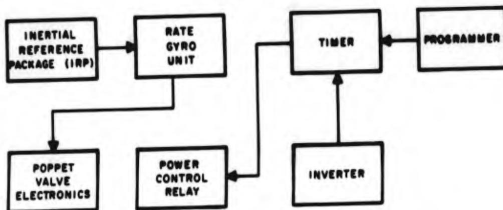
Figure 5. BSII Guidance System Block Diagram
