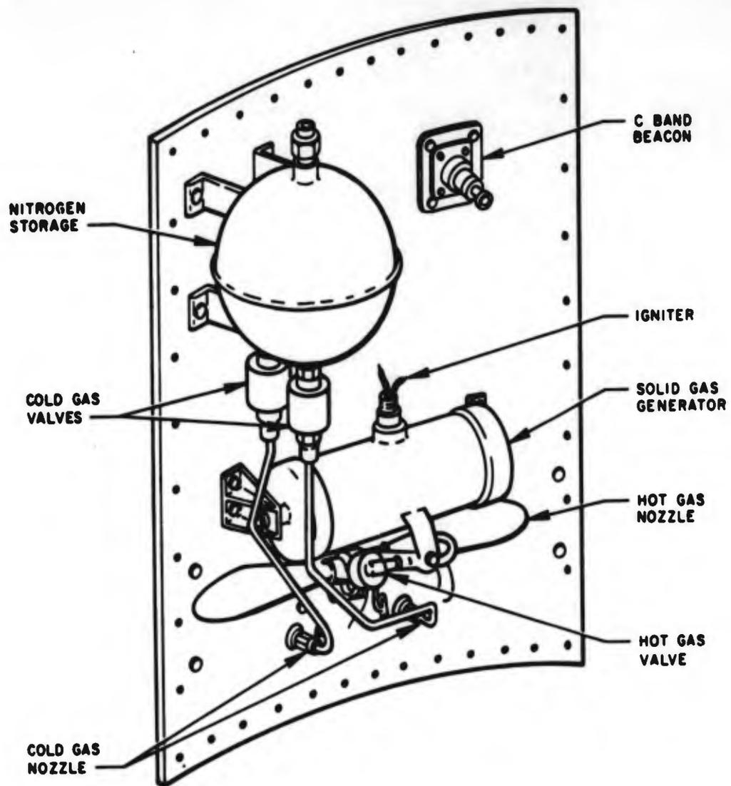
Figure 6. BSII Hot and Cold Gas Control Panel
