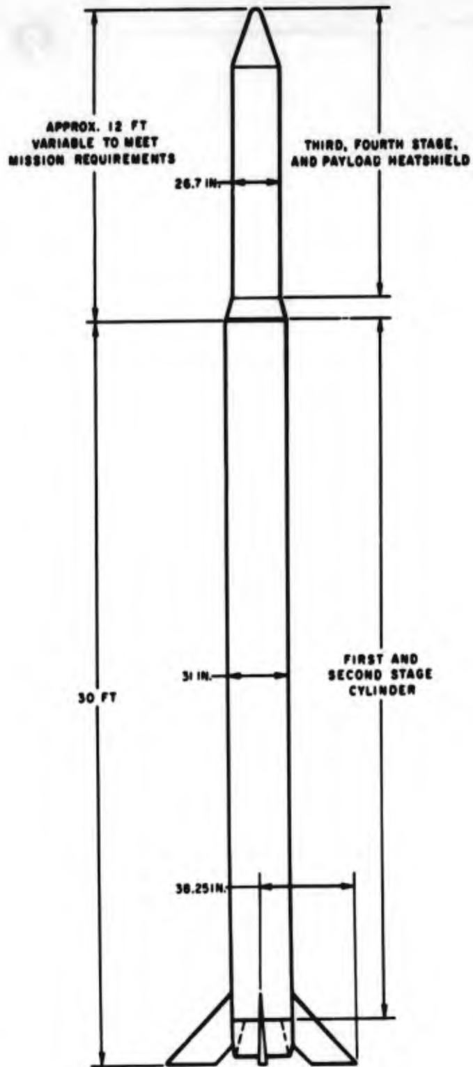
Figure 3. SLV-1B, External View of New Configuration
