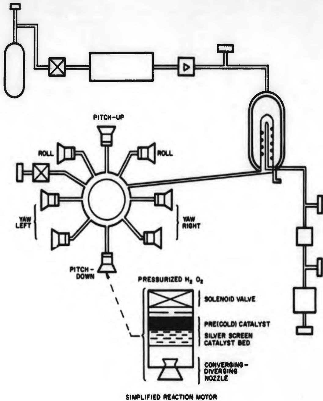
Figure 9.  $H_2O_2$  Reaction Control System
