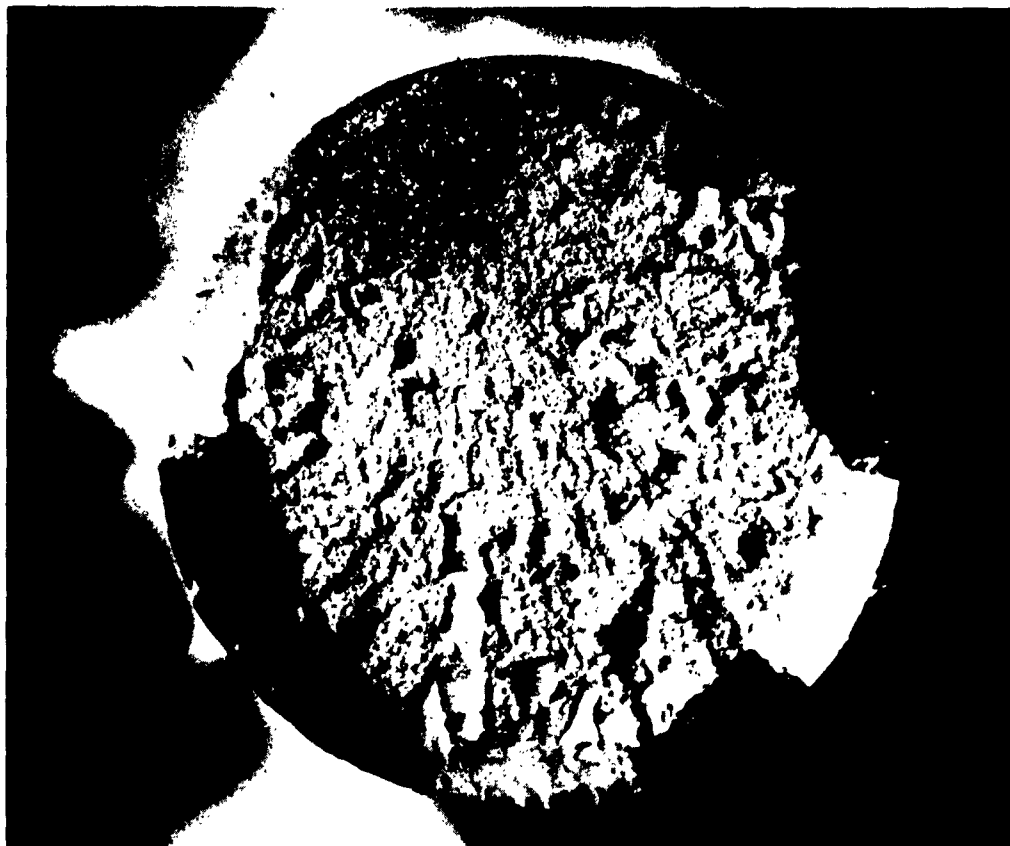
Figure 5 - ALLOY SEGREGATION EXPOSED BY STRESS CORROSION CRACKING IN A 4340 FORGED PART SPECIMEN. 20X
