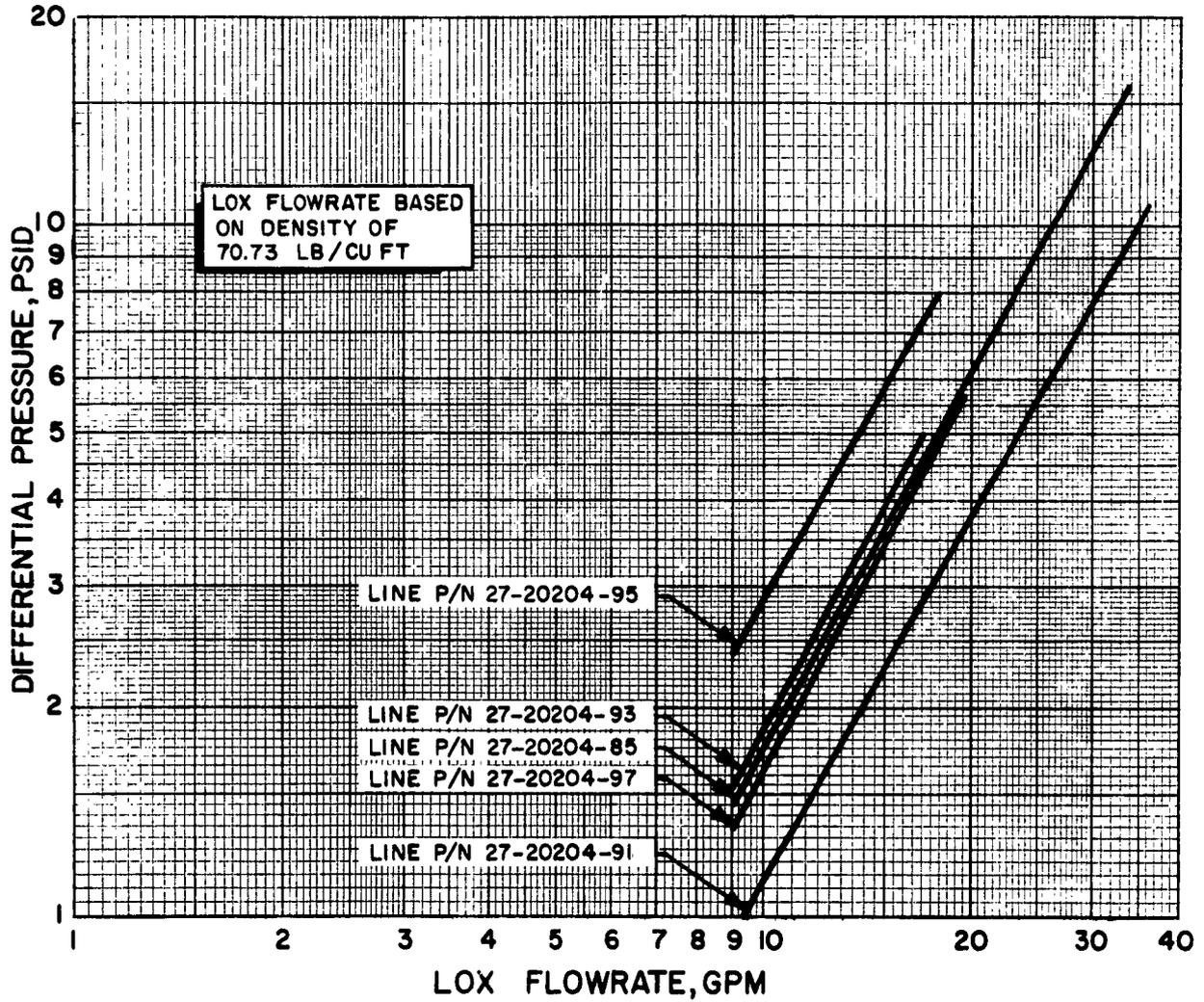
Figure A-5. Differential Pressure Through GD/A Start System Lines at Various LOX Flowrates
