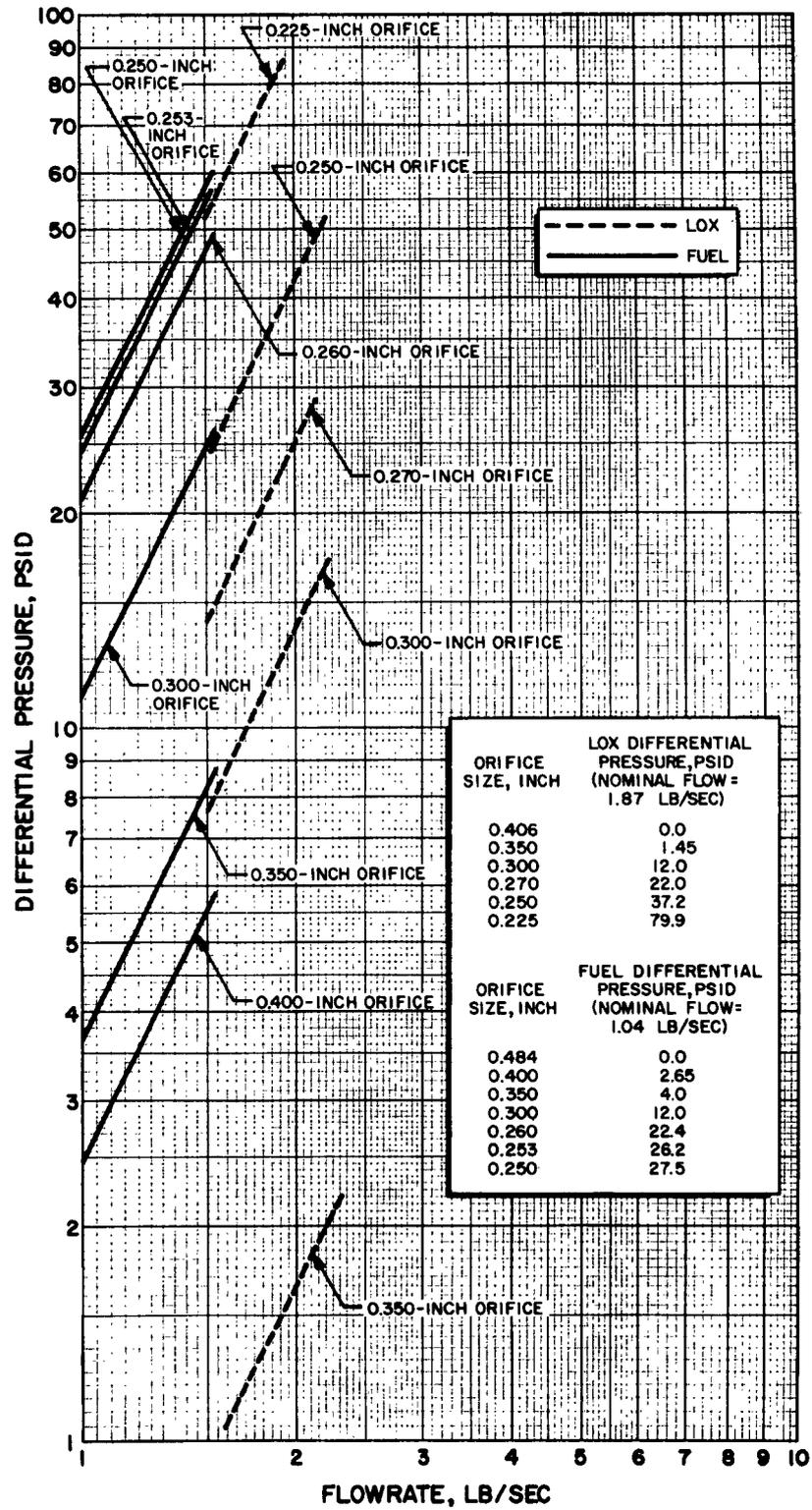
Figure 16. Phase II Orifice Pressure Losses at Various Flowrates
