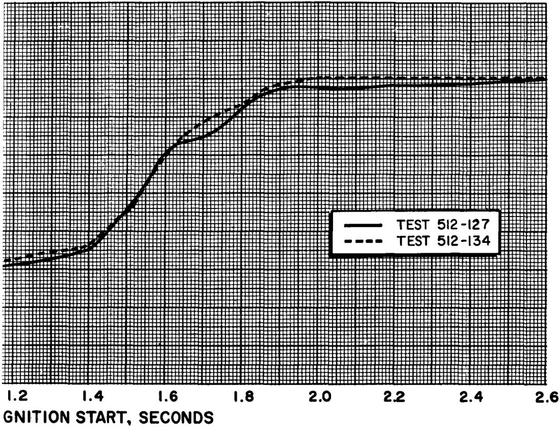
Figure 5. Gas Generator Fuel Injection Pressure Profile After Ignition Start
