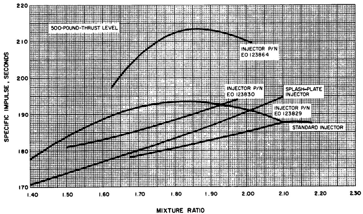
Figure 37. Site Specific Impulse at Various Mixture Ratios
