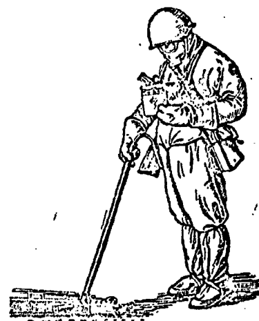
Fig. 23. Position of radiometer during measuring.
