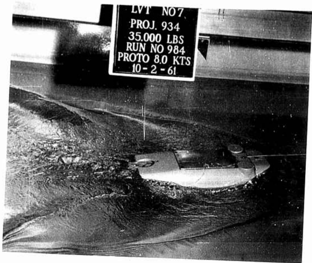
FIGURE 3.9.12 MODEL NO. 7—MAXIMUM WATER PERFORMANCE VEHICLE
