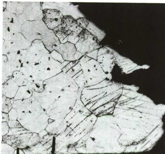
C. Heat Affected Zone of Weld Exposure: 100 Cycles from 75° to 800° F Etchant: Kroll's Magnification: 250 X
