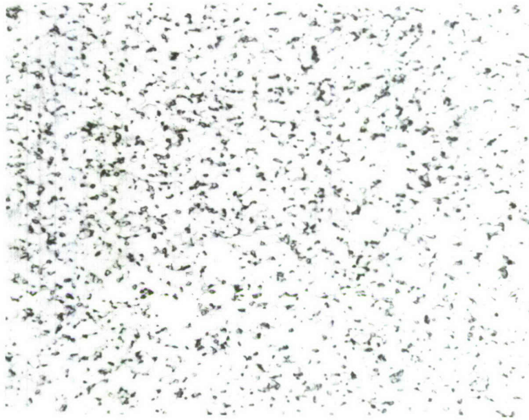
Figure 7. Photomicrograph of Titanium-8Al-1Mo-1V Alloy (Annealed) Etchant: Kroll's Magnification: 500 X
