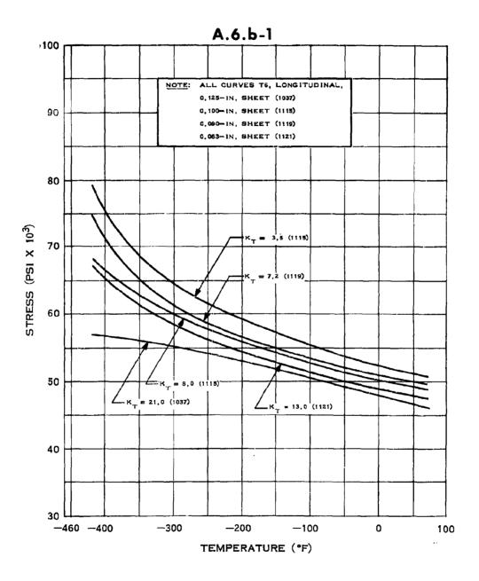
NOTCH TENSILE STRENGTH OF 6061 ALUMINUM
