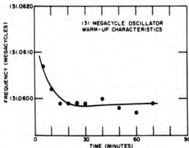
Fig. 16 - 131-Mc oscillator warm-up characteristics
