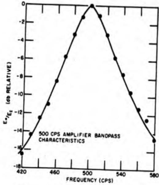
Fig. 8 - 500-cps amplifier bandpass characteristics
