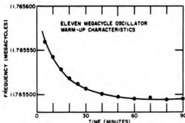
Fig. 15 - 11.7655-Mc oscillator warm-up characteristics
