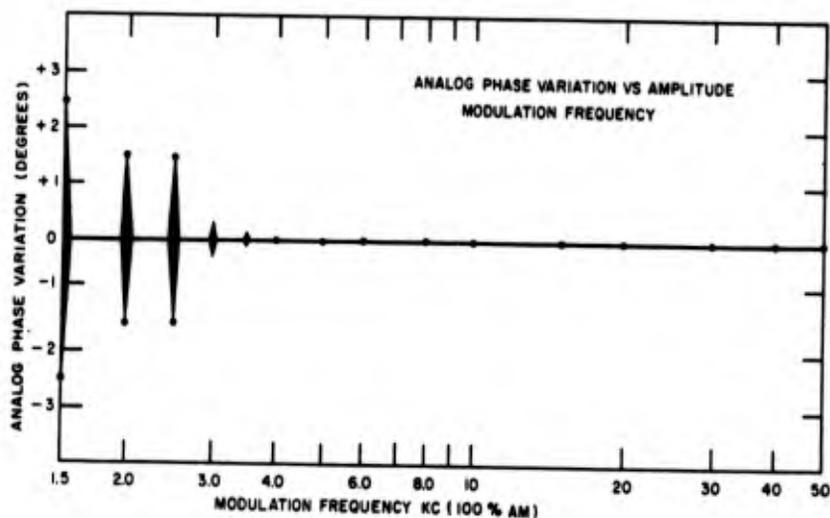
Fig. 12 - Analog phase variation vs amplitude modulation frequency
