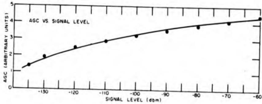
Fig. 9 - AGC vs signal level
