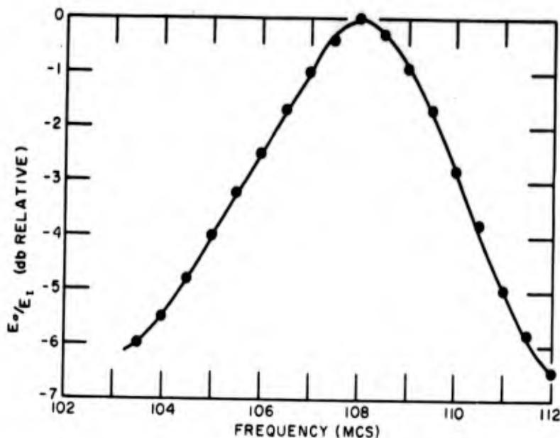
Fig. 3 - Front end bandpass characteristics
