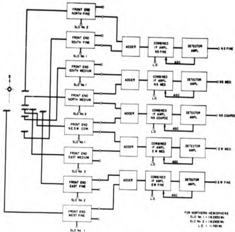
Fig. 1 - Minitrack receiver block diagram
