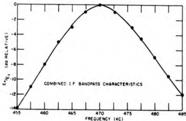
Fig. 7 - Combined i-f bandpass characteristics
