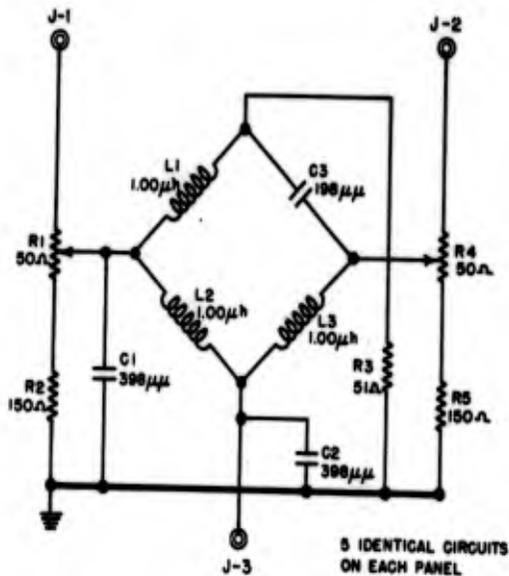
Fig. 4 - Signal adder unit
