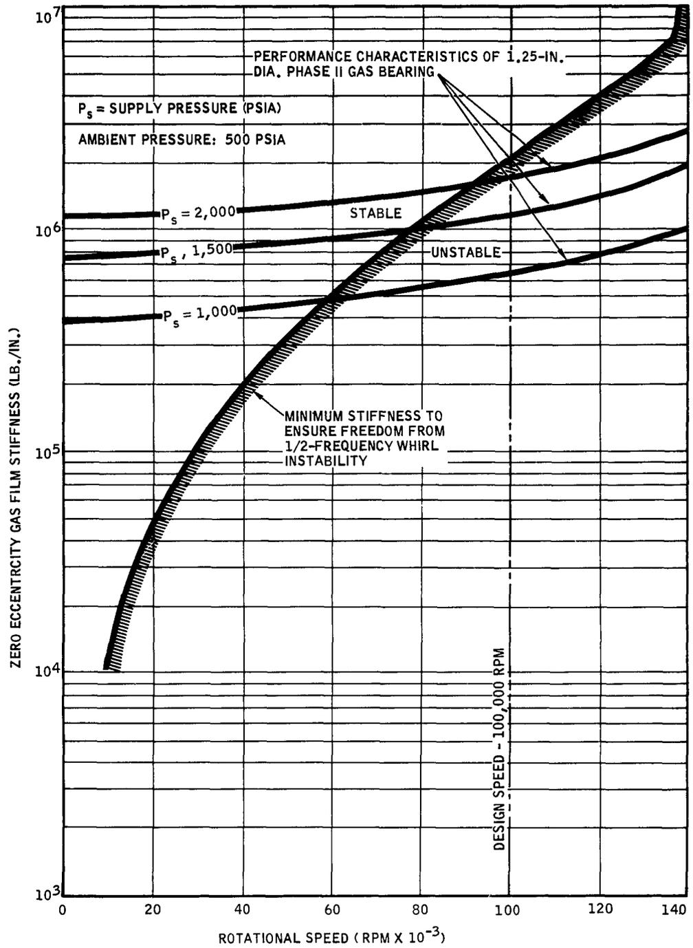
Figure 2. Stability Characteristics of Configuration A Design
