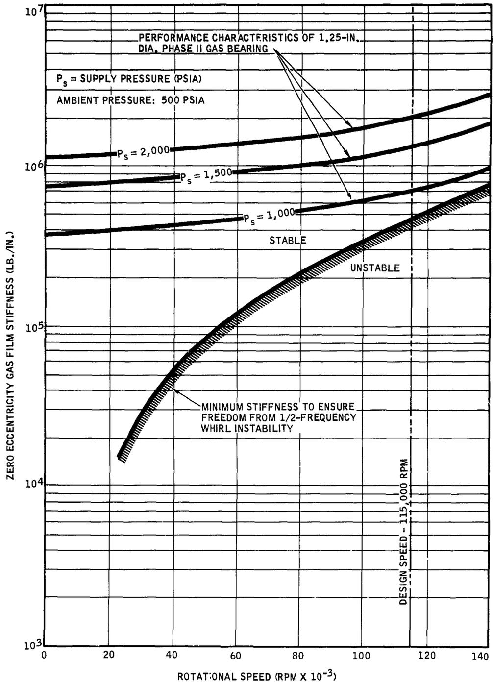
Figure 6. Stability Characteristics of Configuration B Design (0.35-In.-Dia. Impeller Shaft, With Shrouds)
