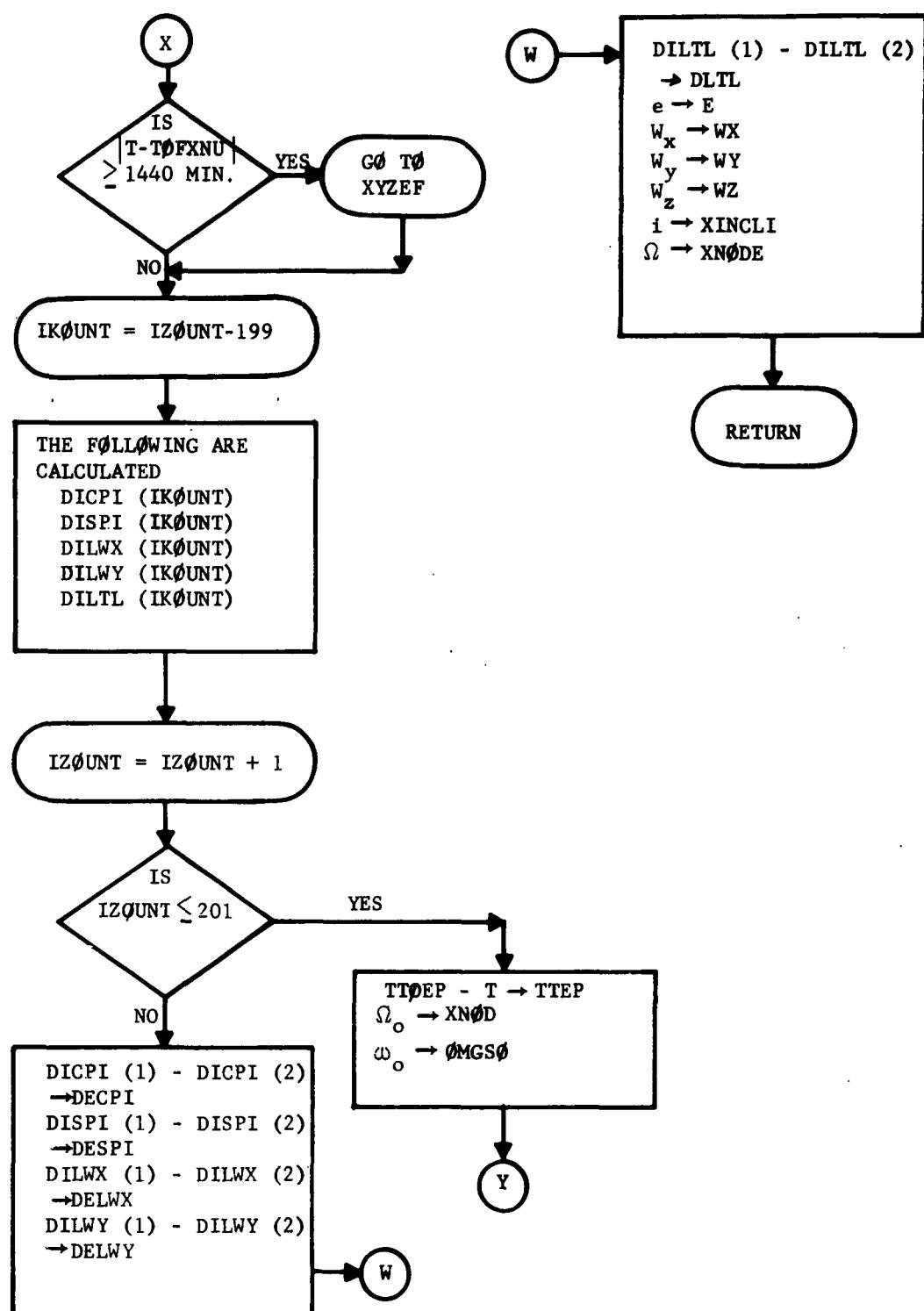
FLOW CHART OF RADIATION PRESSURE SECTION OF
