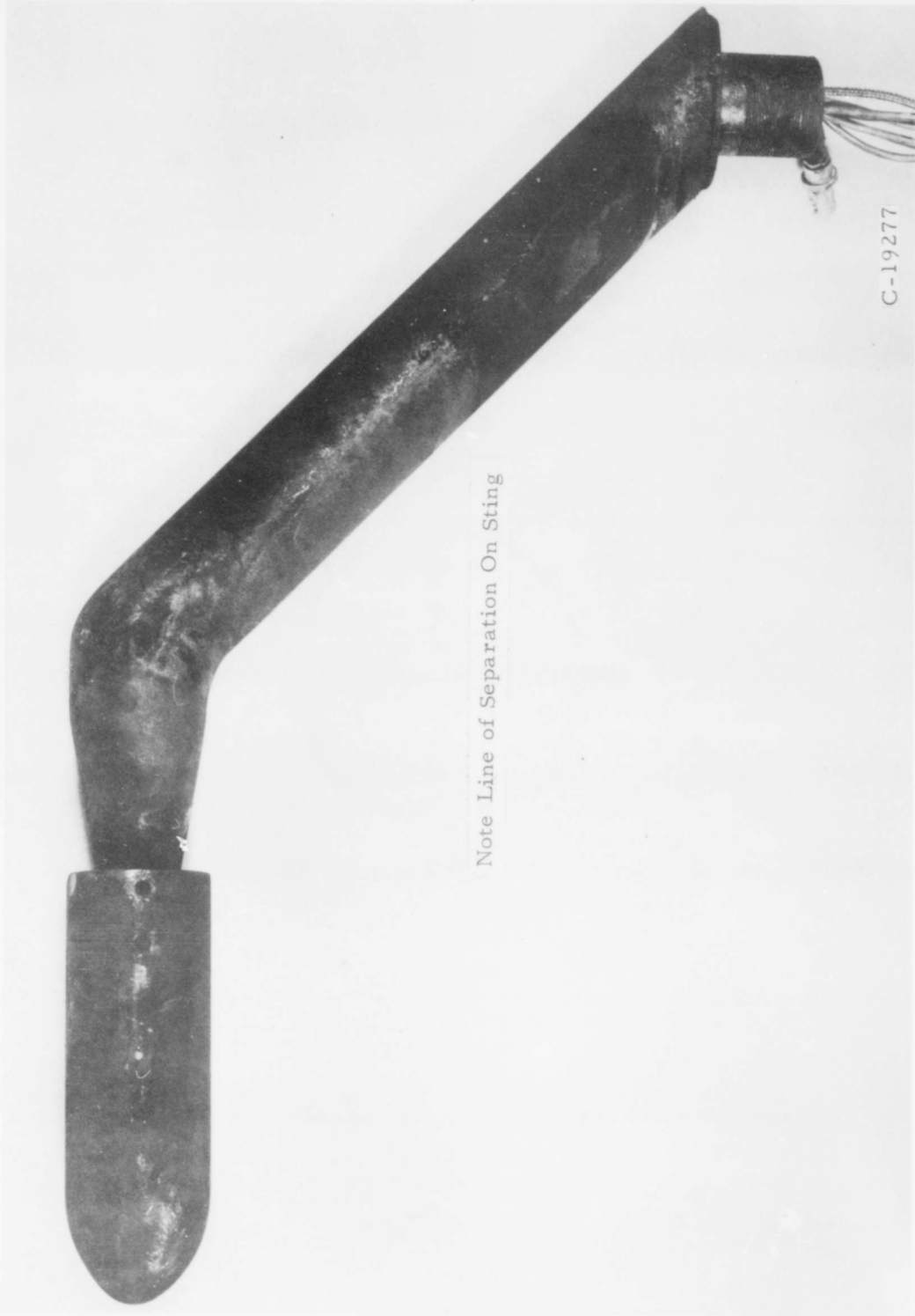
FIGURE 2.9. STING AND MODEL AFTER TEST
