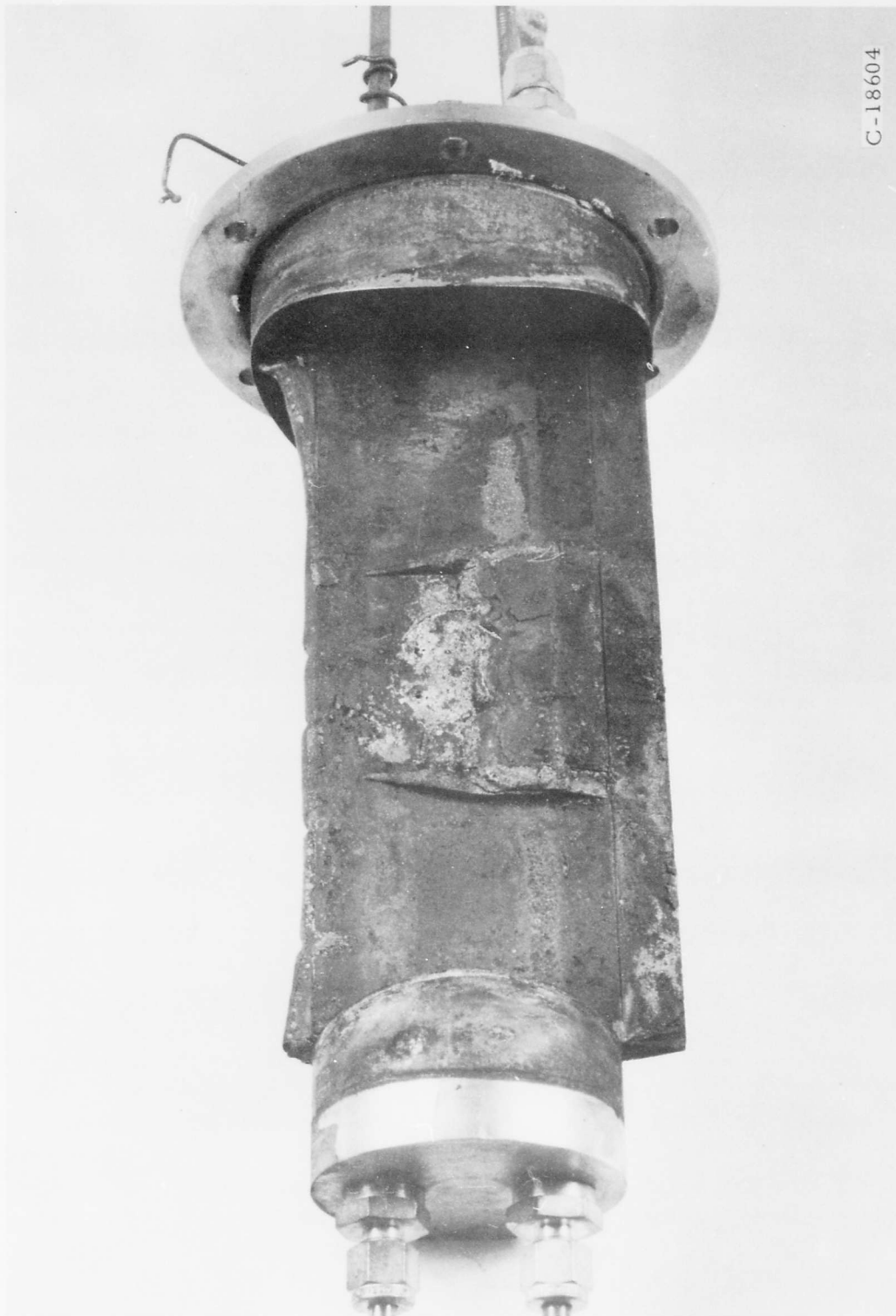
FIGURE 2.7. PLAN VIEW OF STAGNATION SIDE OF BROADVIEW GAGE AFTER FIRING IN TEST 2
