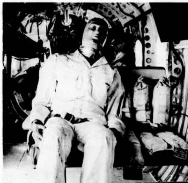
Figure 3. Front View of Seat, Showing Anthropomorphic
