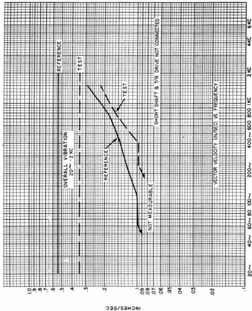
FIGURE 35. FWD ENGINE VIBRATION, VECTOR VELOCITY VS FREQUENCY, (REFERENCE AND TEST) (PART 1)
