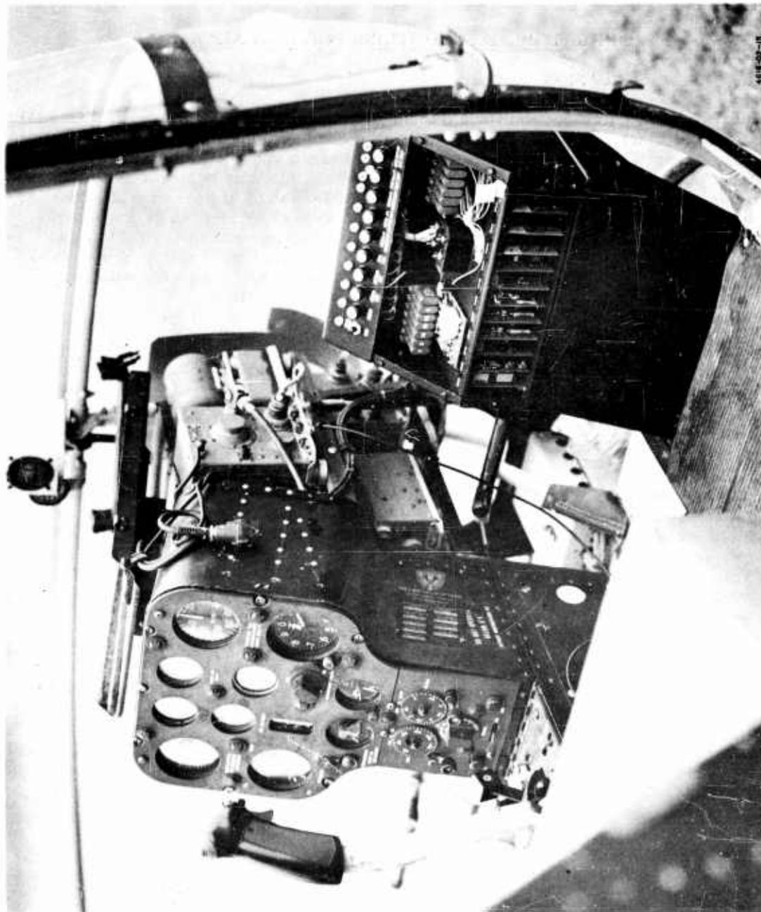
FIGURE 74. TEST ALARM SYSTEM INSTALLED IN H-23 AIRCRAFT
