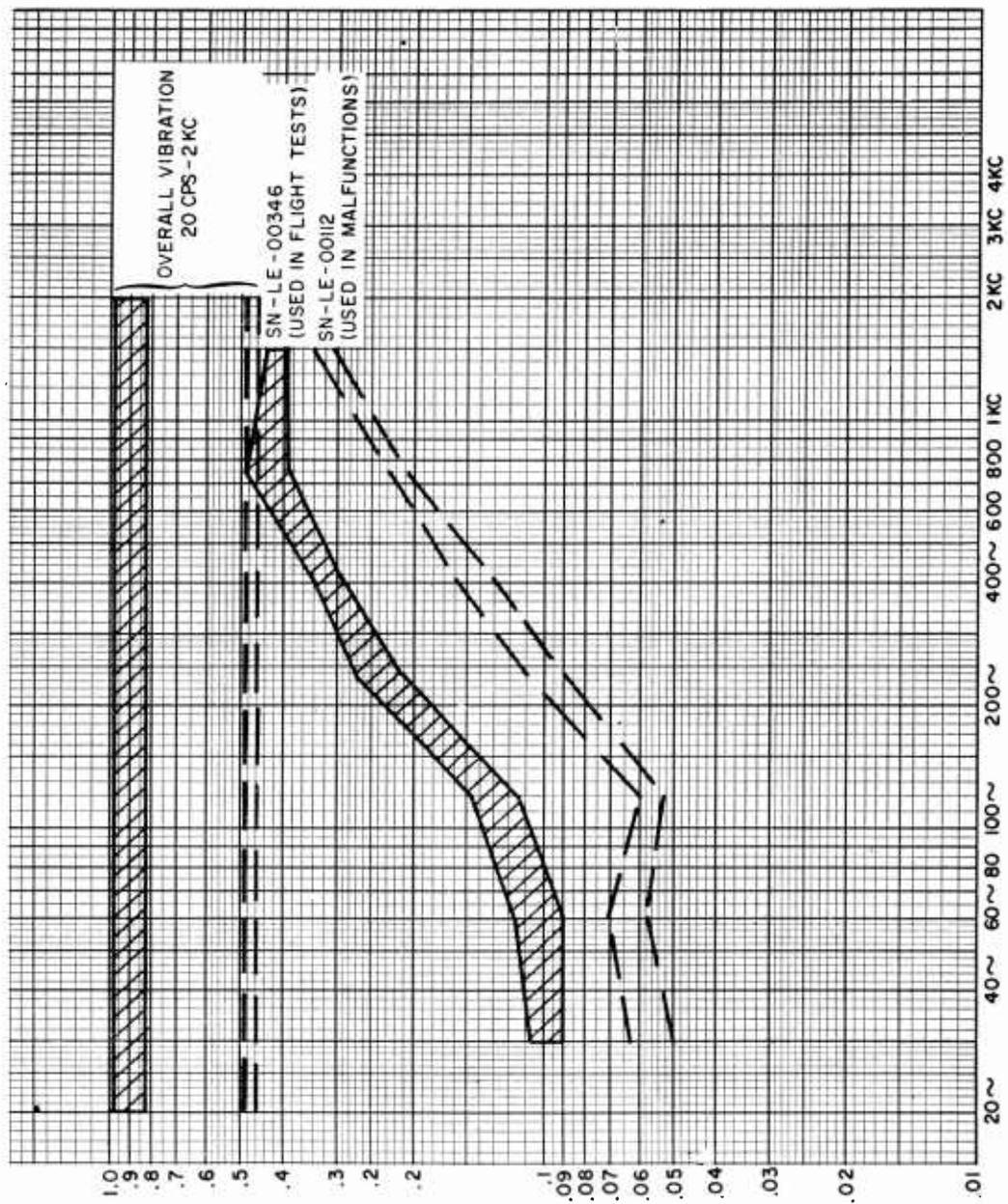
FIGURE 24. FWD ENGINE VIBRATION, ORIGINAL VS MALFUNCTION PLOT
