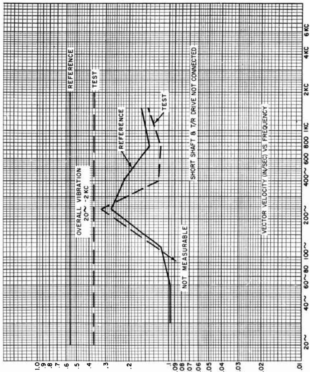
FIGURE 35. AFT ENGINE VIBRATION, VECTOR VELOCITY VS FREQUENCY, (REFERENCE AND TEST) (PART 2)
