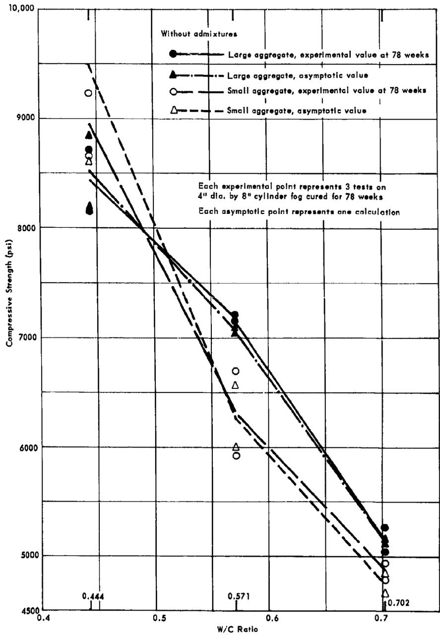
Figure 17. Experimental and asymptotic compressive strength versus W/C ratio - Phase III.
