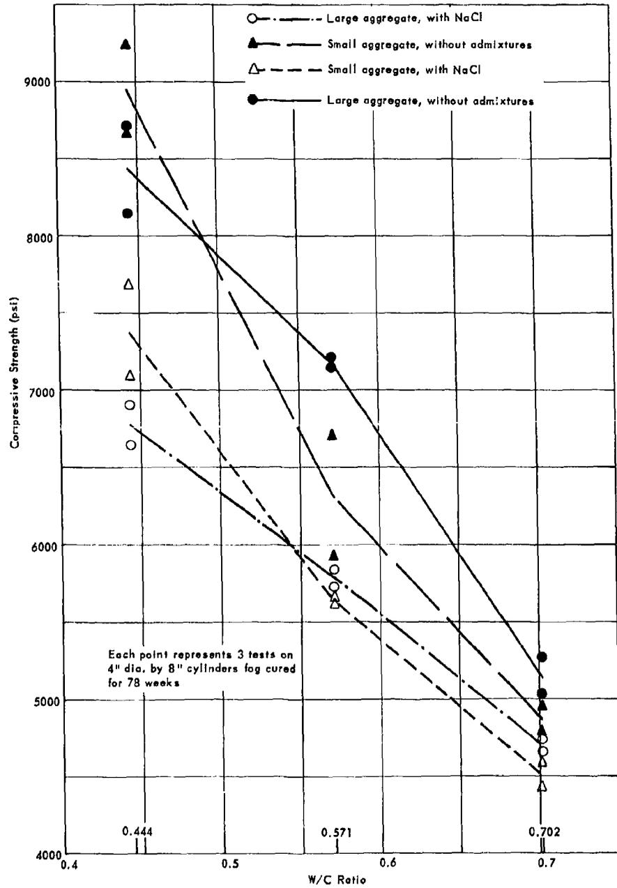
Figure 15. Compressive strength versus W/C ratio - Phase III, with and without NaCl.
