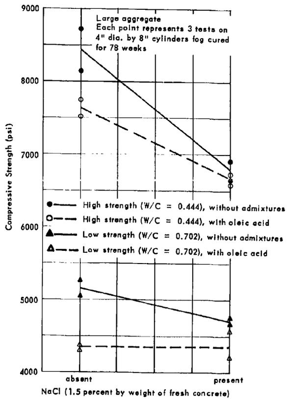
Figure 13. Compressive strength versus NaCl content - Phase III.
