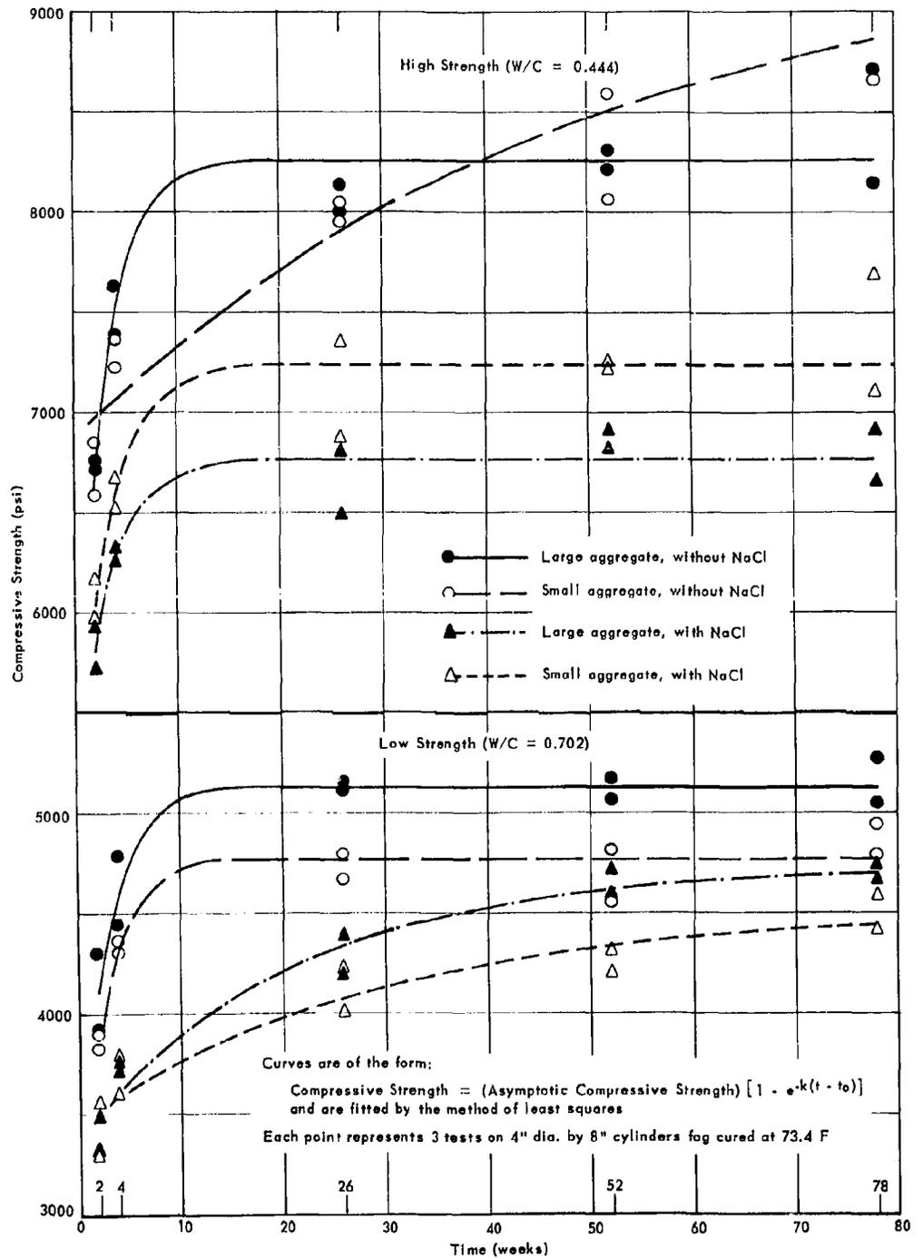
Figure 12. Compressive strength versus time - Phase III.
