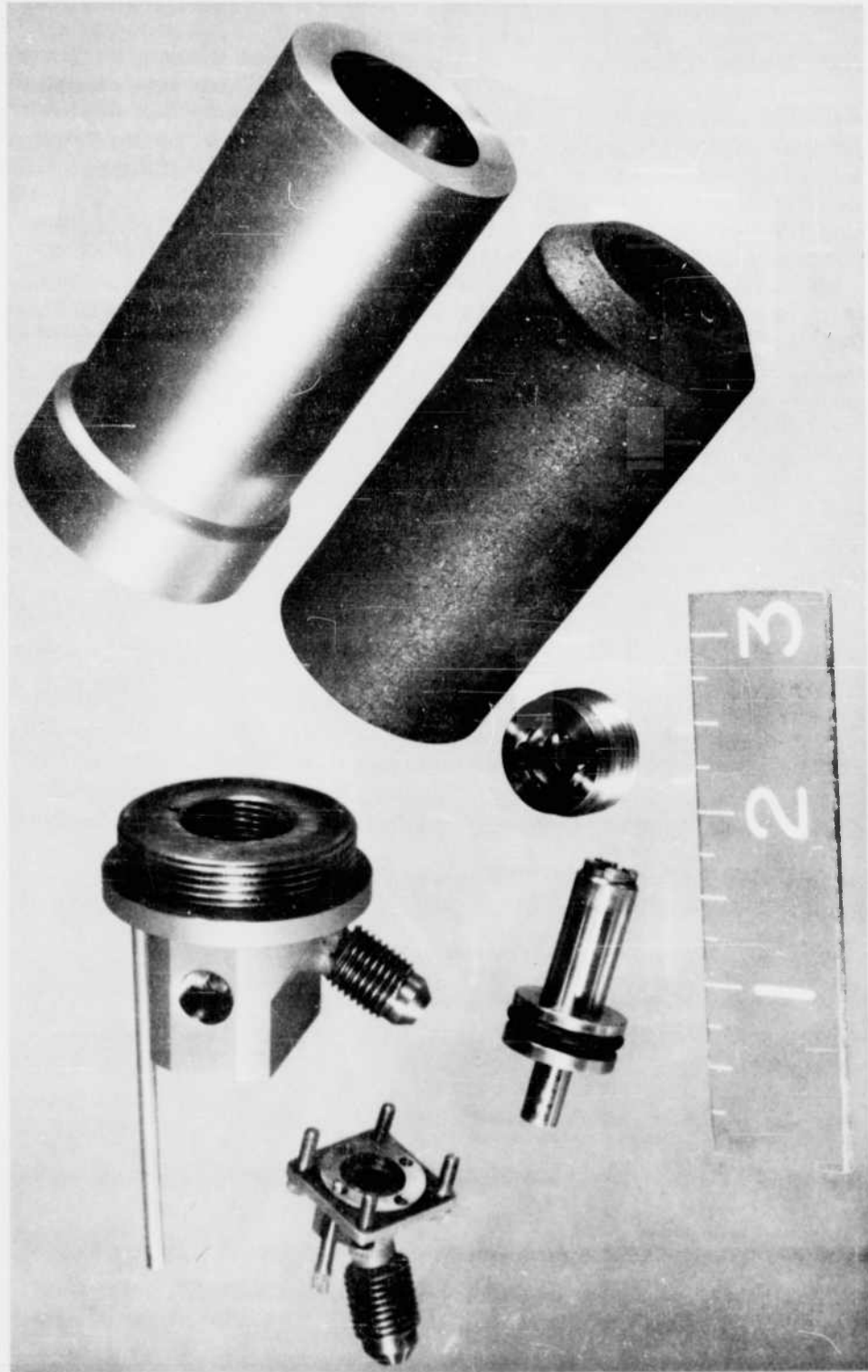
FIG. 3. Disassembled Uncooled Chamber and Injector.
