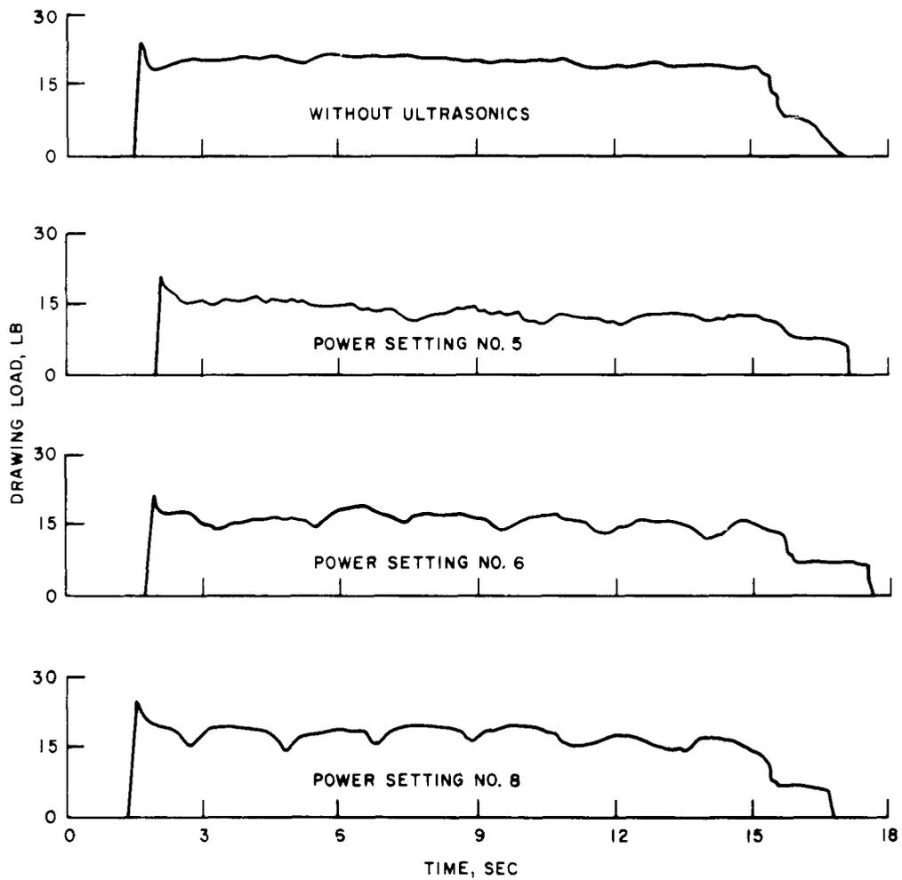
FIG. 10. Load Versus Time Curves for the Drawing of Copper Wire. Draw speed: 1.56 in/sec,  $D_o$ : 0.0403 in.,  $D_f$ : 0.0365 in., Area reduction: 18%.
