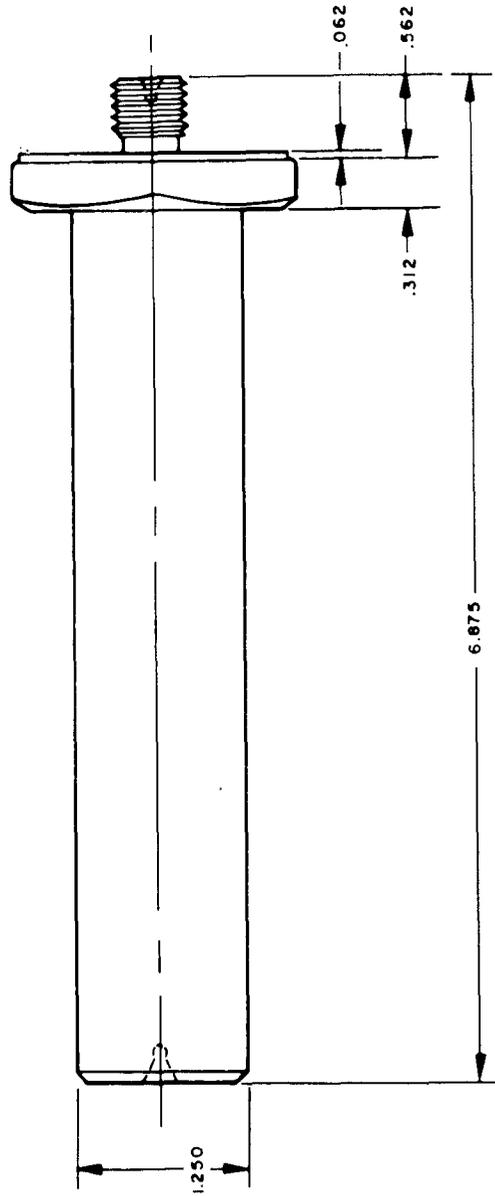
FIG. 6. Load Cell Adapter.
