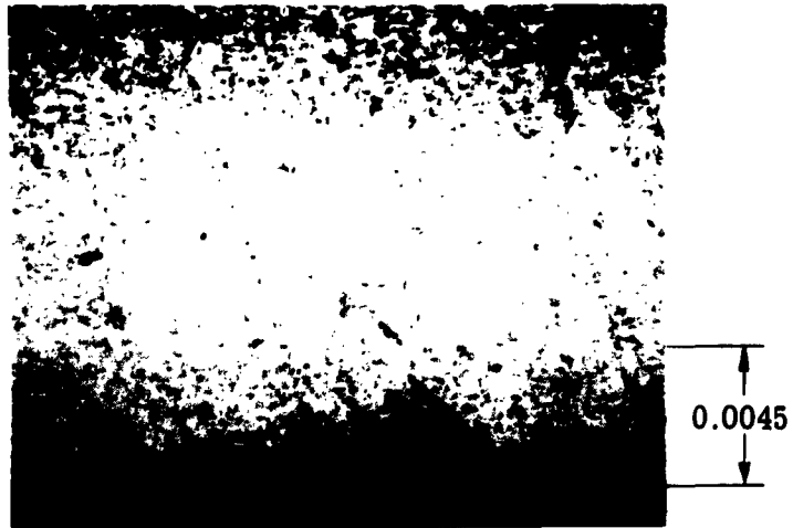
Figure 7. Secondary Fracture of 18-9-5 Mar-aging Steel (about 250X, Schantz Etch)
