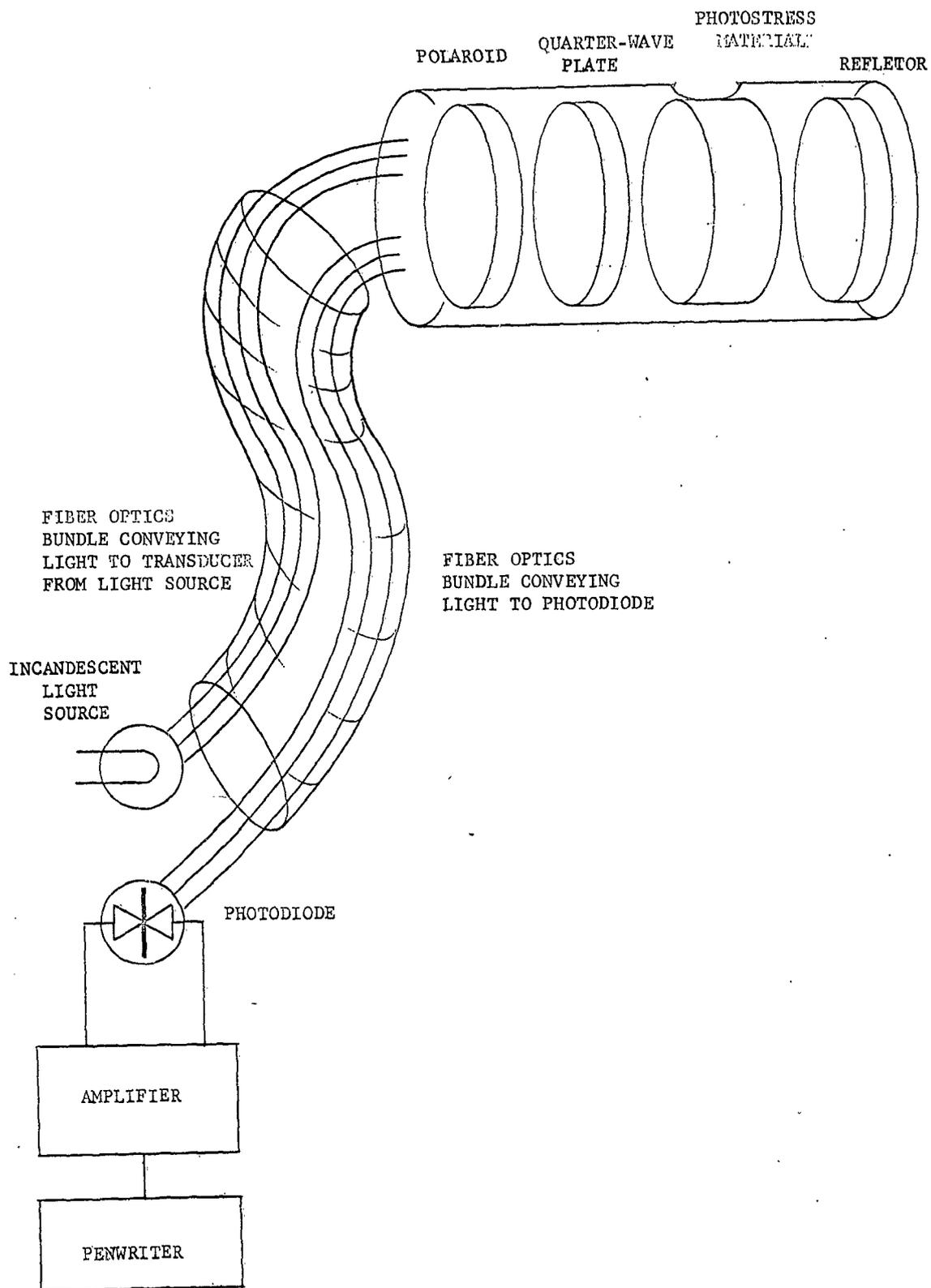
Figure 7. Optical Transducer Catheter - Amplifier-Recorder System
