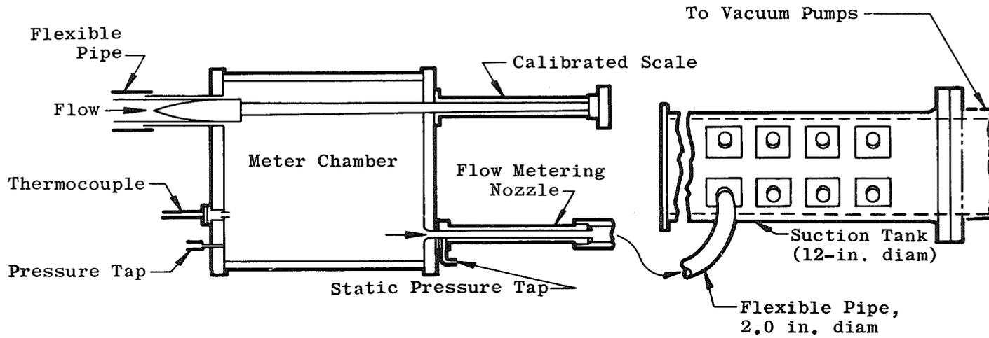
Fig. 6 Schematic Drawing of Suction System
