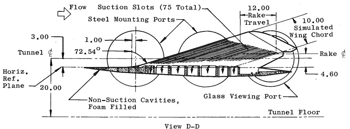
Fig. 3 Model Geometry
