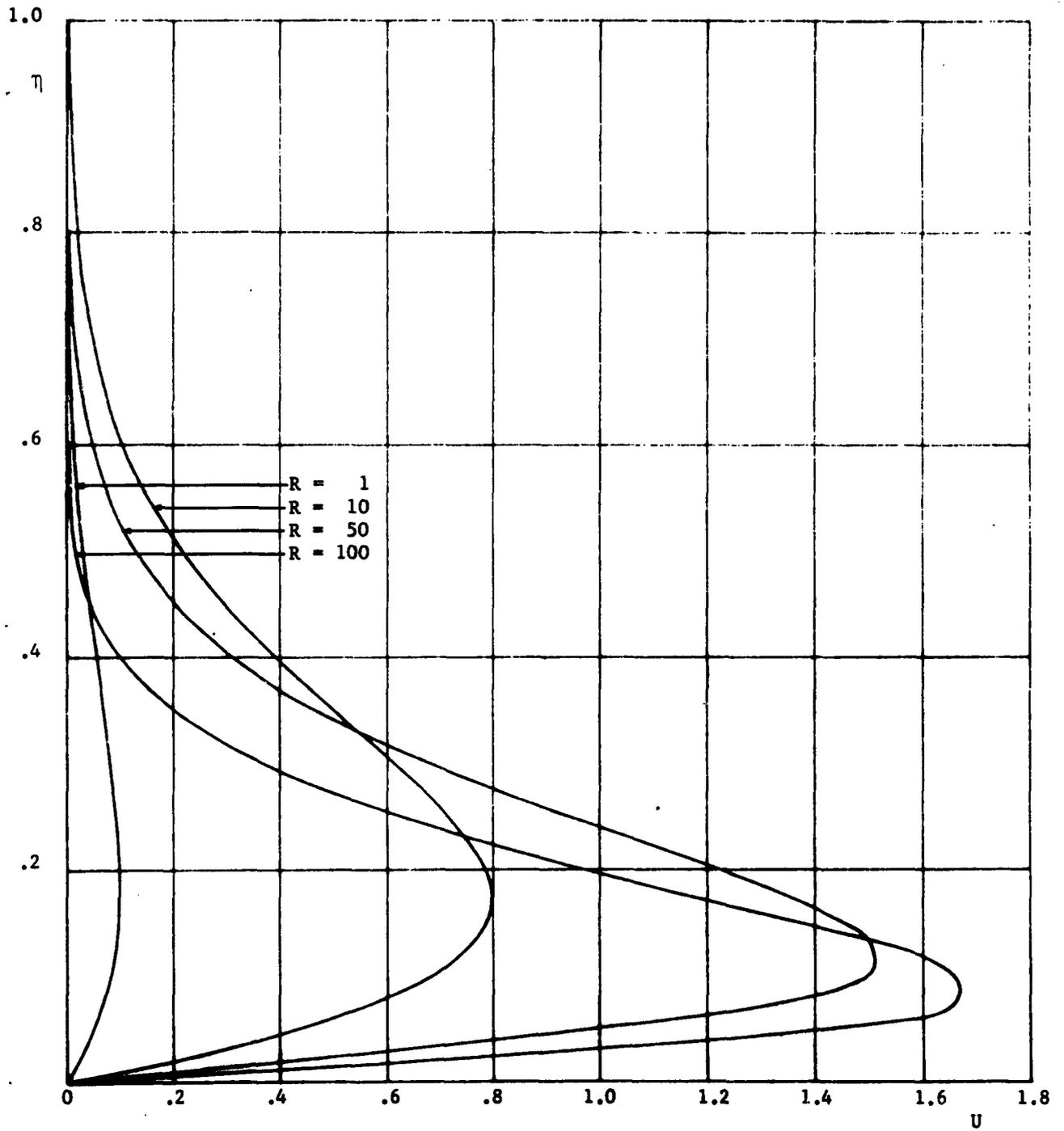
FIGURE 6: The dimensionless velocity component  $U$  vs. the dimensionless variable  $\eta$  for von Karman flows.
