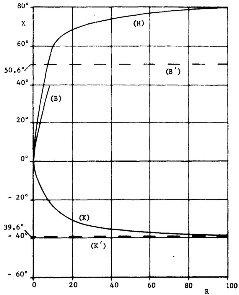
FIGURE 13 : The angle of deviation  $X$  vs. the Reynolds numbers  $R$ .
