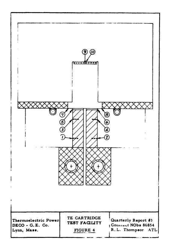
To do this, a copper plate, 4 inches by 4 inches by 1/8 inch with a hole in the center to accommodate the lower end of the case, was prepared. The plate was split from one edge to the hold to permit clamping around the case. A cooling tube of 1/8 inch copper was soldered to one surface of the plate. Thermocouples were spot welded to each lug and the bottom edge of the case adjacent to the lug thermocouples.
