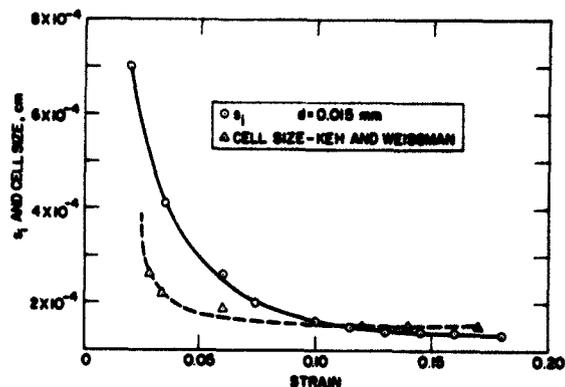
FIG. 6. COMPARISON OF THE AVERAGE DISTANCE MOVED BY DISLOCATIONS DURING EACH 1% INCREMENT OF STRAIN,  $s_i$ , WITH THE DEFORMATION CELL SIZE
