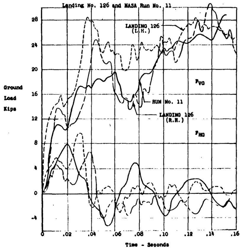
Figure 39. Comparison of Flight Test with NASA Landing-Impact Tests.
