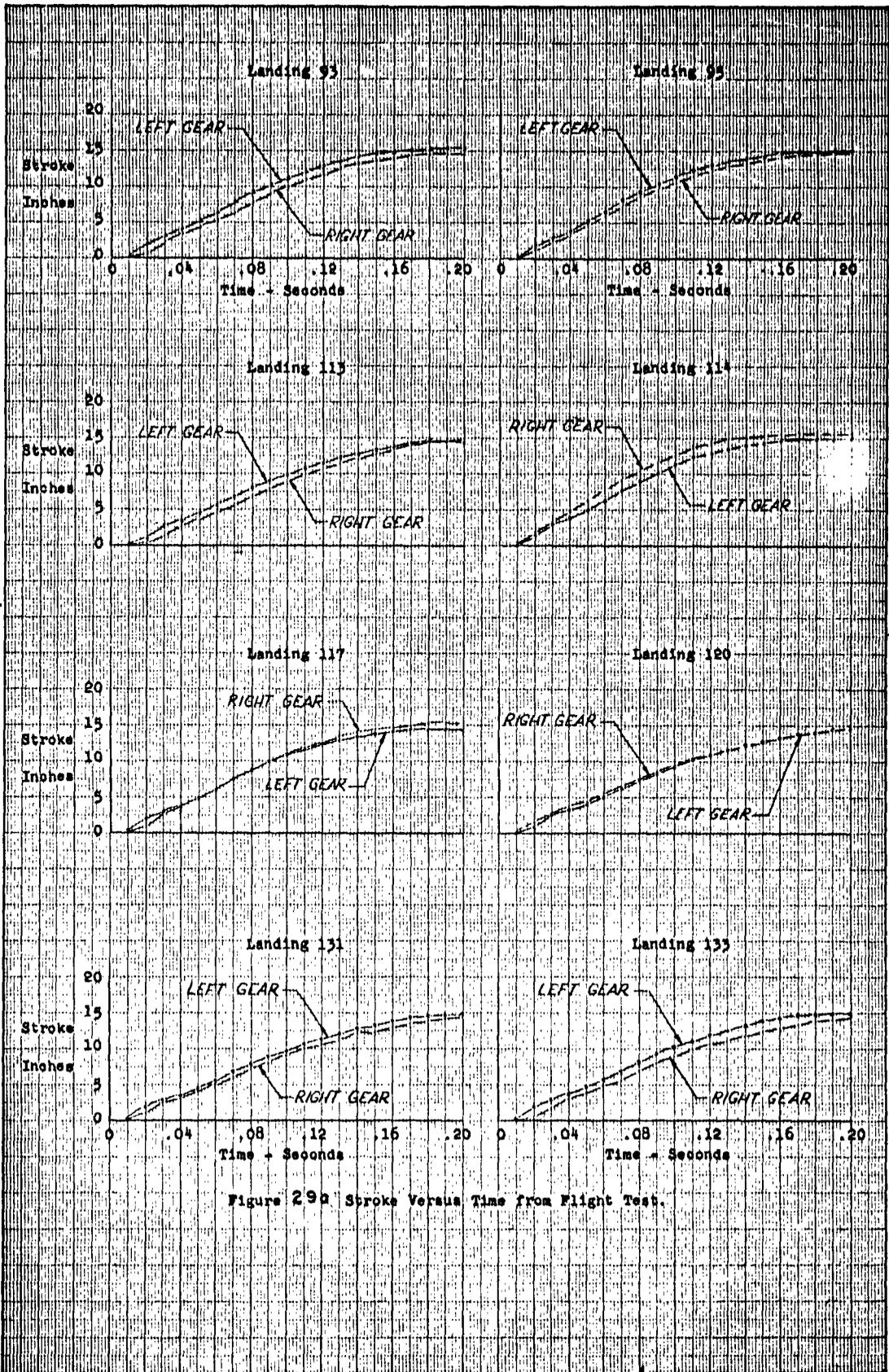
Figure 290 Stroke Versus Time from Flight Test.
