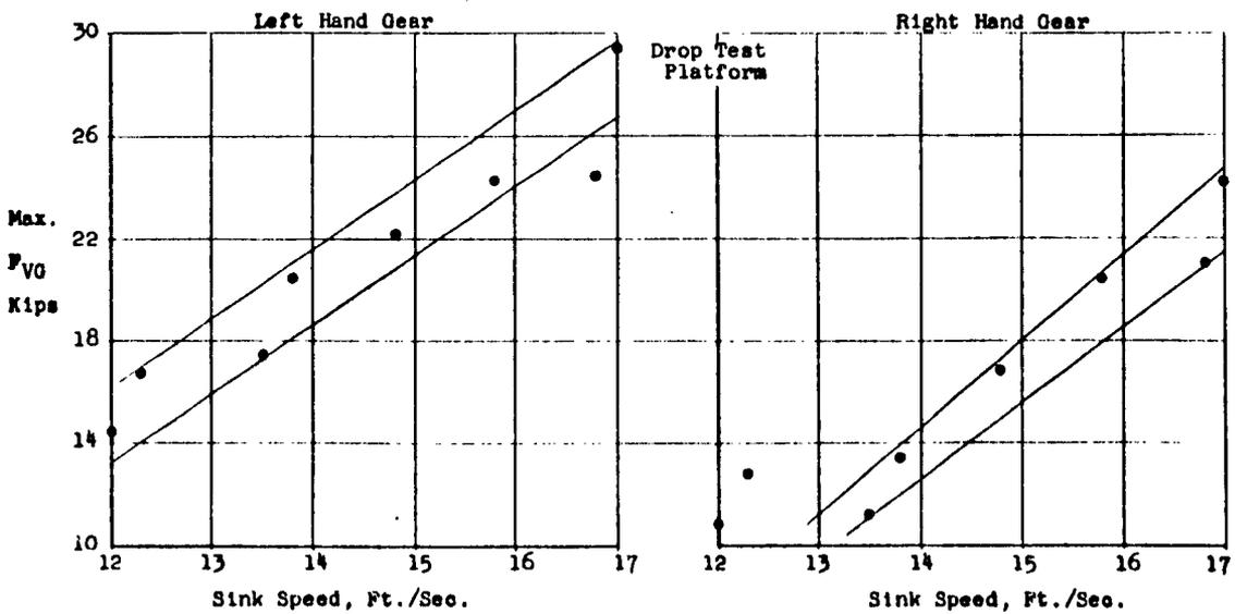
Figure 36. First Peak Maximum Vertical Load Versus Sink Speed.
