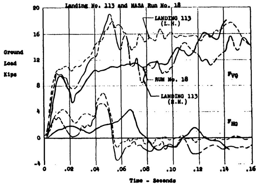
Figure 40. Comparison of Flight Test with NASA Landing-Impact Data.
