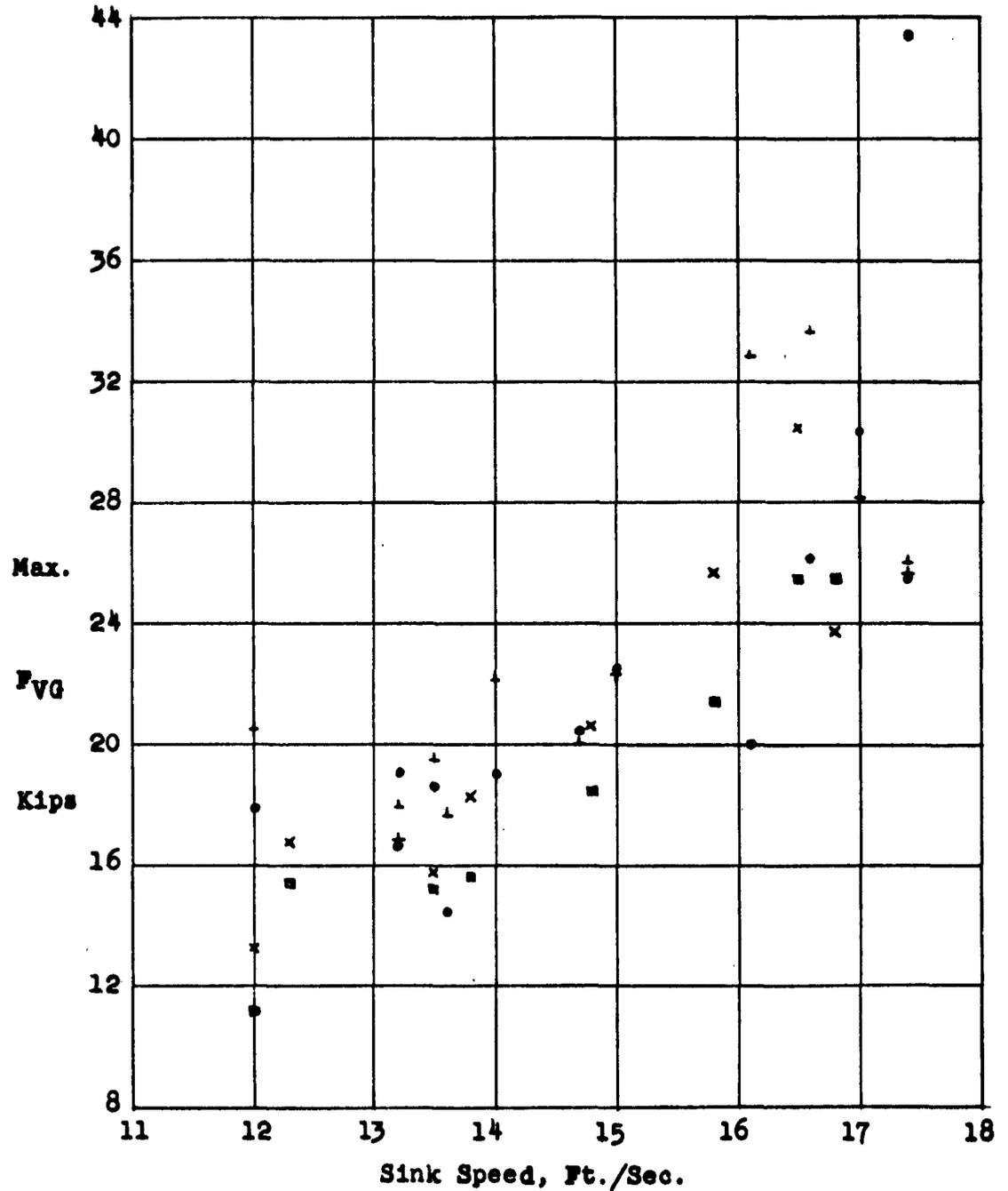
Figure 37a. Maximum Vertical Load Versus Sink Speed from Flight Test and Drop Test.
