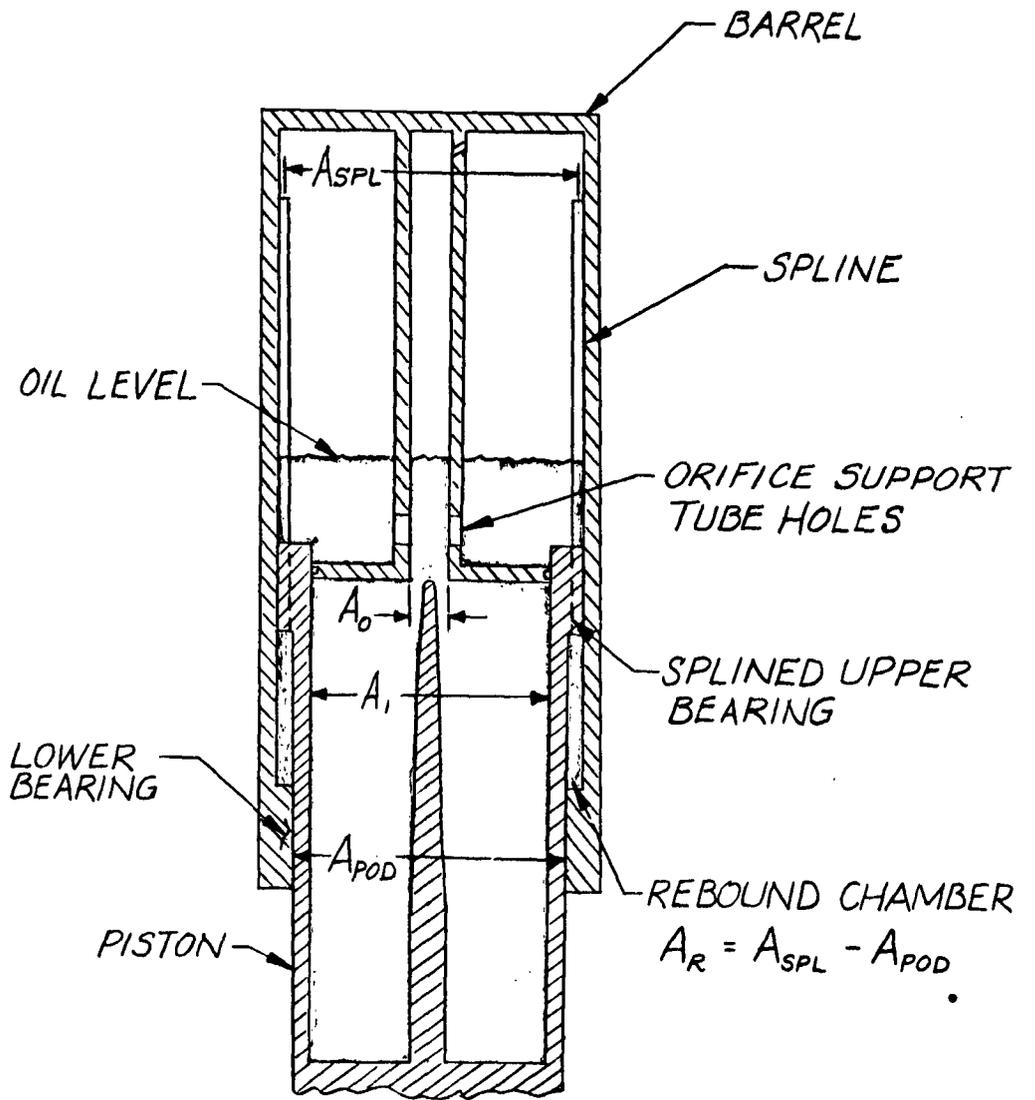
Figure 4. A4D Internal Main Gear Strut Schematic with Strut Extended.
