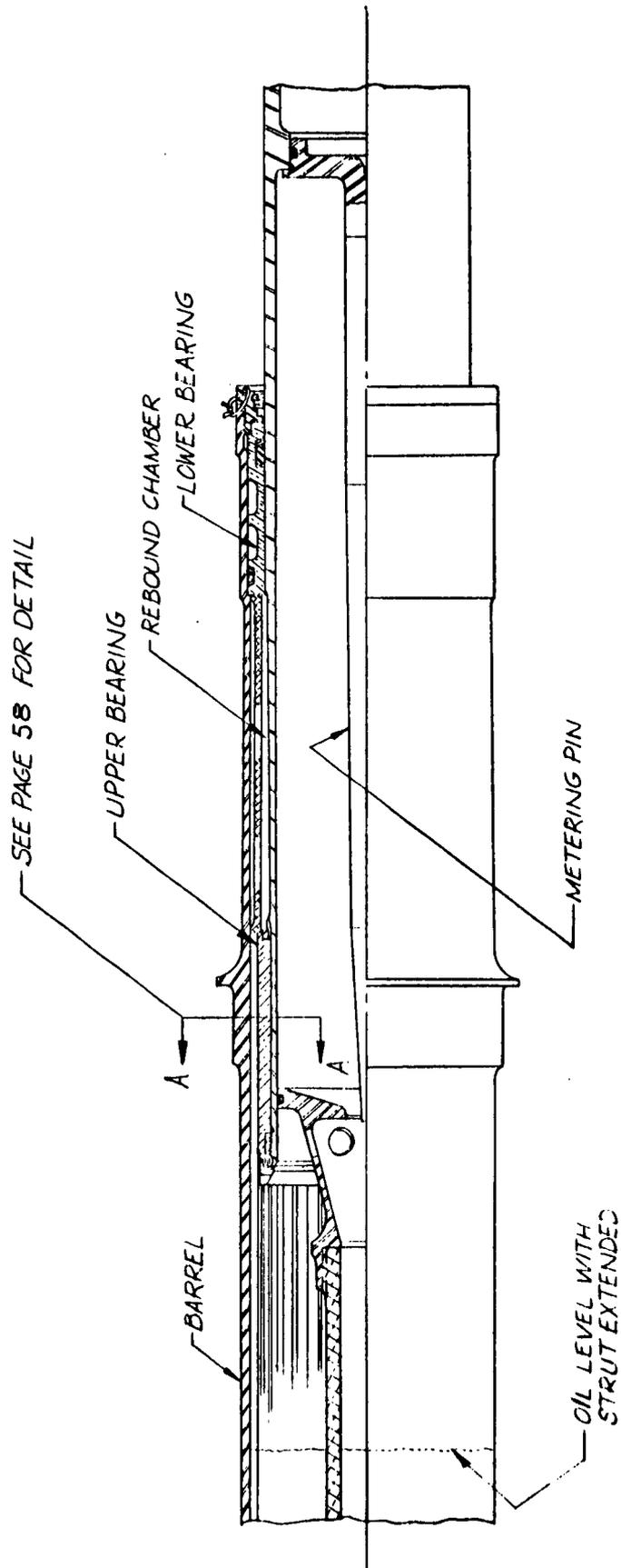
Figure 3. A4D-2 Main Gear Strut in Extended Position.
