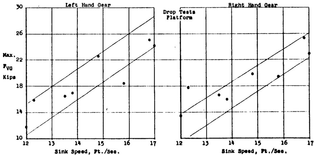
Figure 37. Second Peak Maximum Vertical Load Versus Sink Speed.
