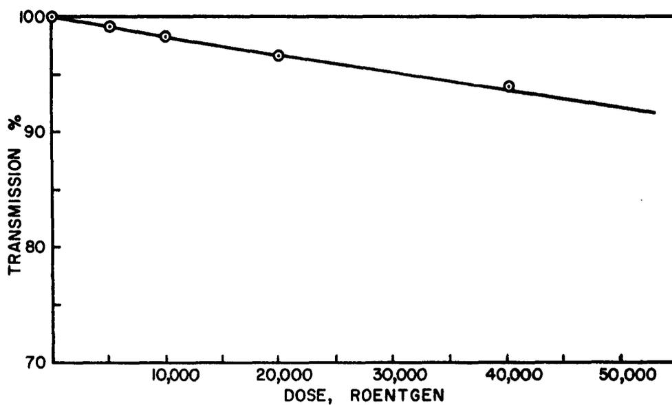
B. % TRANSMISSION OF LIGHT (500 m $\mu$ ) vs DOSE FOR LIME GLASS
