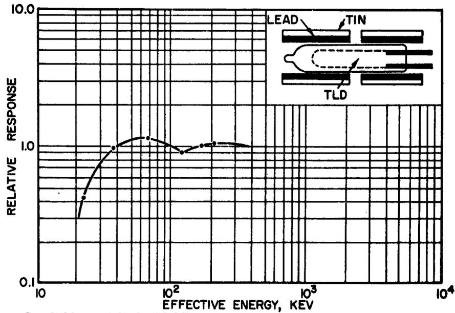
B. 0.86mm TIN OUTSIDE, 0.66mm LEAD INSIDE WITH ANNULAR SLOT TO PROVIDE 10% OPEN AREA.
