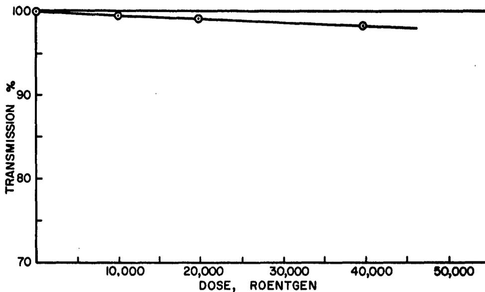
A. % TRANSMISSION OF LIGHT (500 m $\mu$ ) vs DOSE FOR LEAD GLASS
