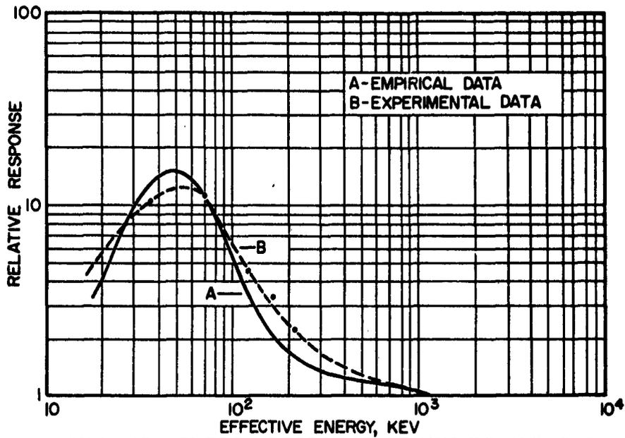
FIGURE 16. ENERGY RESPONSE OF UNSHIELDED  $\text{CaF}_2$  THERMOLUMINESCENT DOSIMETER
