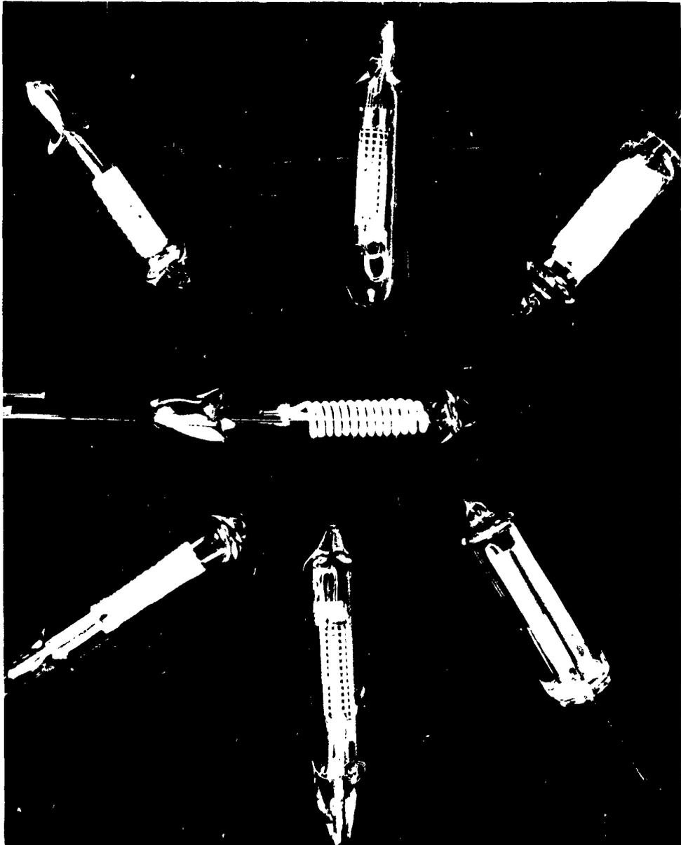
FIGURE 11. SINTERED PHOSPHOR DOSIMETERS
