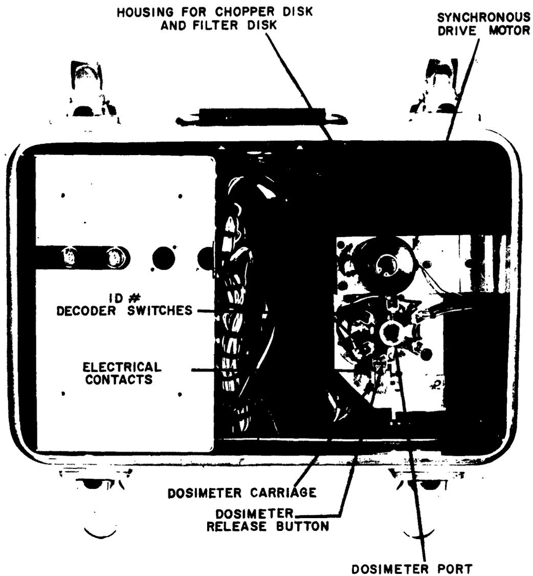
FIGURE 22. COMPLETE READER MOUNTED IN CASE, FRONT
