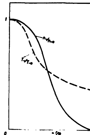
Fig. 4: Schematic sketch of the density and temperature distribution in the thermal glow column.
