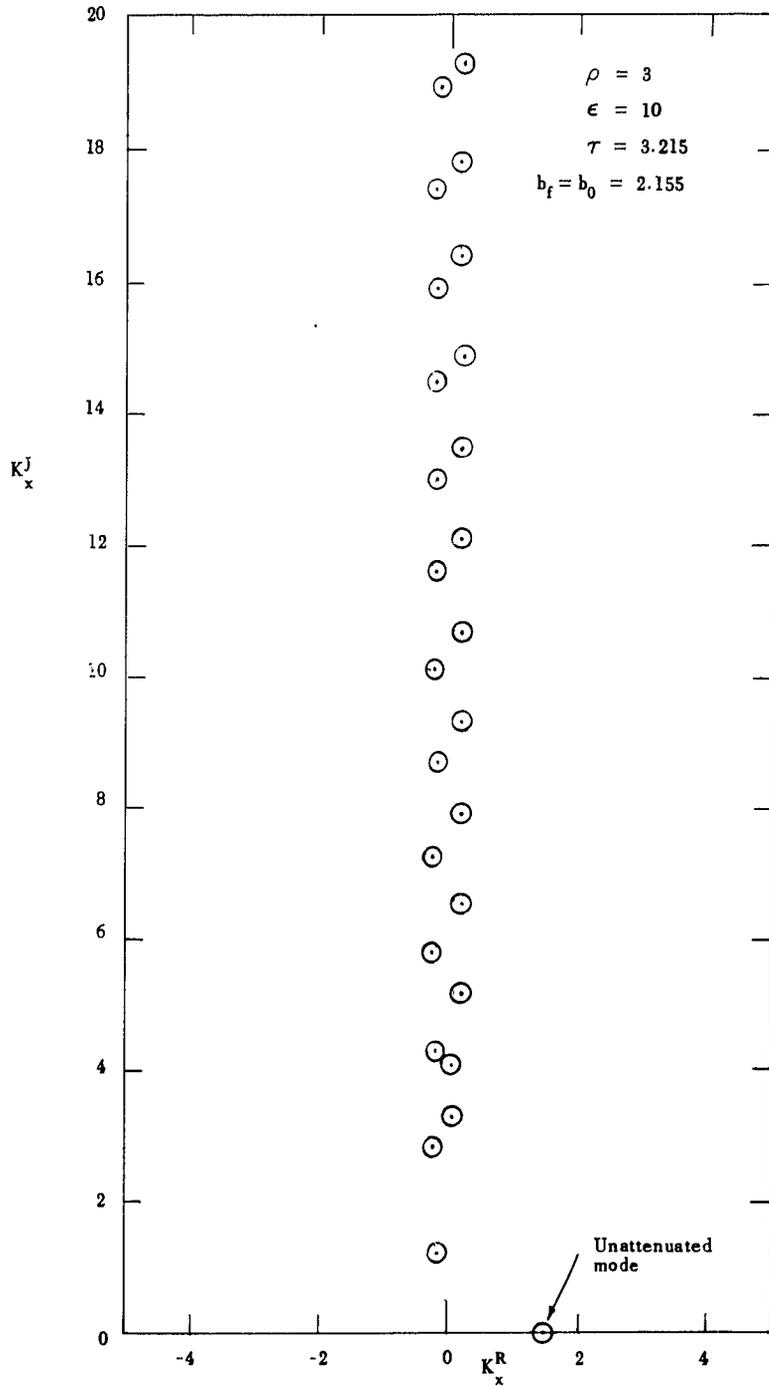
Fig. 2 - Solutions of equation (1) in the complex plane of the propagation constant  $k_x = k_x^R + j k_x^J$ . The numerical results refer to the numerical values of  $\rho$ ,  $\epsilon$ ,  $\tau$ ,  $b_f$  and  $b_0$  indicated in the figure. These values may be taken to correspond to
