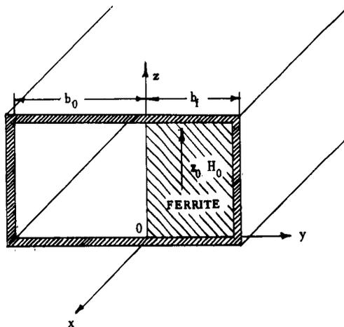
Fig. 1 - The rectangular guide partially filled with ferrite.
