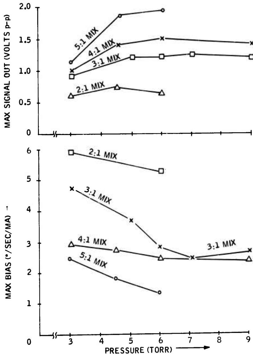
Figure 12. Bias and Signal Sensitivity versus Pressure
