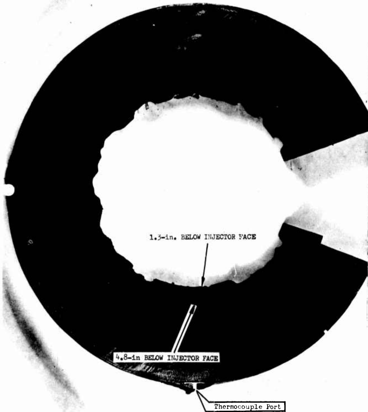
Figure 91. End View of Graphite Phenolic Chamber Section Tested with Injector S/N 2, Mod 3 (u)
