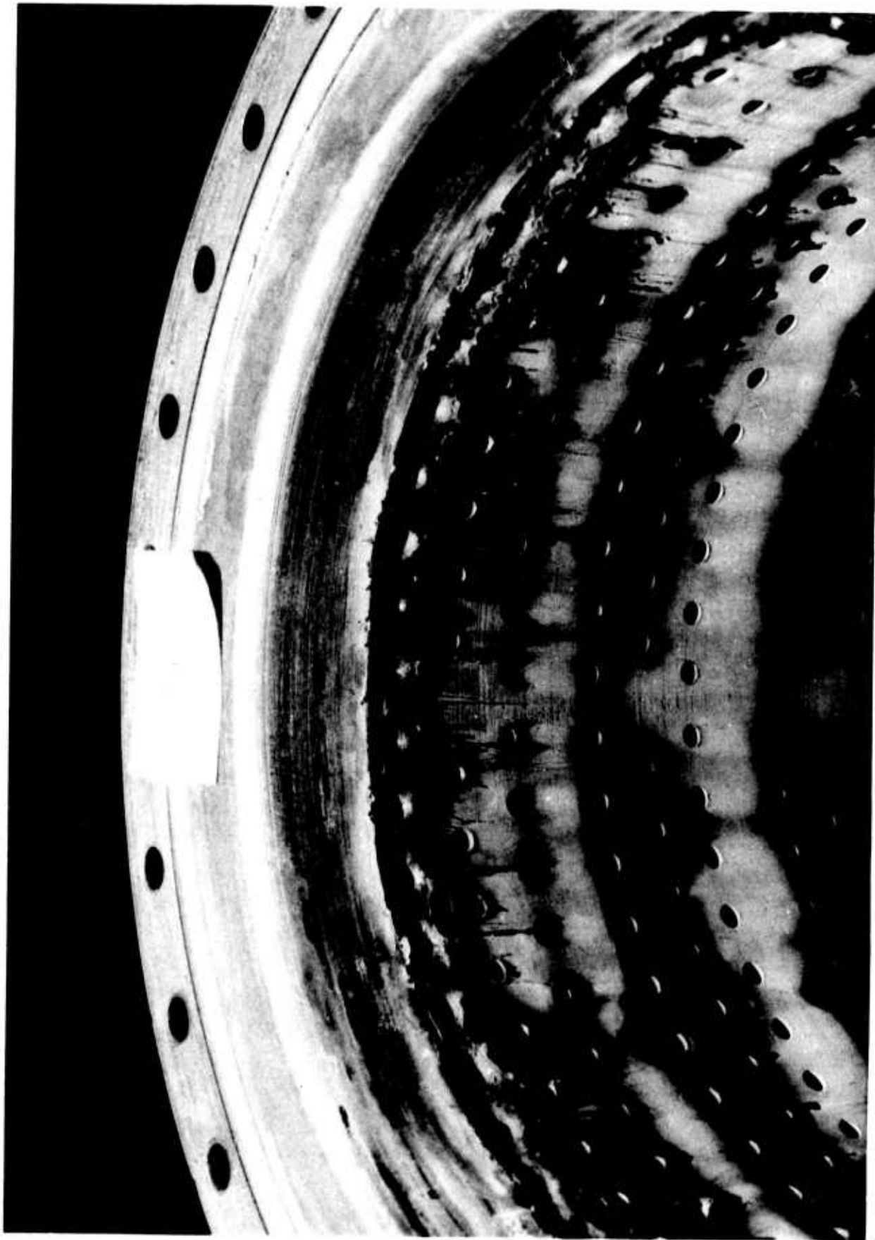
Figure 54. Post-Test (No. 025) View of Steel Chamber with Acoustic Resonator (u)
