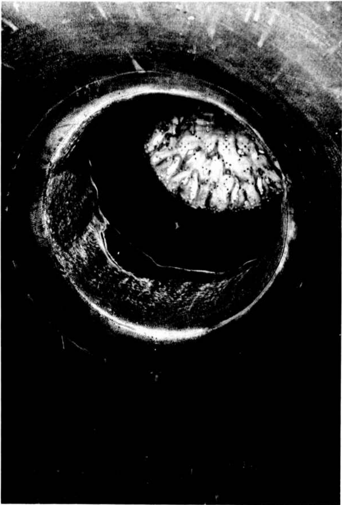
Figure 44. Delaminated Section of Throat Insert, Ablative Chamber S/N 002 (u)
