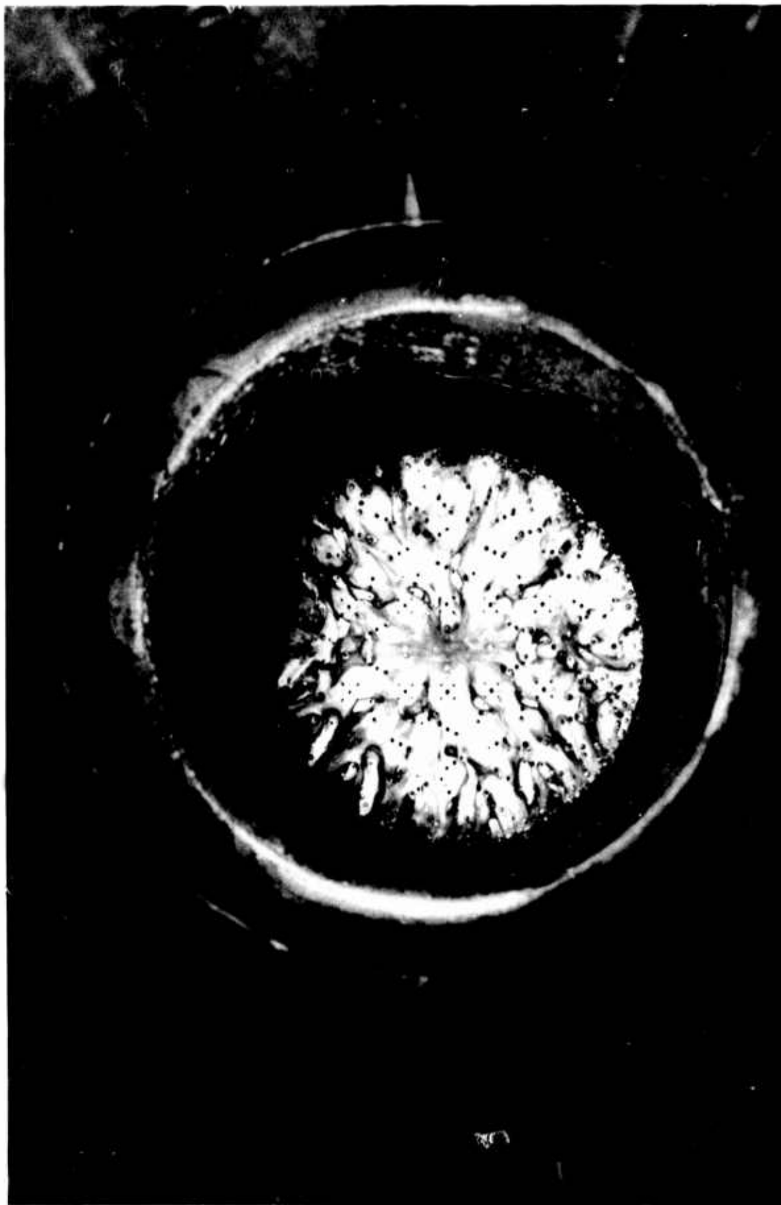
Figure 90. Graphite Phenolic Chamber after 202 sec of Testing with Injector S/N 2, Mod 3 (u)
