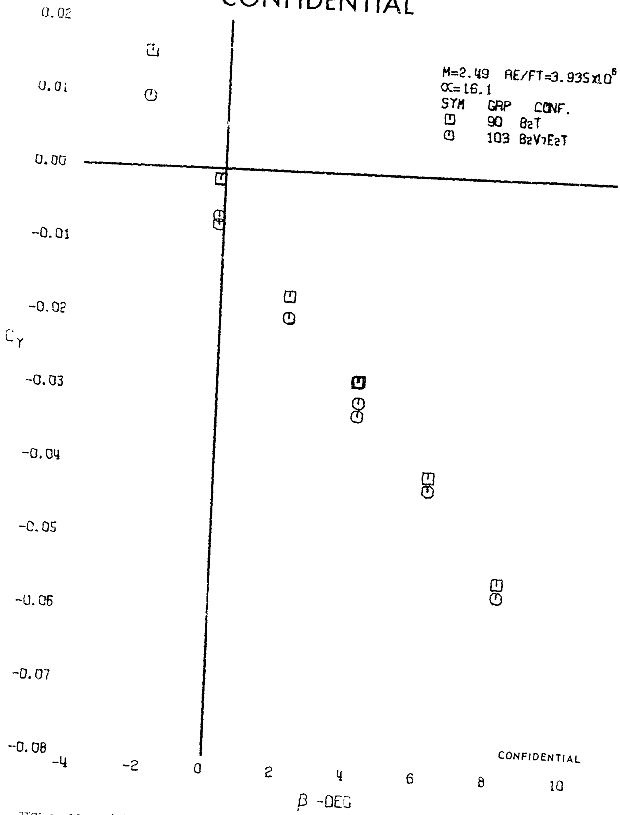
FIGURE 112 (U) CONFIGURATION BUILDUP - SIDE FORCE COEFFICIENT VARIATION WITH ANGLE OF YAW (M=2.49)
