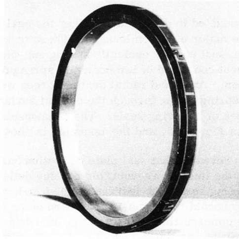
Figure 90. Regenerator I. D. Ring Seal, Segmented Carbon, With Axial and Radial Spring Loading.
