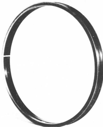
Figure 116. Regenerator I.D. Ring Seal, All-Metal Simplex Seal.
