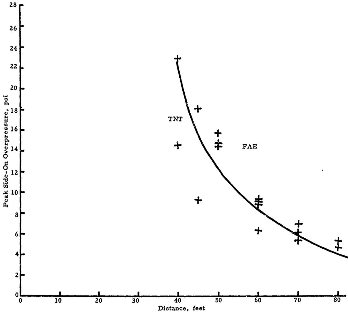
FIGURE 22. PEAK SIDE-ON OVERPRESSURE VS. DISTANCE FOR FAE PROPELLANT AND TNT
