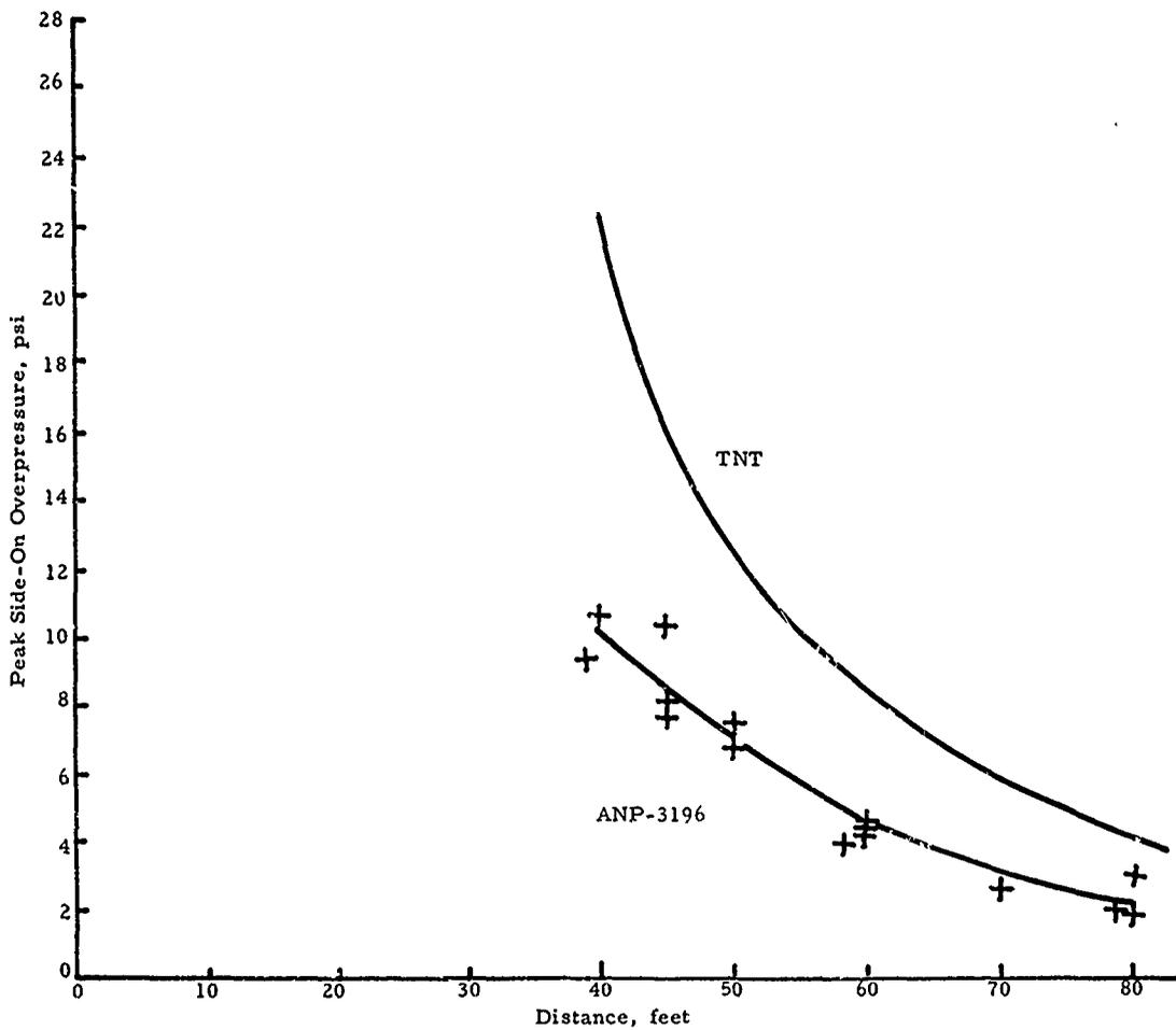
FIGURE 36. PEAK SIDE-ON OVERPRESSURE VS. DISTANCE FOR ANP-3196 PROPELLANT AND TNT
