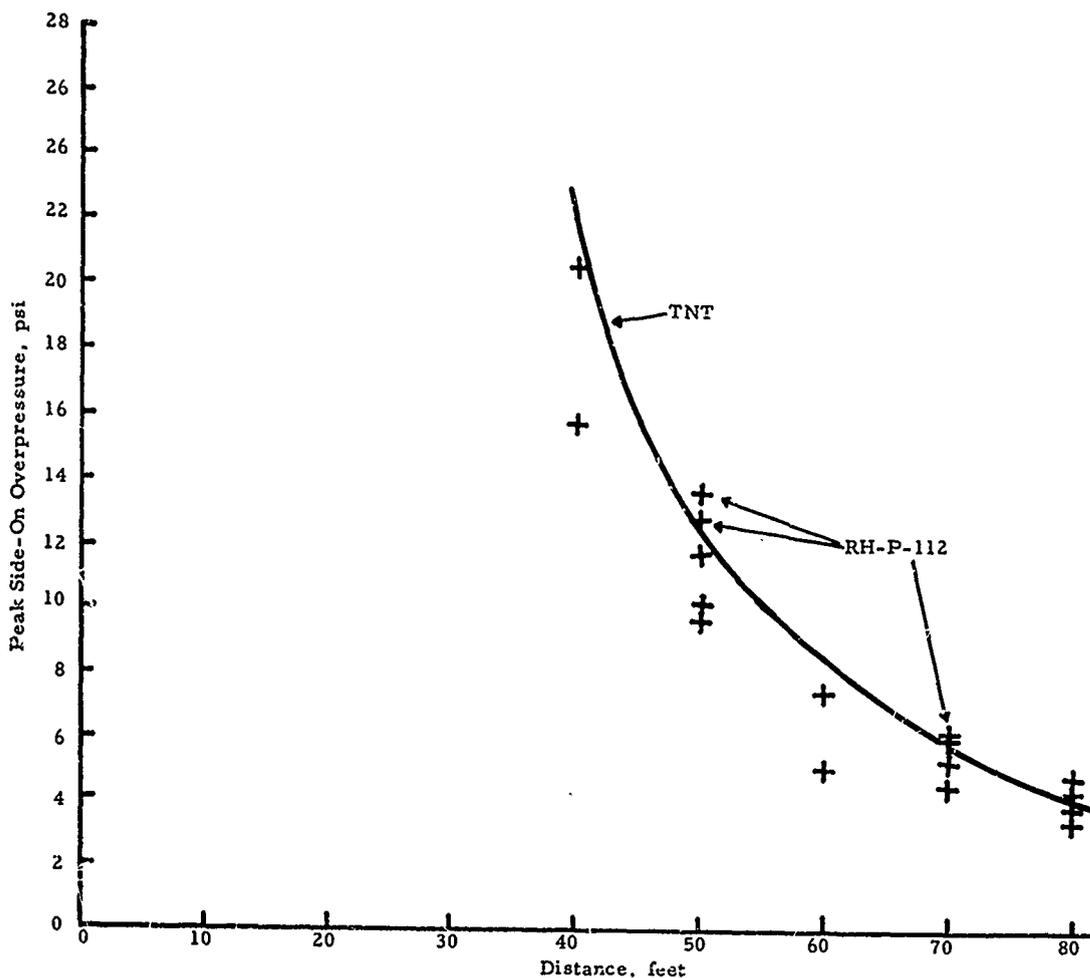
FIGURE 46. PEAK SIDE-ON OVERPRESSURE VS. DISTANCE FOR RH-P-112 PROPELLANT AND TNT
