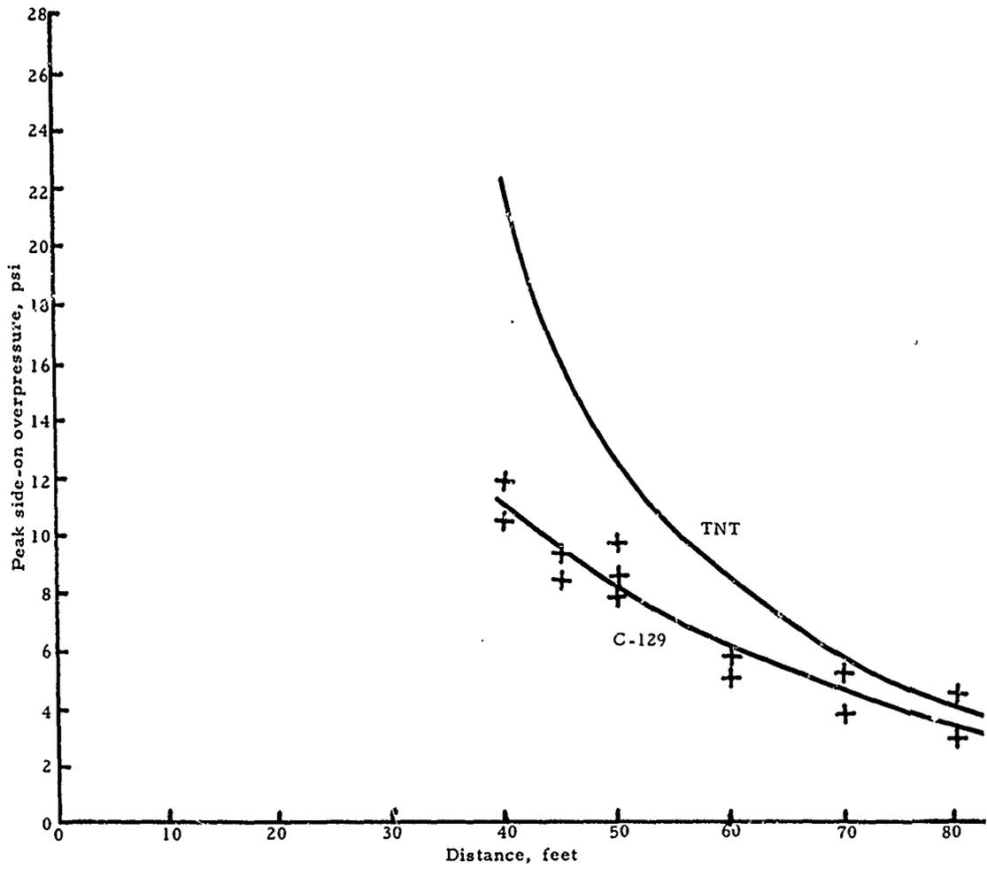
FIGURE 38. PEAK SIDE-ON OVERPRESSURE VS. DISTANCE FOR C-129 PROPELLANT AND TNT
