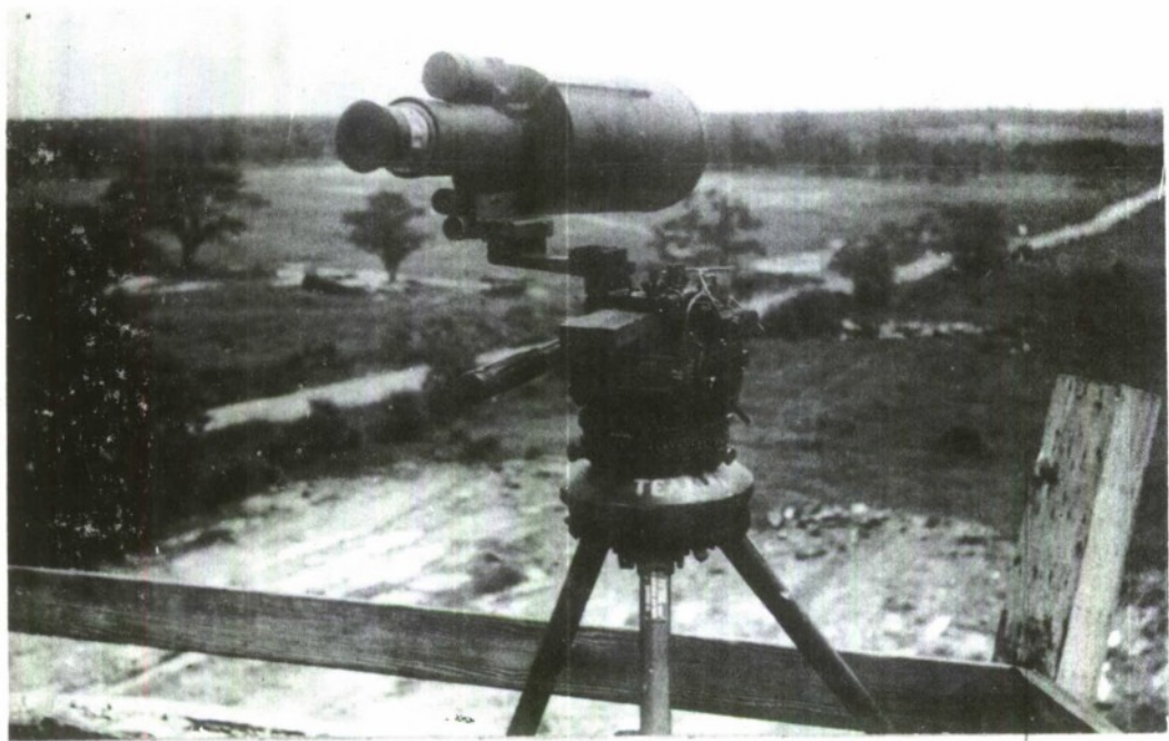
(C) FIGURE 3. Crew-Served Night Vision Sight used in conjunction with the AN/PPS-4 radar set.
