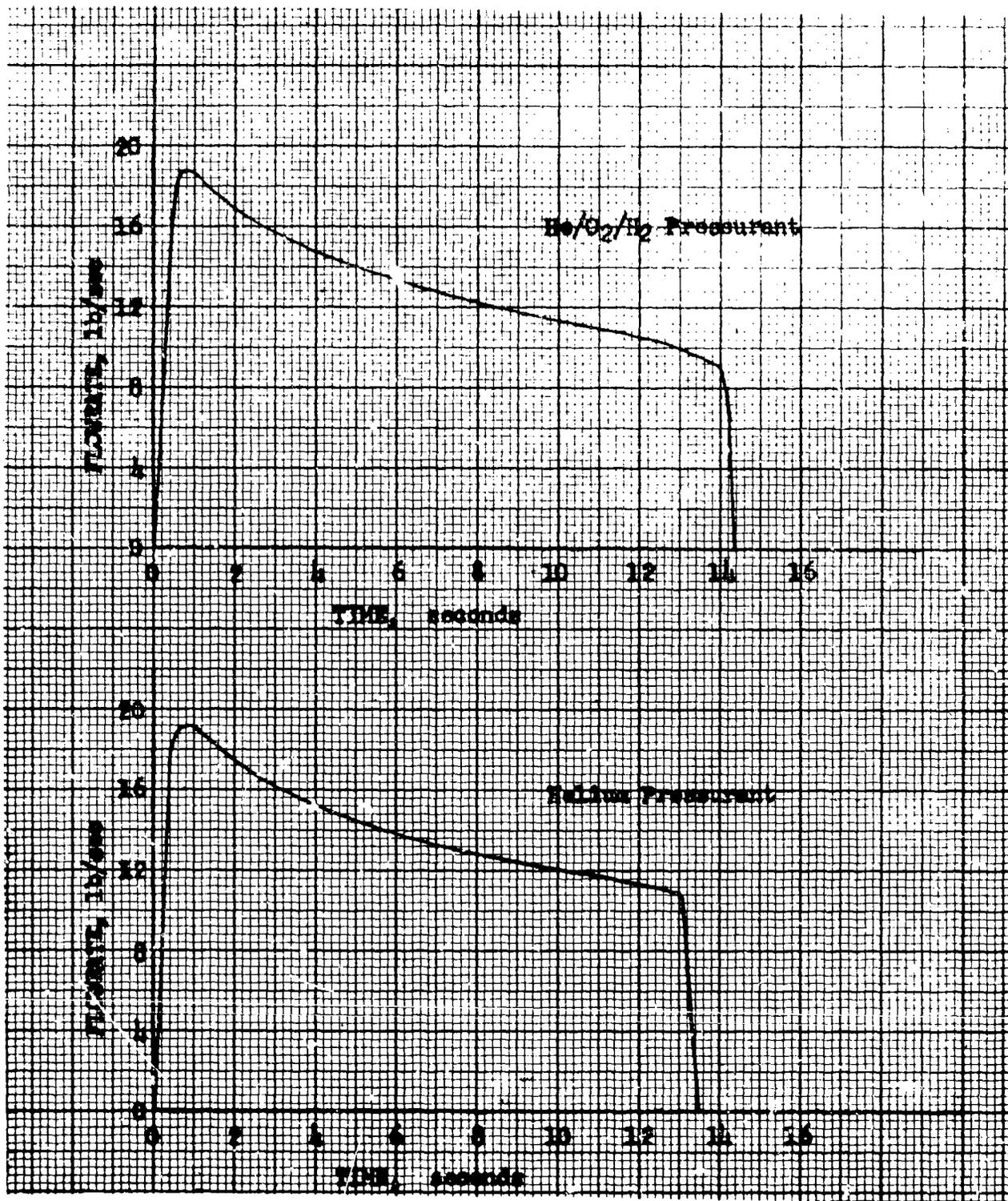
Figure 50. Liquid Nitrogen Flowrate as a Function of Time for Expulsion Demonstration Tests
