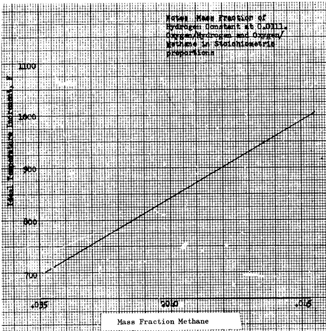
Figure B-2 Ideal Temperature Increment for
