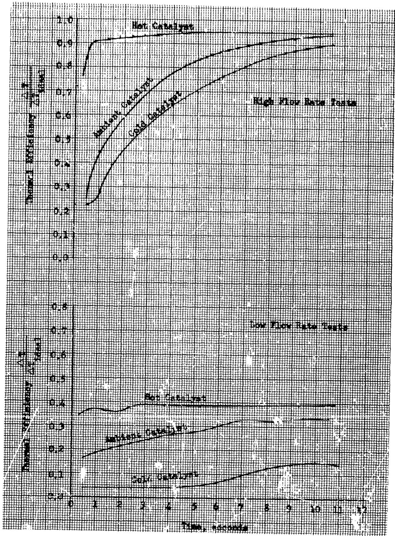
Figure 41. Delivered Thermal Efficiency for He/O<sub>2</sub>/H<sub>2</sub> at -155 F and High Injection Pressure (Tests 71<sup>A-F</sup>)
