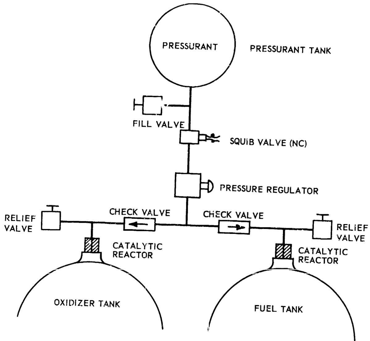
Figure 69. Schematic Representation of a Typical Catalytically Ignited Pressurization System
