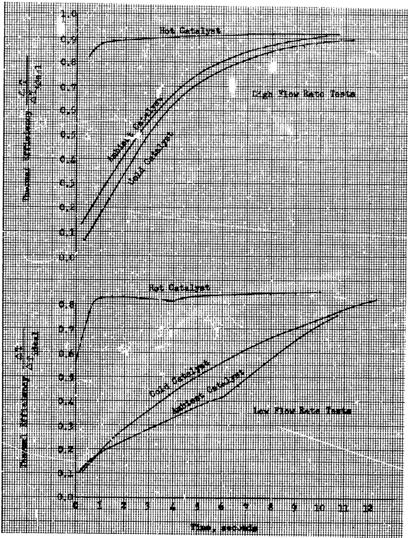
Figure 44. Delivered Thermal Efficiency for He/O<sub>2</sub>/H<sub>2</sub>/CH<sub>4</sub> at -115 F and Low Injection Pressure (Tests 74 A-F)
