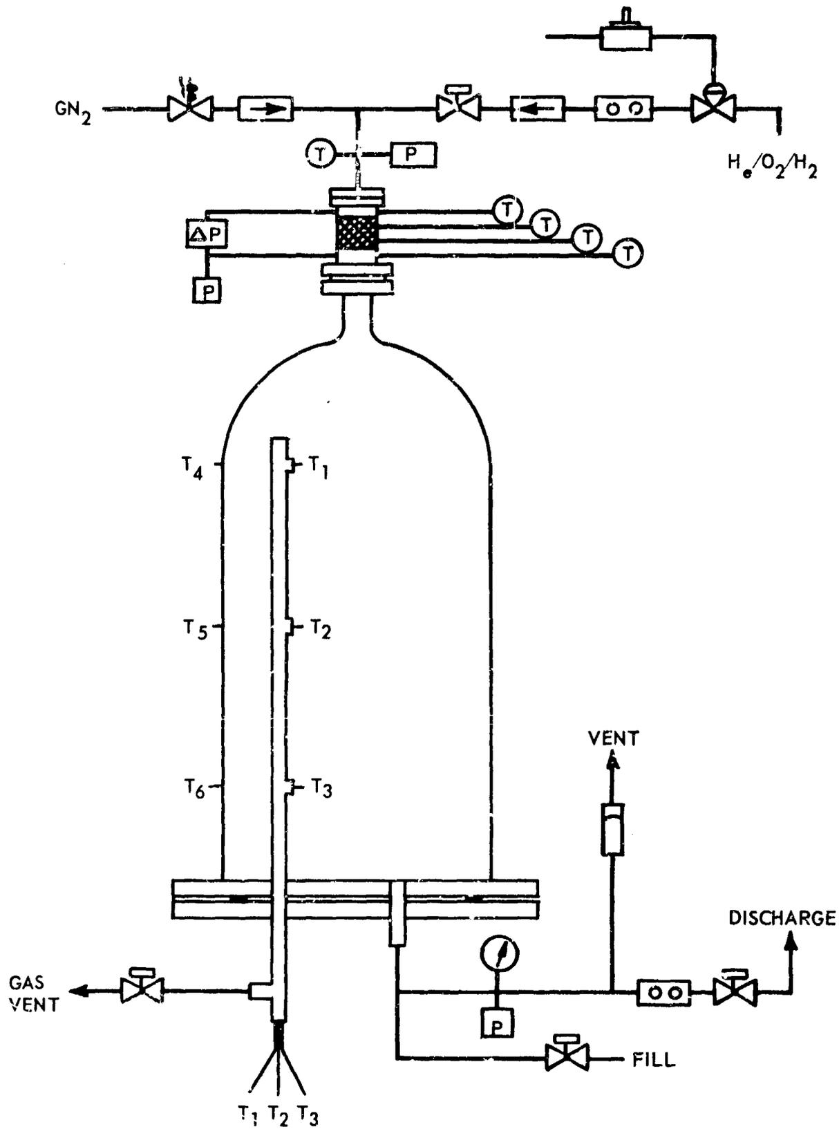
Figure 47. Expulsion System Schematic
