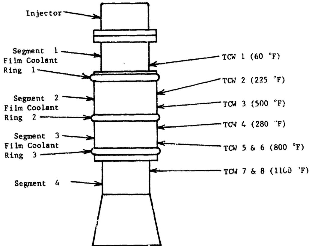
Figure 13. Thrust Chamber Temperature Profile
