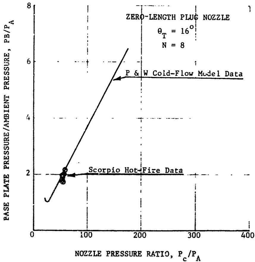
Figure 34. Hot-Fire and Cold-Flow Baseplate Pressure Correlation
