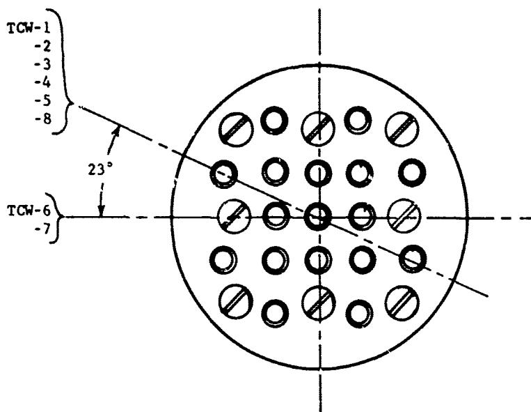
Figure 21. Thrust Chamber Wall Temperature Probe Locations
