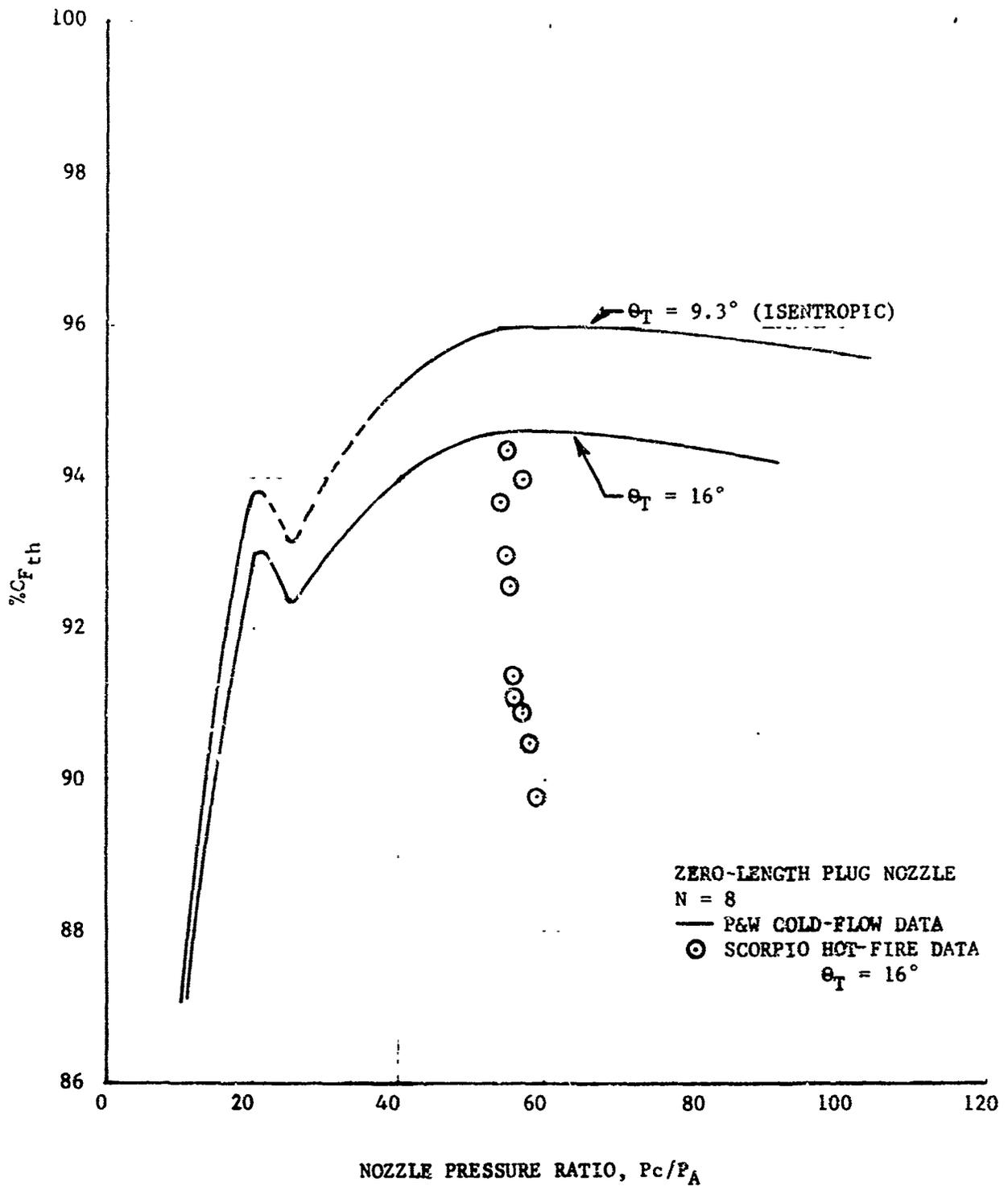
Figure 35. Tilt-Angle Effect on Nozzle Performance, Zero-Length Plug
