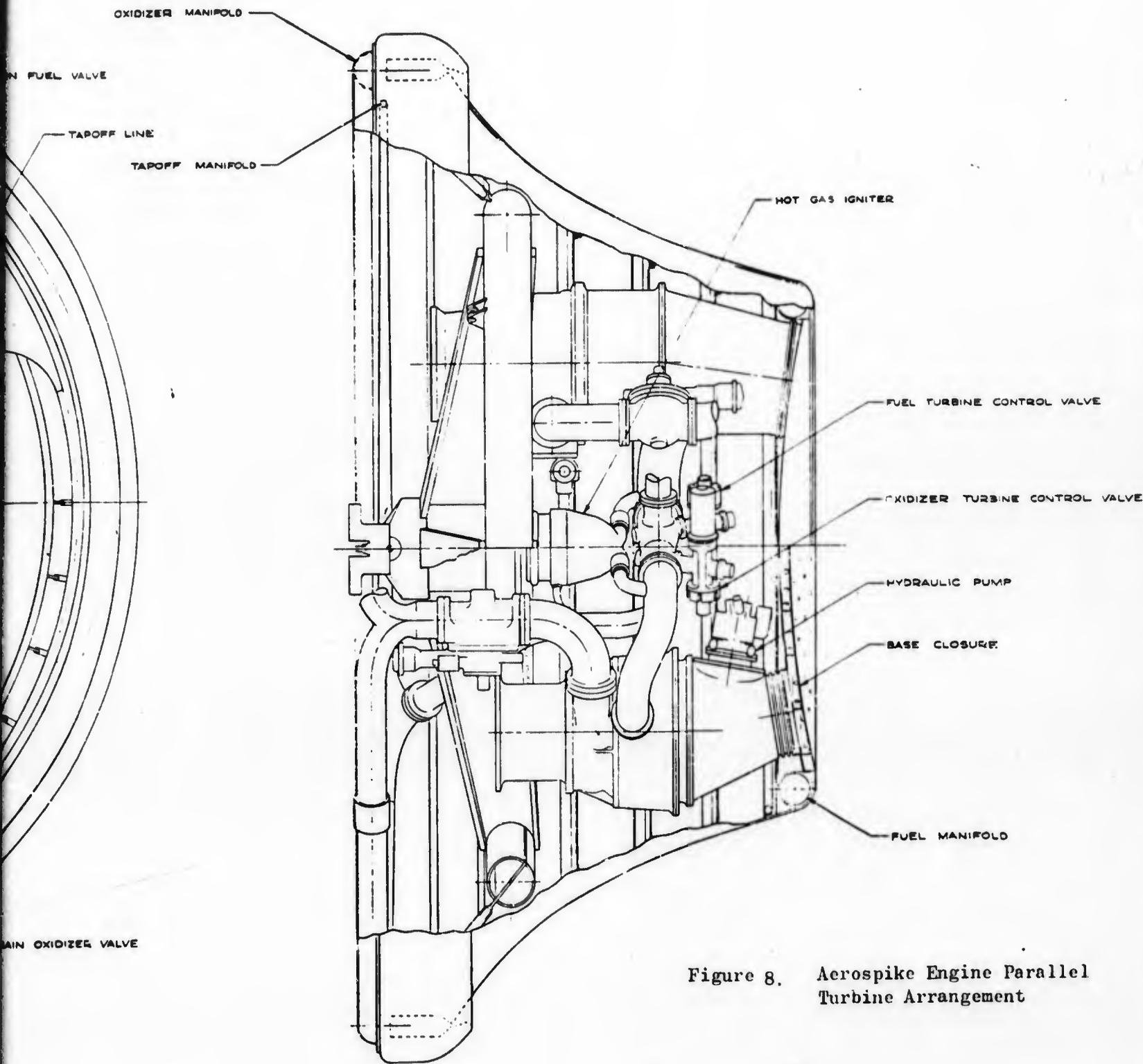
Figure 8. Aerospike Engine Parallel Turbine Arrangement
