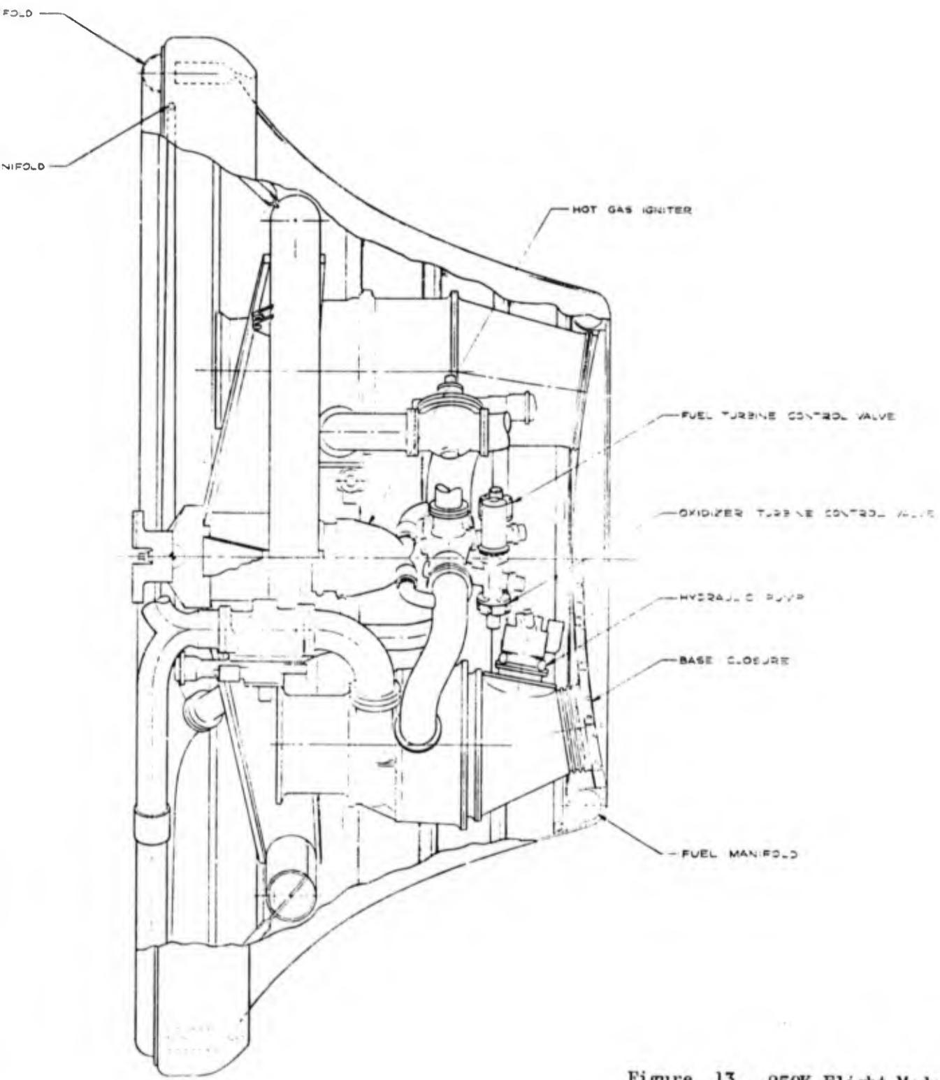
Figure 13. 250K Flight Module
