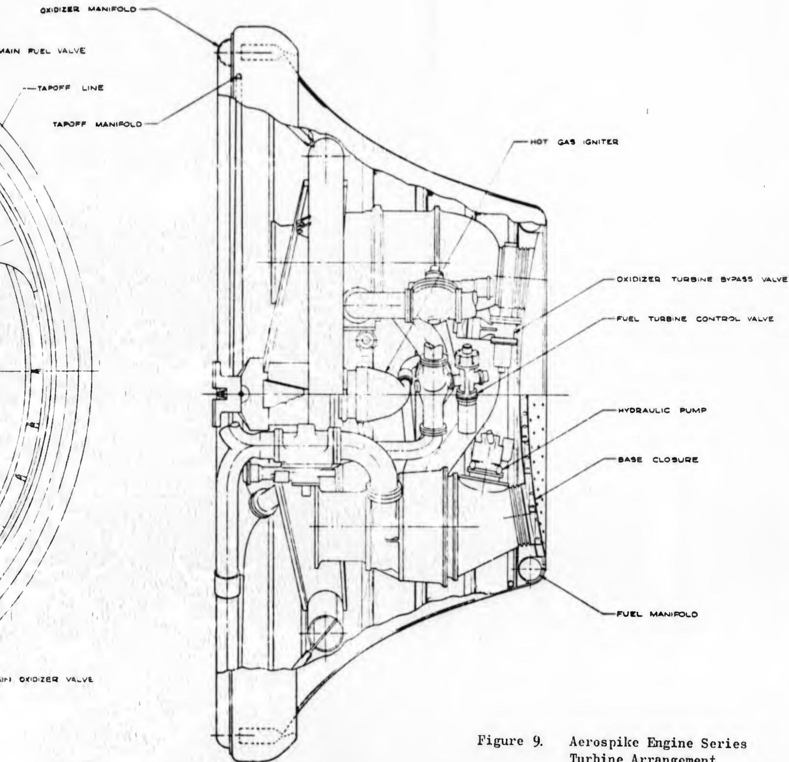
Figure 9. Aerospike Engine Series Turbine Arrangement
