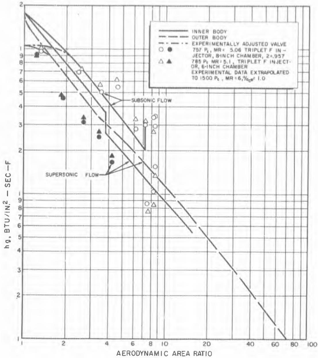
Figure 36. Theoretical and Experimental Heat Transfer Coefficients, 250K Experimental Thrust Chamber Breadboard Engine,  $O_2/H_2$ , MR = 6.0,  $P_c = 1500$  psia, Vacuum Operation
