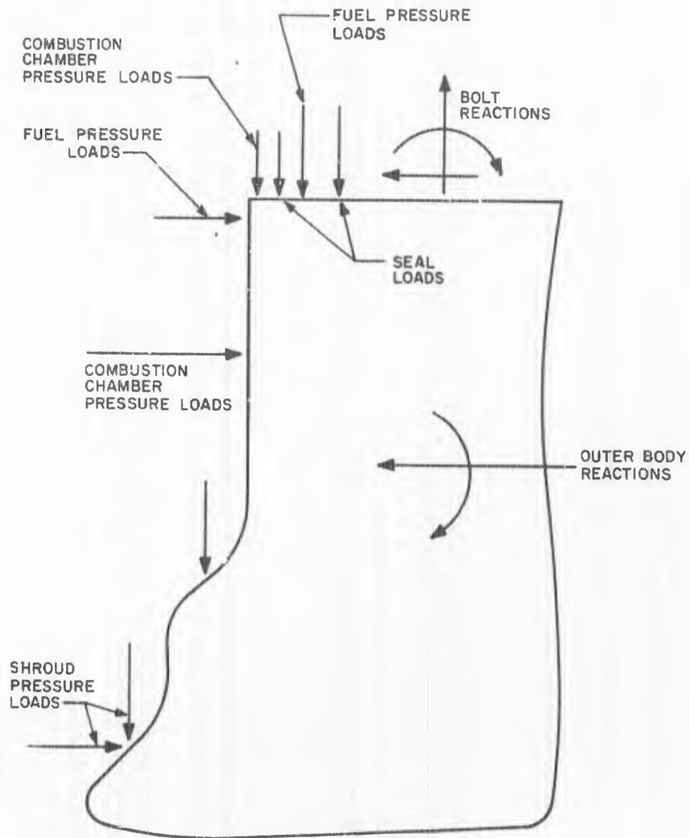
Figure 26. Forces Acting on Outer Body
