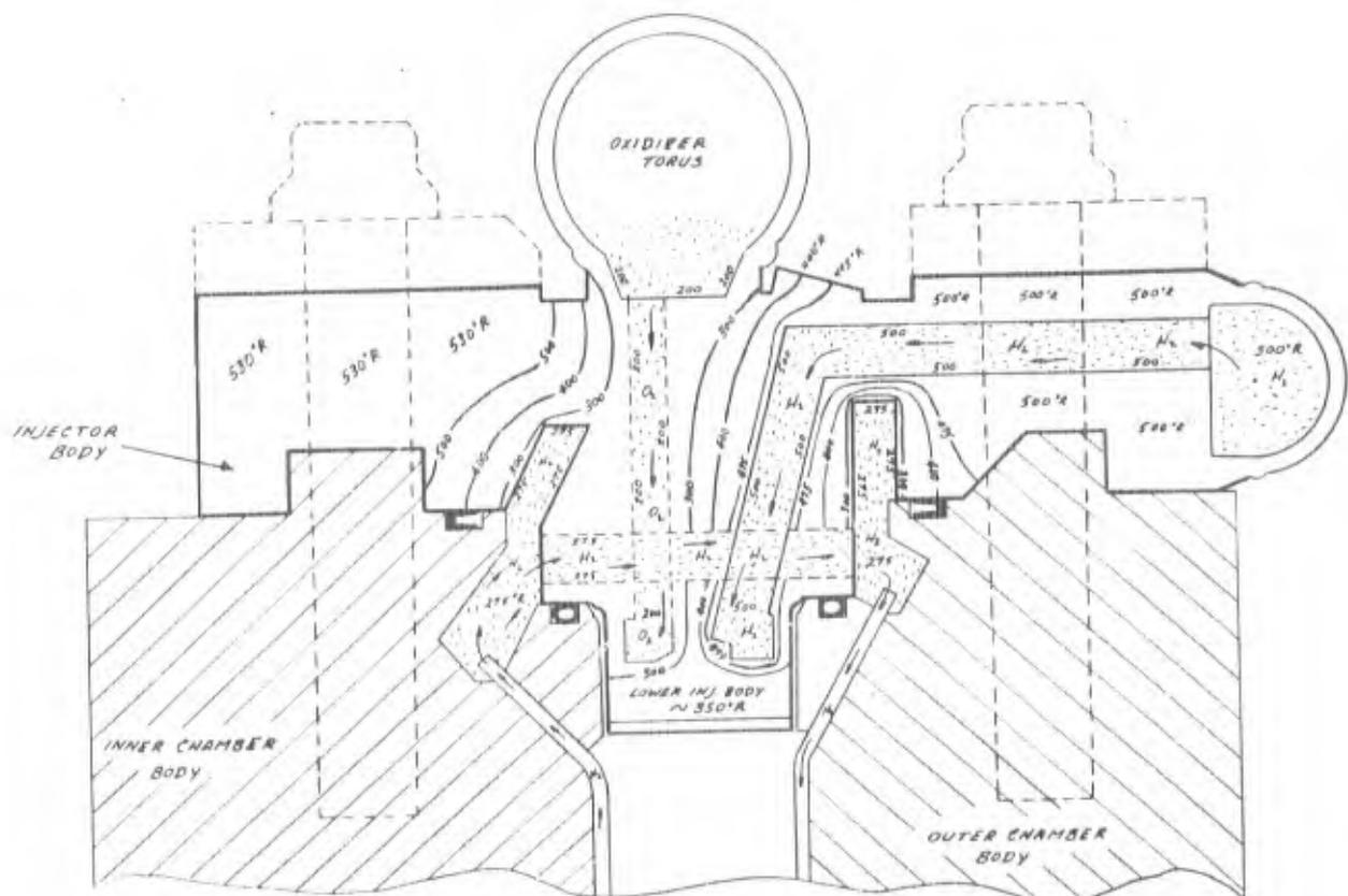
Figure 45. Approximate Injector Body Isotherm Distribution After a 10-Second Mainstage Test
