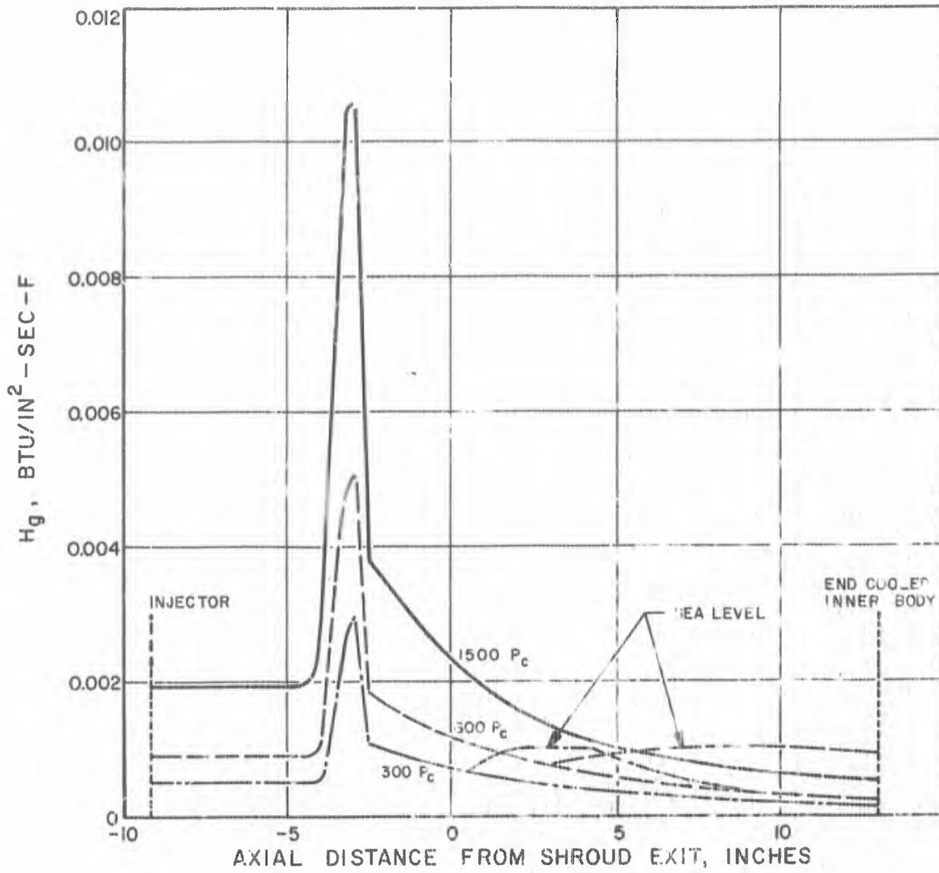
Figure 35. Theoretical Nozzle Gas-Side Heat Transfer Profiles at Vacuum and Sea Level Conditions (250K Experimental Chamber, MR = 6.0)
