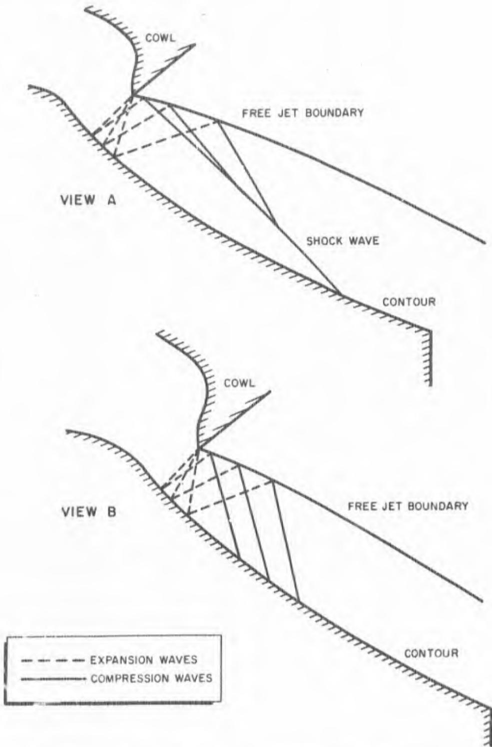
Figure 35. Expansion and Compression Waves in Aerodynamic Spike Nozzle Flow Field Analysis
