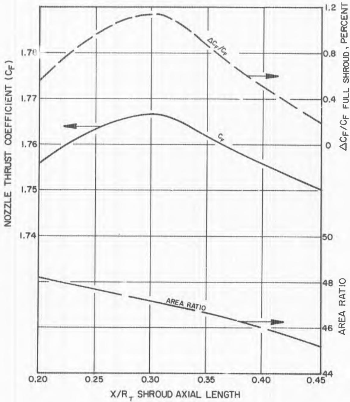
Figure 31. Performance vs Shroud Length
