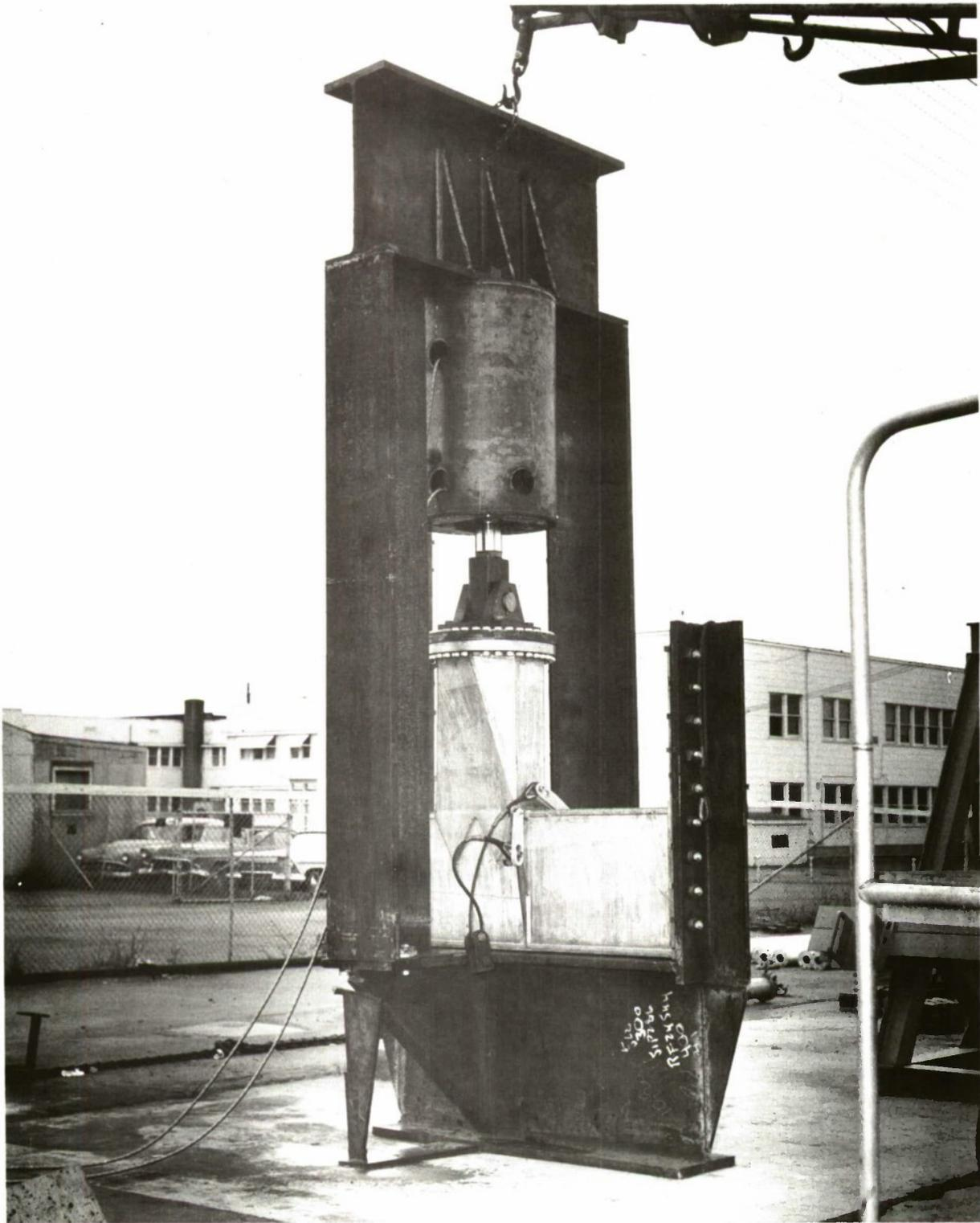
FIG.II TESTING BEAM VIA BONNET LOADING OF 364,000 LBS.
