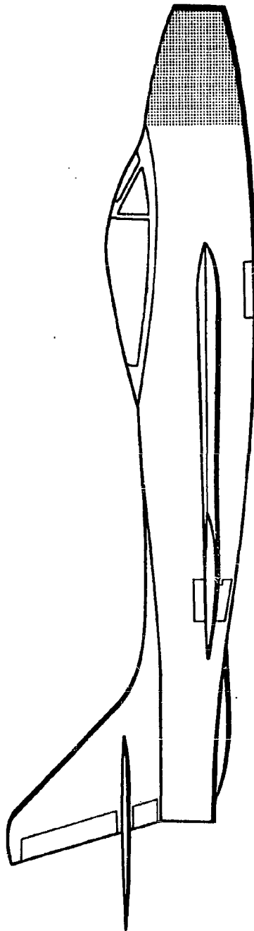
FIGURE 29. F-84F Nose Damage
